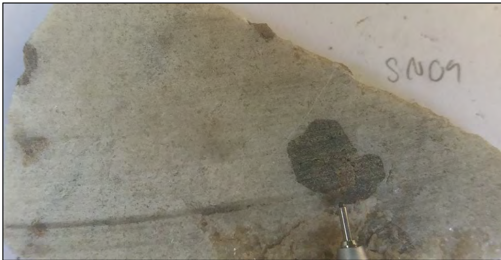
Figure 3.25 Hand specimen [upper photo] and slab [lower photo] garnet marble is showing large dark green garnet phenoblasts and coarse-grained of calcite. (sample number: SN09)
