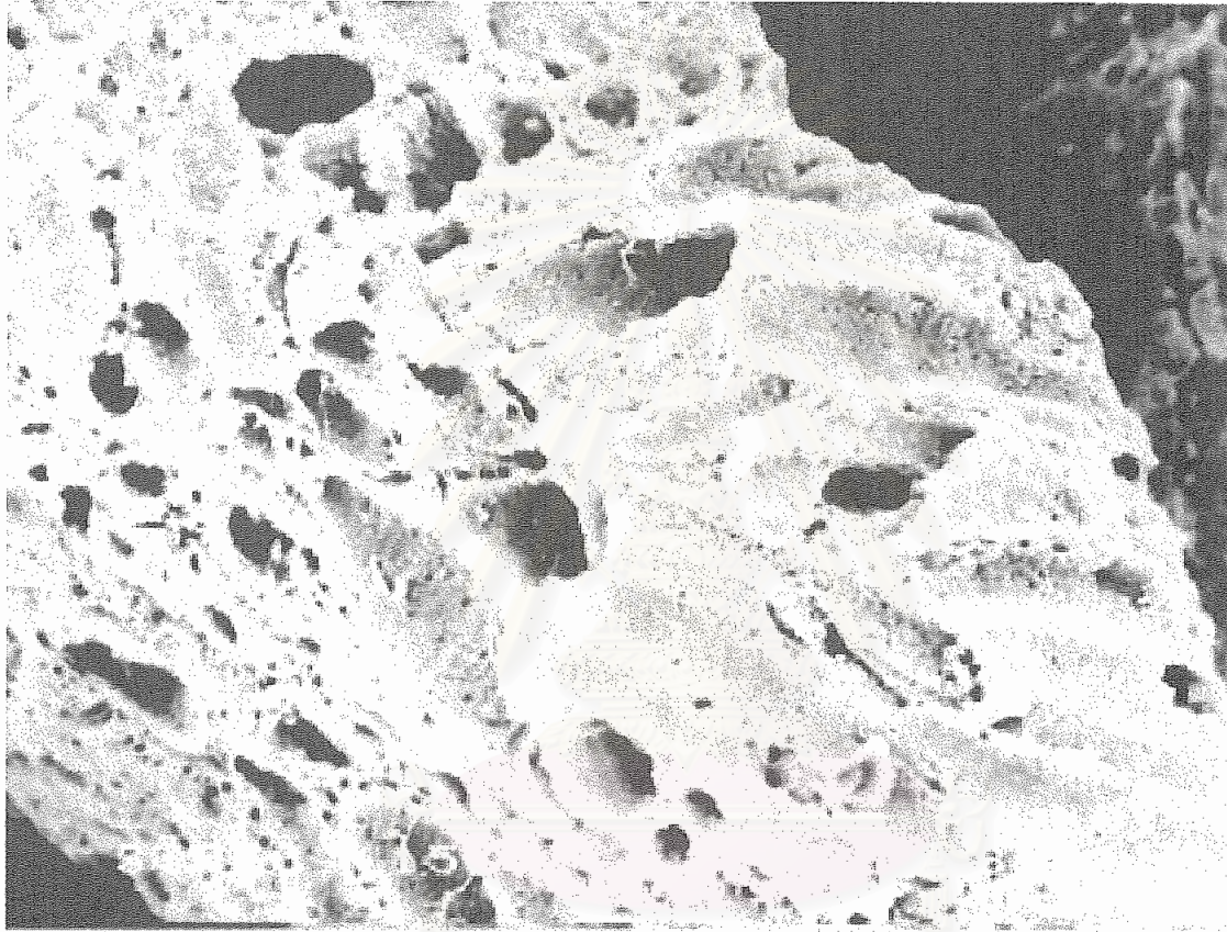
Figure 5.8 The surface specific area of catalyst before using in reaction
