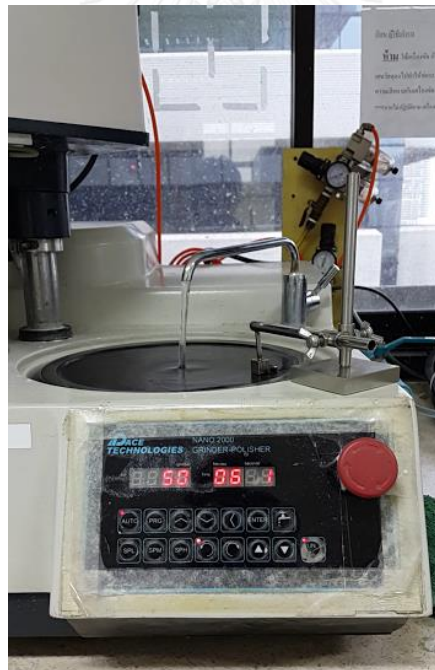
Figure 9: Polishing ceramic block with a 240, 400, 600-grit silicon carbide paper
