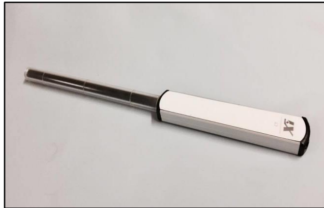
Figure 3.7 Pencil-type ionization Unfors Xi CT Detector.
