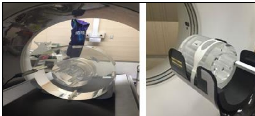
Figure B 17 CTDI 100 measurement in body and head PMMA phantoms using 100 mm pencil ion chamber.
