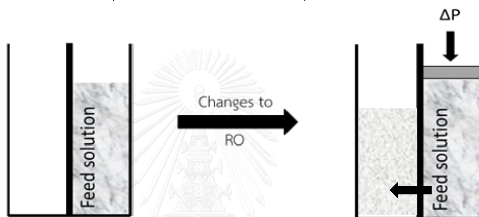
Figure 2.1 Reverse osmosis (RO) process[3].
