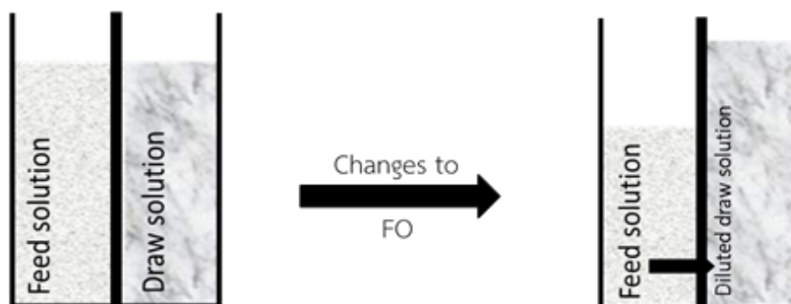
Figure 2.2 Forward osmosis (FO) process[3].
