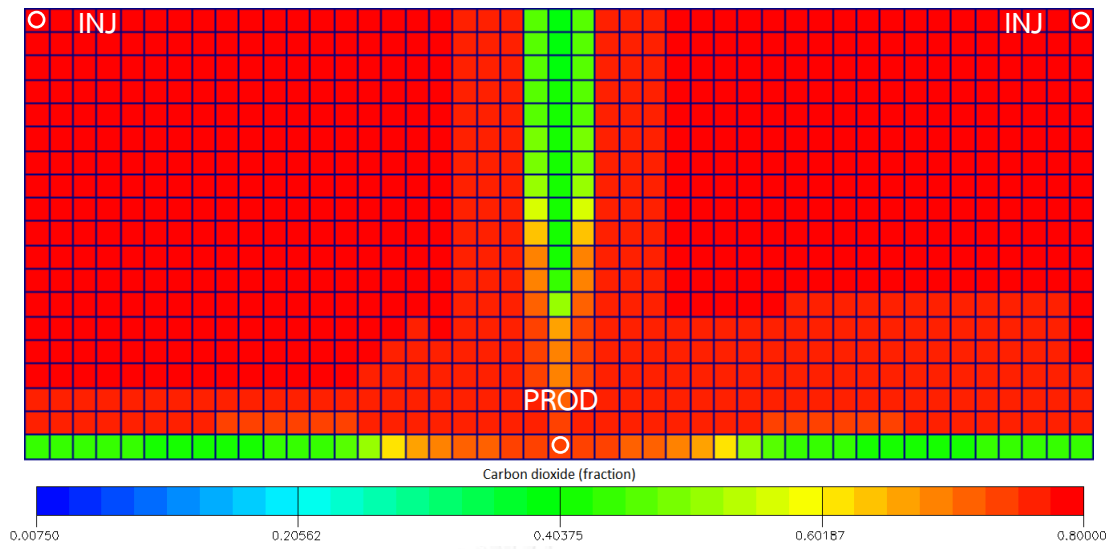
Figure 5.32 Carbon dioxide mole fraction distribution of case with gas injection rate of 1 MMscf/d of conventional gas injection with well patten 3 at the end of production
