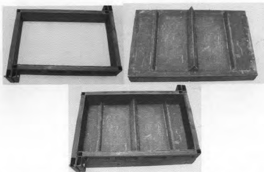
Figure 3.2: Existing specimen molds built from specifications
