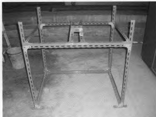
Figure 3.6: Steel stand for taking pictures
