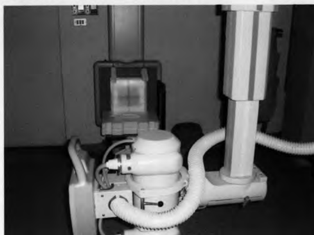
Figure 20. Perspex phantoms with test objects
