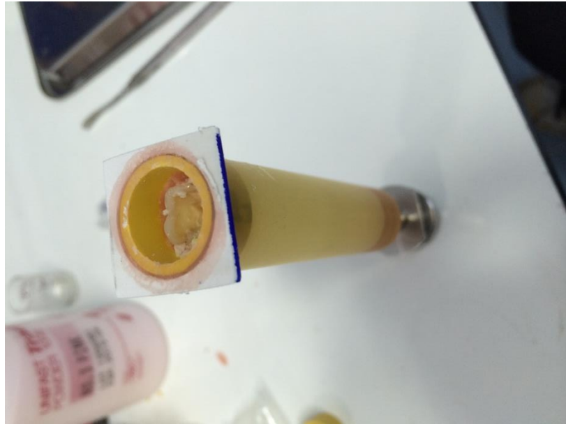
Figure 9: Plastic jig ensured horizontal and vertical orientation of sample.
