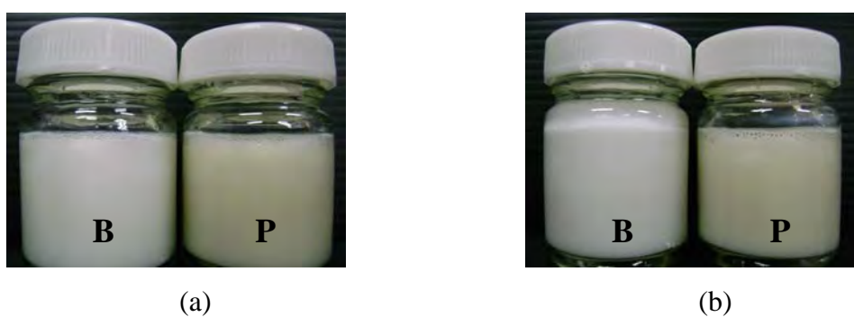
Figure 72 Freshly prepared SLN by w/o/w double emulsion method (a : using water as vehicle, b : using citrate buffer pH 5.5 as vehicle) (Left : Blank SLN, B and Right : SLN containing Puag-Haad, P)
