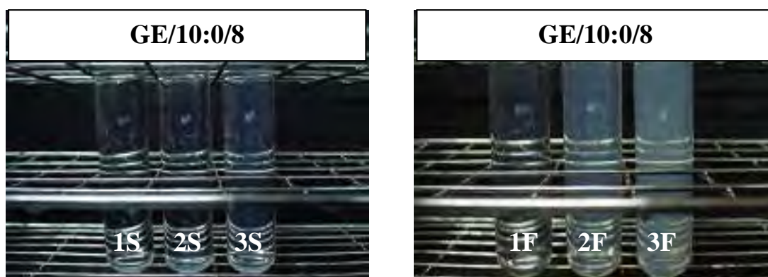
Figure 51 Freshly prepared blank SLN by w/o/w double emulsion method using gelucire ® 50/13 as lipid and S-40:F-68 mixed surfactant ratio of 10:0 (formula no. 8)
