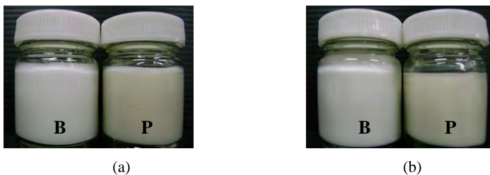
Figure 73 Freshly prepared SLN by cold homogenization method (a : using water as vehicle, b : using citrate buffer pH 5.5 as vehicle) (Left : Blank SLN, B and Right : SLN containing Puag-Haad, P)
