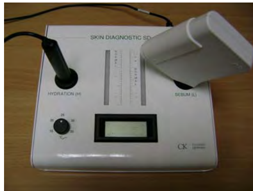
Figure 21 Skin Diagnostic ® SD 27, portable device with Corneometer ® and Sebumeter ® probe to measure the skin hydration and sebum content.
