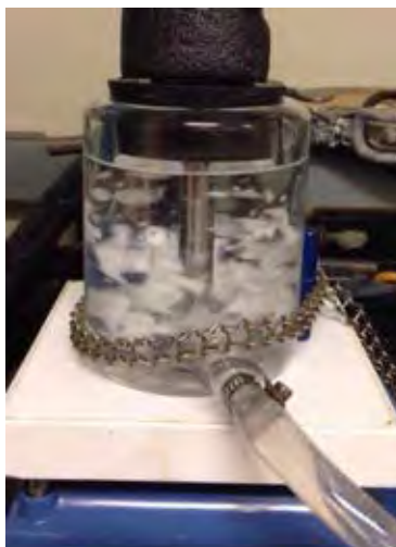
Figure 3.3 Michigan cold finger apparatus.
