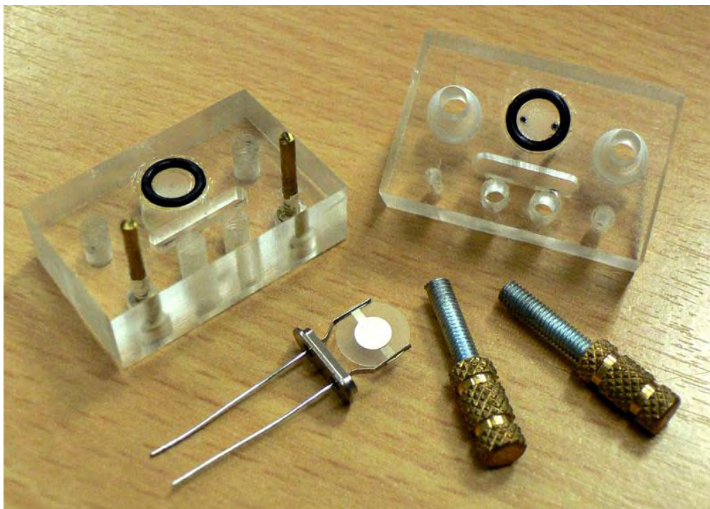
Figure 3.3 (a) A microchannel flowcell (b) parts.
