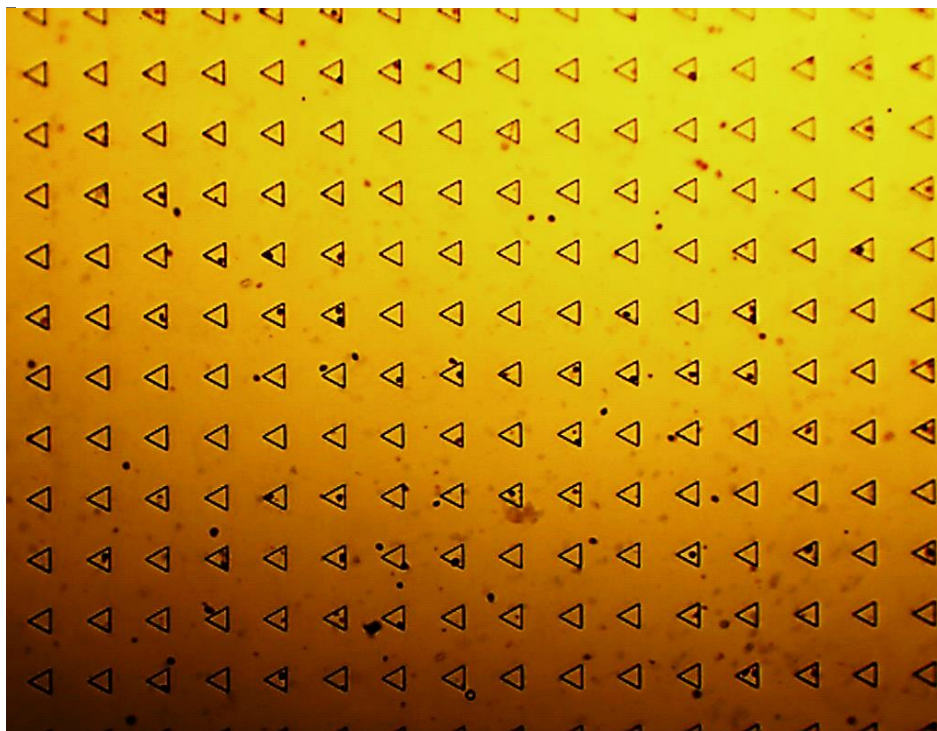
Figure 4. 26: At the scanning magnification power (4X), the exploit micrograph revealed the internal structure of the entrapment microdevice. Notably, it had a capability to entrapping single MCT cells in their microwell array (approximately 53.16%) and almost were single entrapments.
