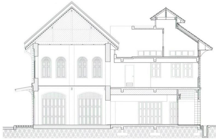
Figure 3-24. Section of newly refurbished shophouse.
