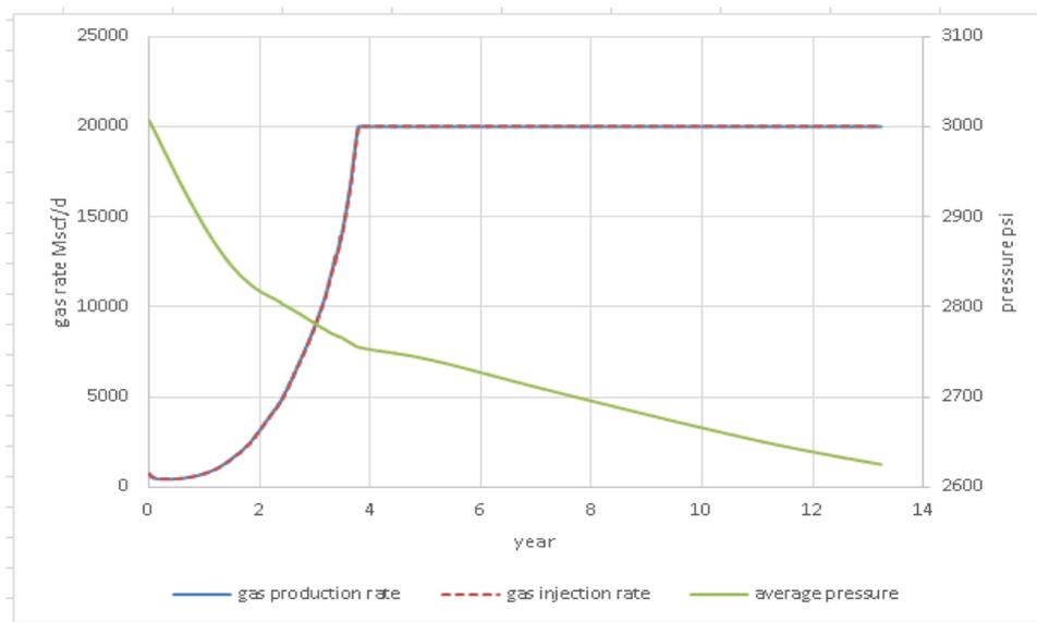
Figure 5.118 Trends of gas injection, gas production and average pressure for vertical well producer at 500 stb/d for production well on position 1
