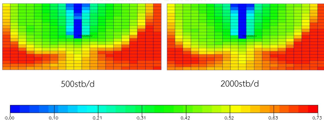
Figure 5.58 Oil saturation of plane  $k = 10$  at abandonment for vertical well under gas injection when  $P < 2500$  psi at different oil rates (xy plane view)
