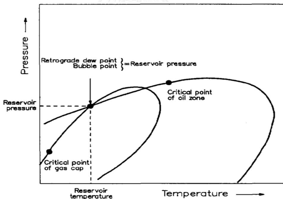
Figure 2.1 Pressure-temperature phase diagrams of gas cap and oil fluids in a reservoir that is initially at saturated conditions [1]
