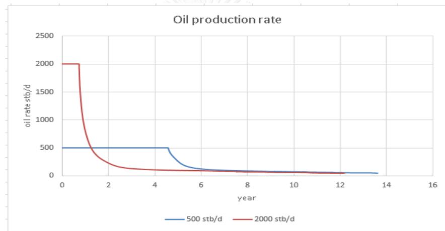
Figure 5.38 Oil production rate for horizontal well under gas reinjection
