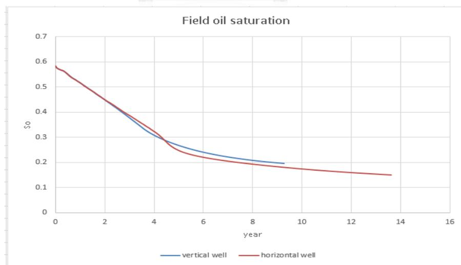
Figure 5.48 Average field oil saturation versus time for reservoir under gas injection using different well types
