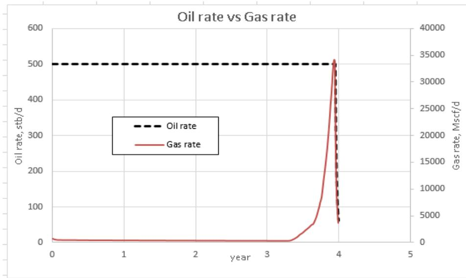
Figure 5.10 Oil rate profile, and gas rate profile of horizontal well producing at 500 stb/d
