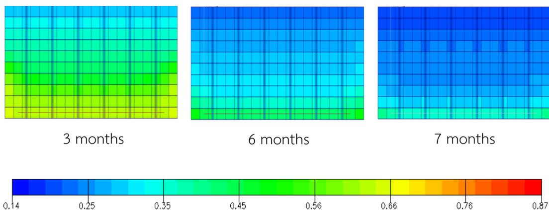
Figure A-12 Oil saturation versus time for grid plane  $j = 11$ : Fracture horizontal production well under natural depletion at 2000 stb/d (xz plane view)
