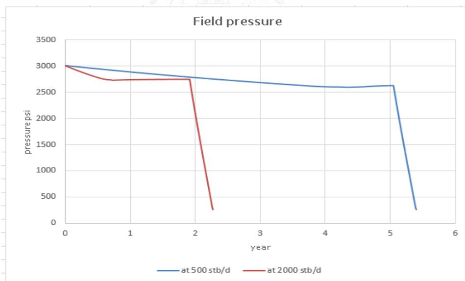
Figure 5.95 Field pressure for horizontal wells for production constrained at GOR < 80 Mscf/stb
