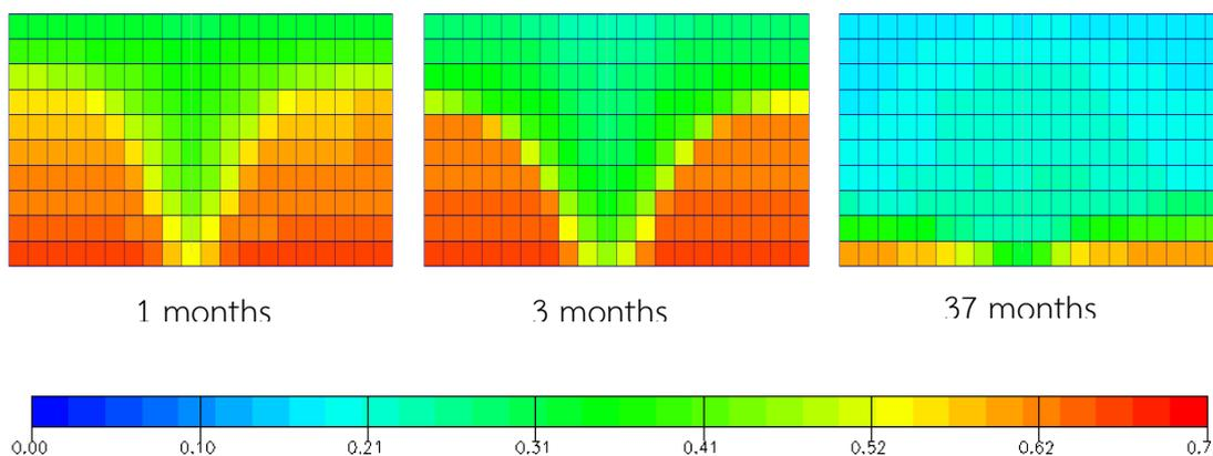
Figure A-27 Oil saturation versus time for grid plane  $j = 11$ : gas injection constrained at  $GOR < 80$  Mscf/stb and vertical production well at 2000 stb/d (xz plane view)
