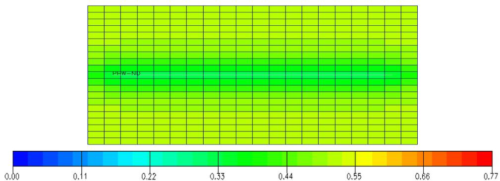
Figure 5.26 Oil saturation at abandonment for reservoir with a horizontal well under natural depletion at 500 stb/d (xy plane view)
