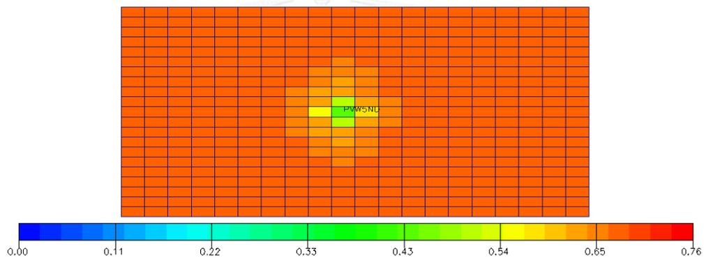
Figure 5.25 Oil saturation at abandonment for reservoir with a vertical well under natural depletion at 500 stb/d (xy plane view)
