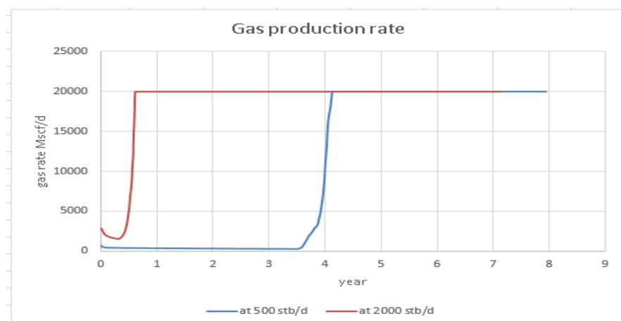
Figure 5.78 Gas production rate for horizontal well under gas reinjection at pressure lower than 1500 psi
