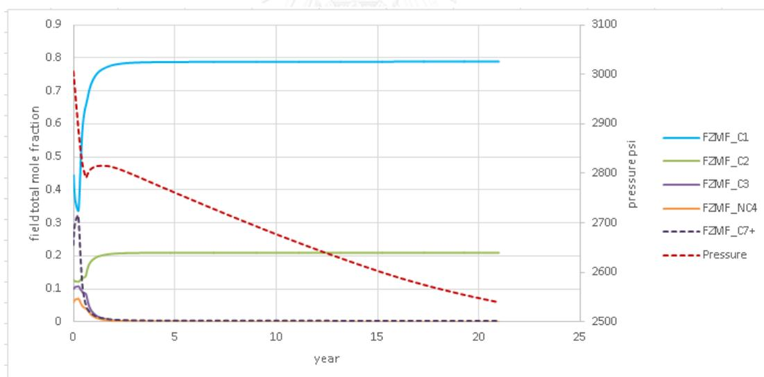
Figure B-18 Field total mole fraction and reservoir pressure vs time for the case of gas injection with production using well position 1 using horizontal well at 2000 stb/d
