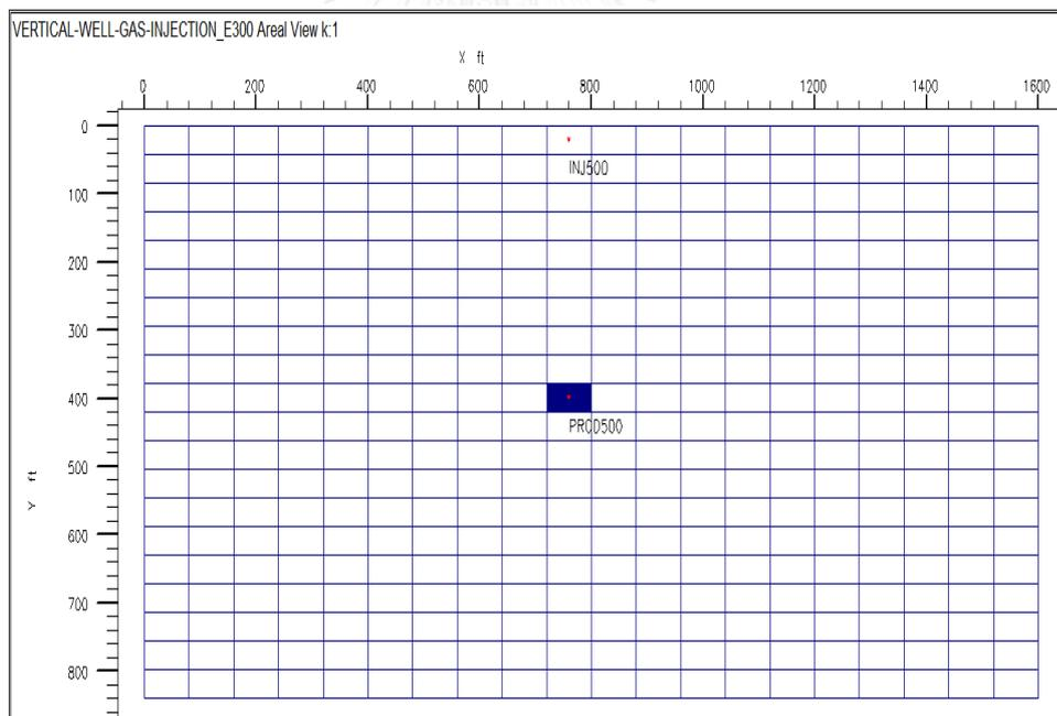
Figure 4.8 Top view (xy plane) for one vertical producing well (PROD500) and one vertical gas injection well (INJ500).
