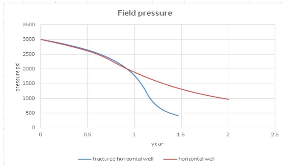
Figure 5.23 Field pressure for different well types in a tight reservoir under natural depletion
