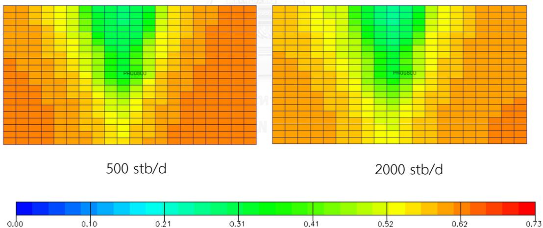
Figure 5.91 Oil saturation of plane k = 10 at abandonment for vertical well under gas injection constrained at GOR<80 Mscf/stb at different oil rates (xy plane view)
