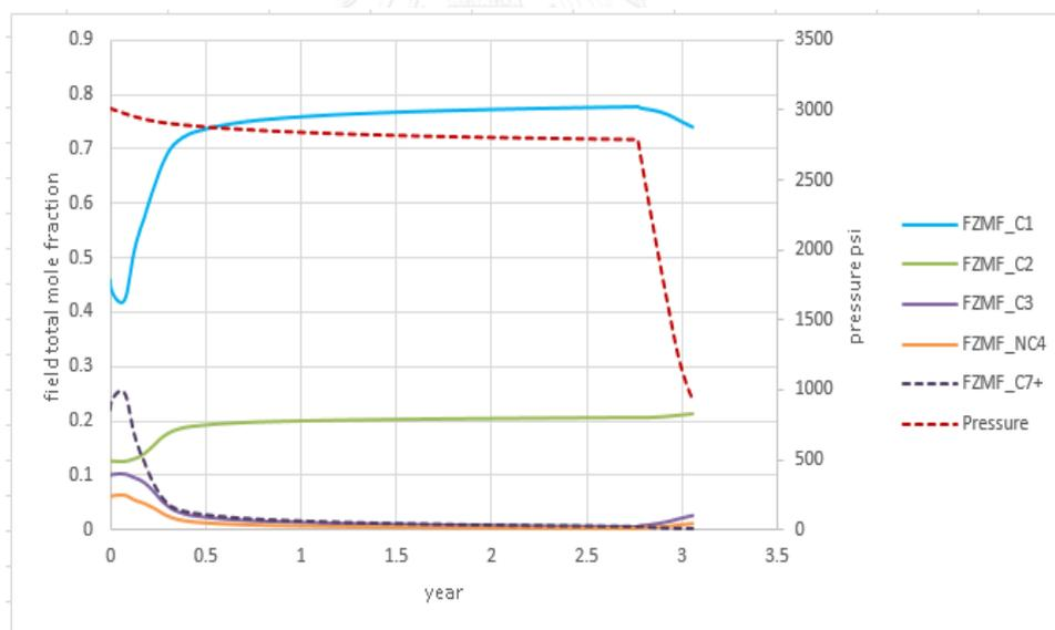
Figure B-12 Field total mole fraction and reservoir pressure vs time for the case of gas injection terminated when GOR > 80 Mscf/stb using vertical well at 2000 stb/d
