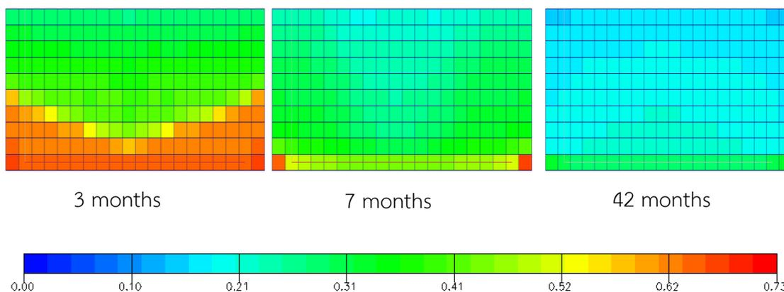
Figure A-39 Oil saturation versus time for grid plane  $j = 11$ : gas injection constrained at  $\text{GOR} < 160$  Mscf/stb and horizontal production well at 2000 stb/d (xz plane view)
