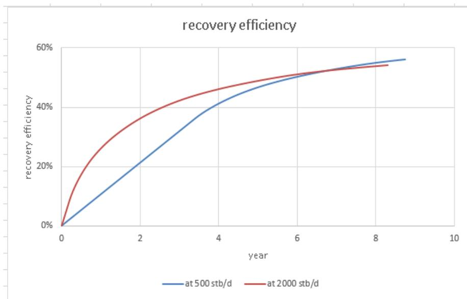
Figure 6.5 Field oil efficiency for vertical well at position 2 under produced gas reinjection
