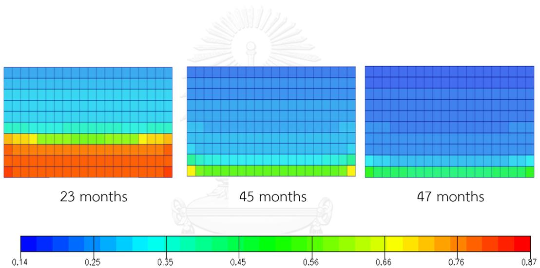
Figure 5.12 Oil saturation versus time for grid plane  $j = 11$ : Horizontal production well at 500 stb/d (xz plane view)
