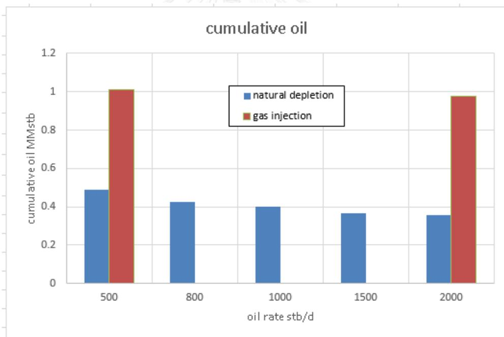
Figure 5.36 Cumulative oil for vertical well under natural depletion and gas injection
