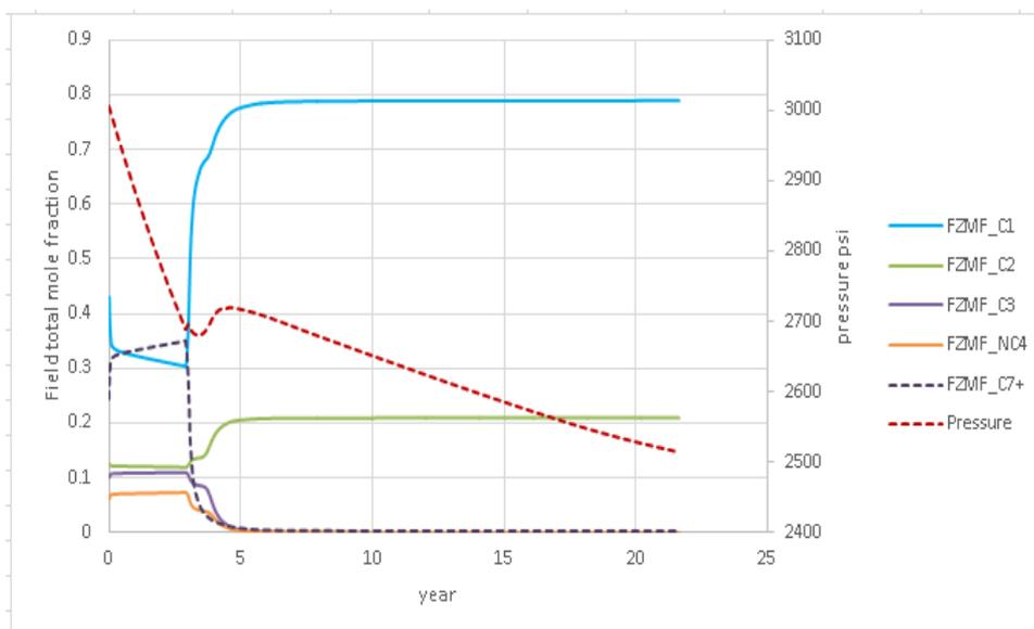
Figure B-17 Field total mole fraction and reservoir pressure vs time for the case of gas injection with production using well position 1 using horizontal well at 500 stb/d
