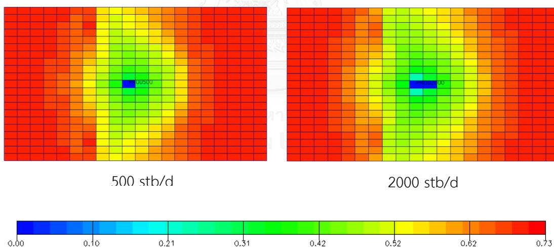
Figure 6.6 Oil saturation profile for grid plane k-10 at abandonment for vertical well at position 2 (xy plane view)
