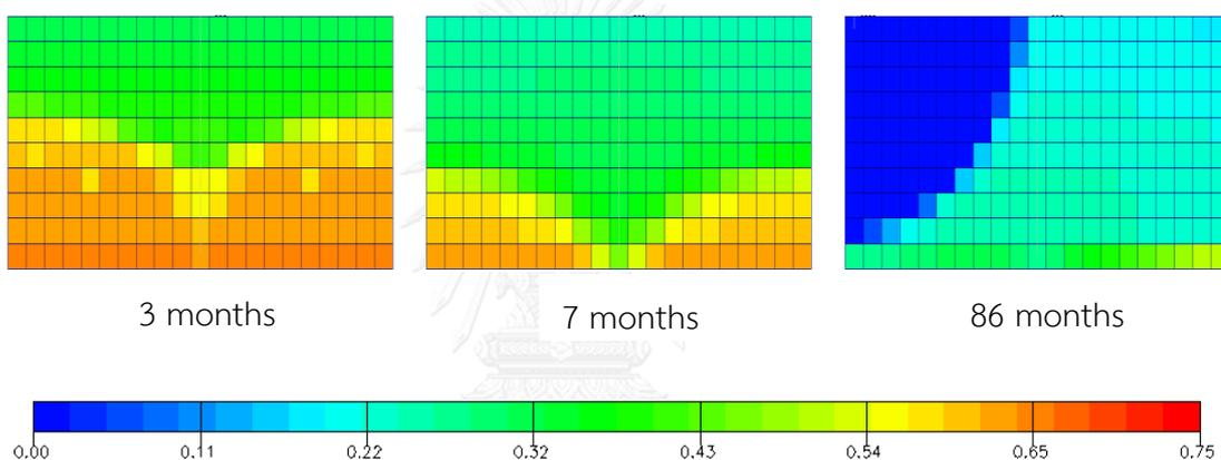
Figure A-25 Oil saturation versus time for grid plane  $i = 10$ : gas injection when  $P < 1500$  psi and horizontal production well at 2000 stb/d (yz plane view)
