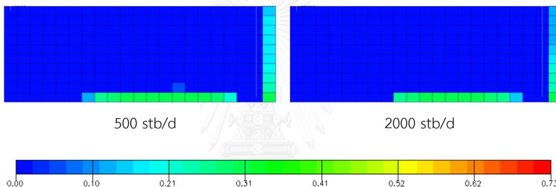
Figure A-43 Oil saturation at end of production for plane  $i = 10$ : gas injection scenario and vertical production well in position 1 for different oil rates (yz plane view)
