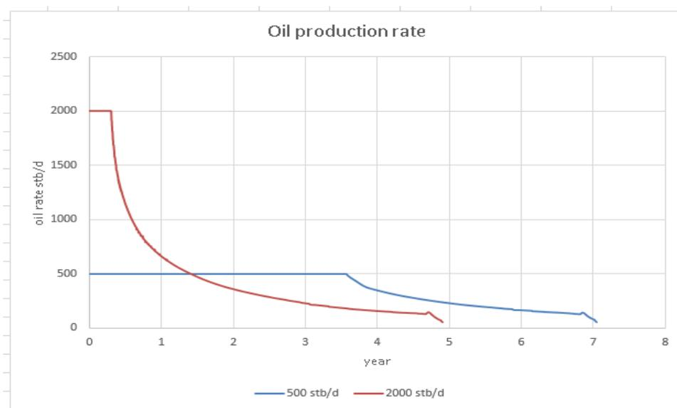
Figure 5.99 Oil production rate for vertical wells: production constrained at  $GOR < 160$  Mscf/stb
