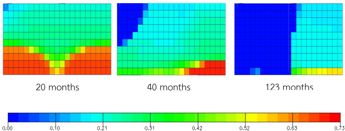
Figure A-18 Oil saturation versus time for grid plane  $i = 10$ : gas injection when  $P < 2500$  psi and vertical production well at 500 stb/d (yz plane view)
