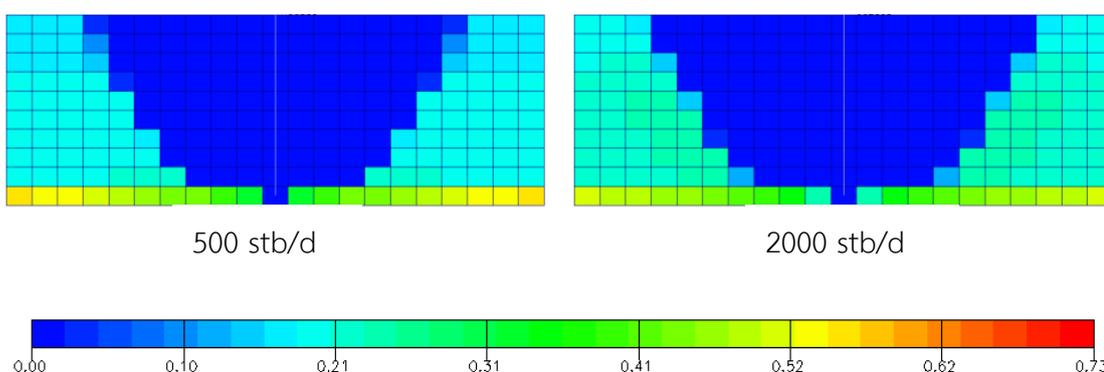
Figure A-47 Oil saturation at end of production for plane  $i = 10$ : gas injection scenario and vertical production well in position 2 for different oil rates (yz plane view)
