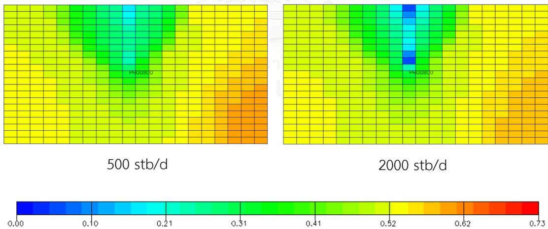
Figure 5.104 Oil saturation of plane k = 10 at abandonment for vertical well under gas injection constrained at GOR<160 Mscf/stb at different oil rates (xy plane view)
