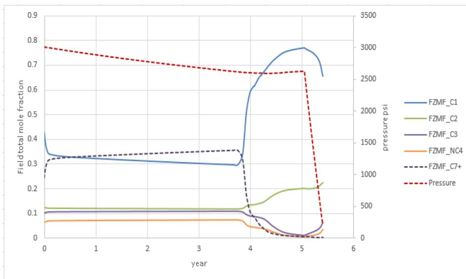
Figure B-13 Field total mole fraction and reservoir pressure vs time for the case of gas injection terminated when  $GOR > 80$  Mscf/stb using horizontal well at 500 stb/d
