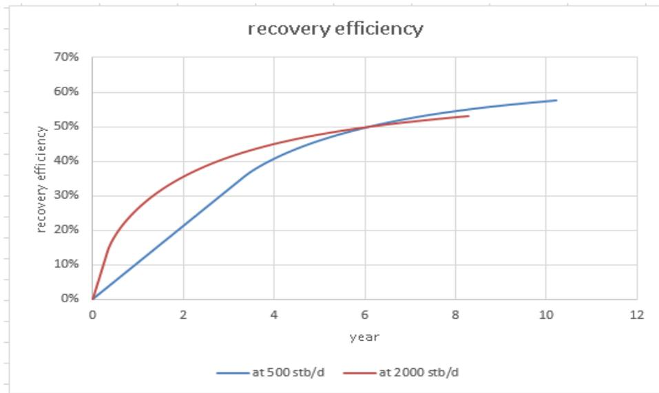
Figure 5.54 Field oil efficiency for vertical well under gas reinjection at pressure lower than 2500 psi
