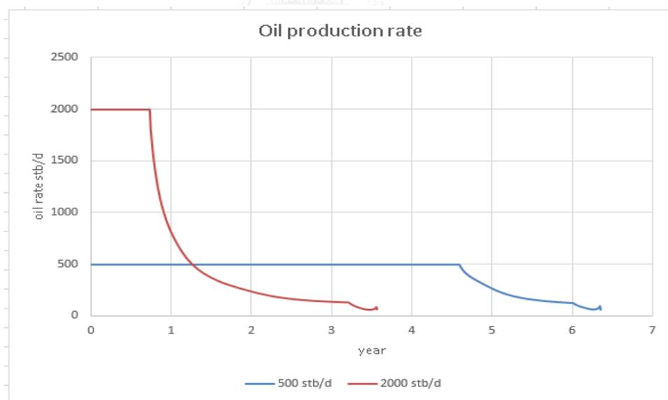
Figure 5.106 Oil production rate for horizontal wells: production constrained at  $GOR < 160$  Mscf/stb
