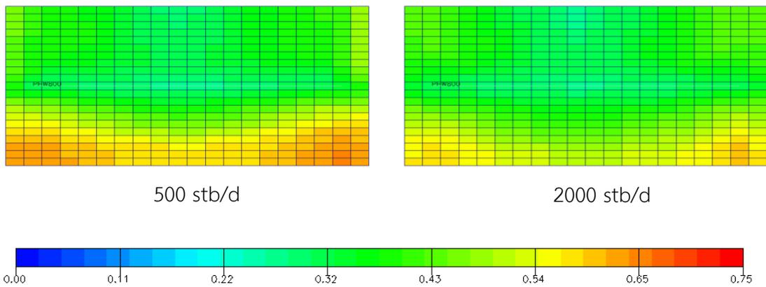
Figure 5.83 Oil saturation of plane  $k = 10$  at abandonment for horizontal well under gas injection when  $P < 1500$  psi at different oil rates (xy plane view)
