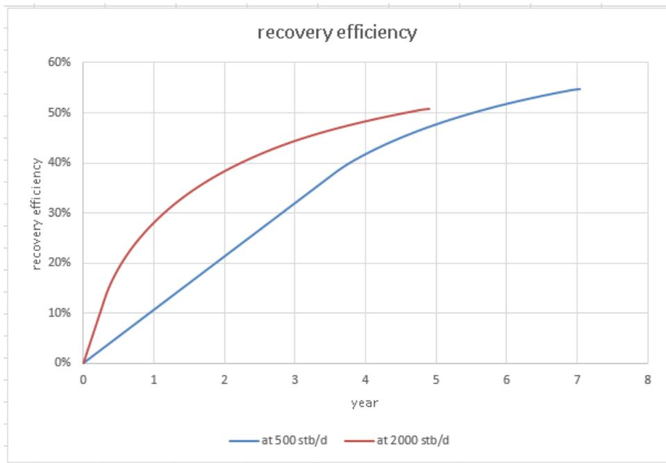
Figure 5.103 Field oil efficiency for vertical wells: production constrained at GOR<160 Mscf/stb
