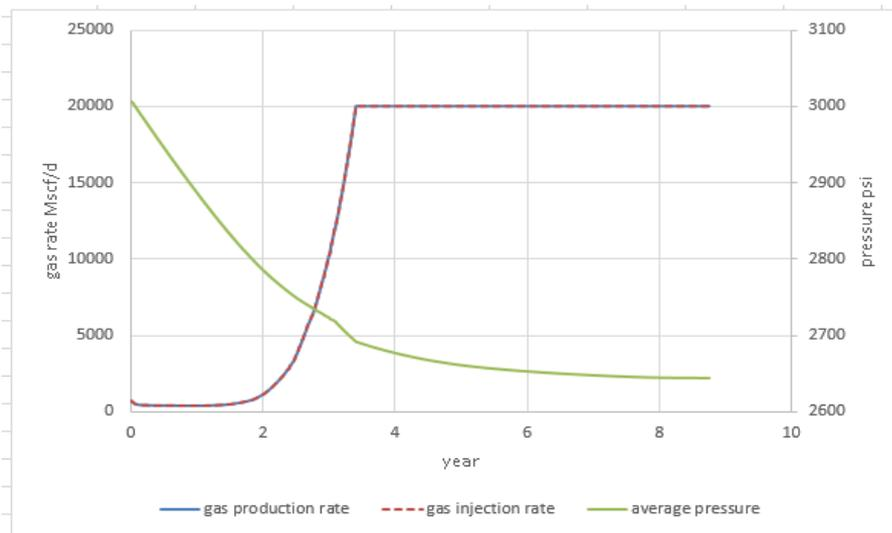
Figure 6.1 Trends of gas injection, gas production and average pressure for vertical well producer at 500 stb/d: production well on position 2
