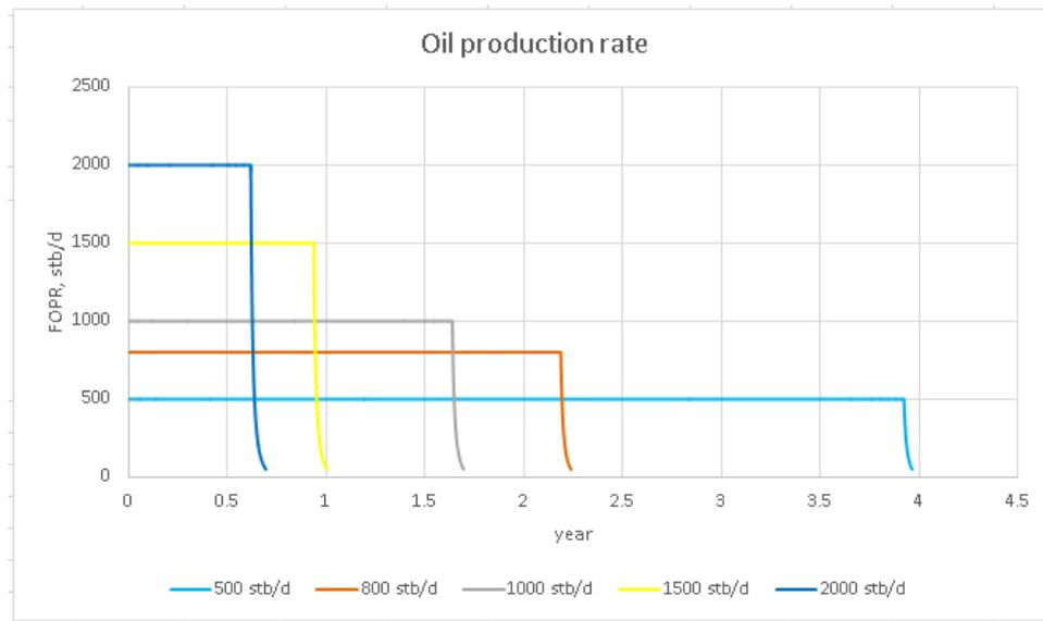
Figure 5.13 Oil production rate of fractured horizontal well under natural depletion
