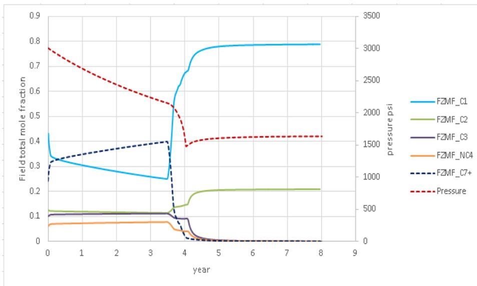
Figure B-9 Field total mole fraction and reservoir pressure vs time for the case of gas injection when pressure drops below 1500 psi using horizontal well at 500 stb/d
