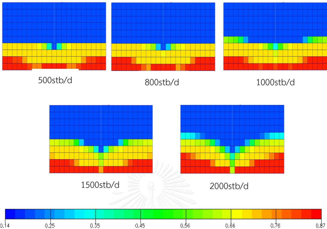
Figure A-13 Comparison of oil saturation profile for fractured plane (plane  $i = 7$ ) at mid plateau production for different oil rates (yz plane view)
