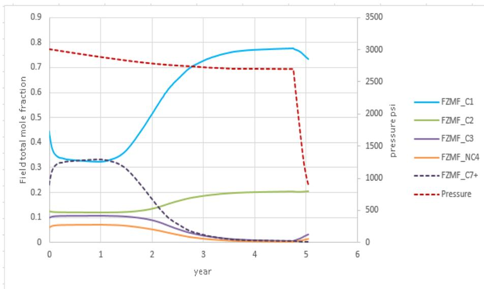
Figure B-11 Field total mole fraction and reservoir pressure vs time for the case of gas injection terminated when GOR > 80 Mscf/stb using vertical well at 500 stb/d
