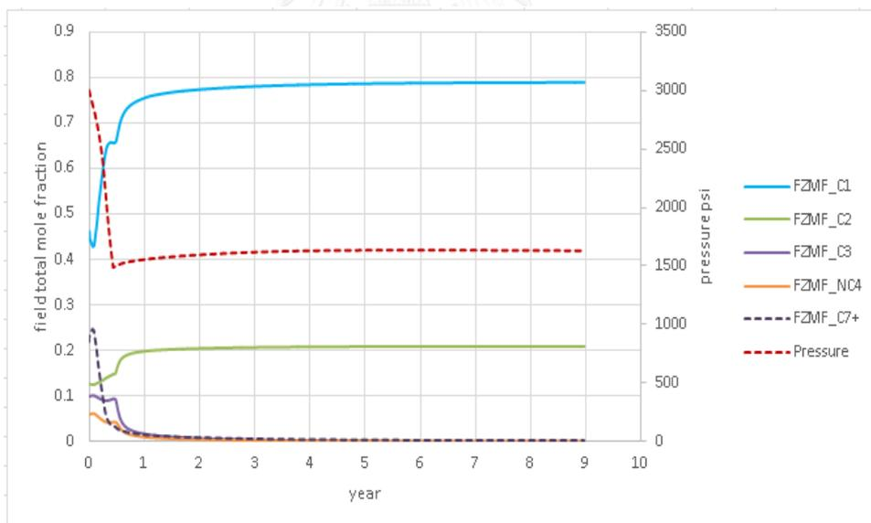
Figure B-8 Field total mole fraction and reservoir pressure vs time for the case of gas injection when pressure drops below 1500 psi using vertical well at 2000 stb/d
