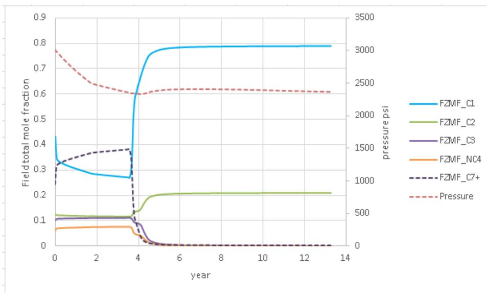
Figure B-5 Field total mole fraction and reservoir pressure vs time for the case of gas injection when pressure drops below 2500 psi using horizontal well at 500 stb/d
