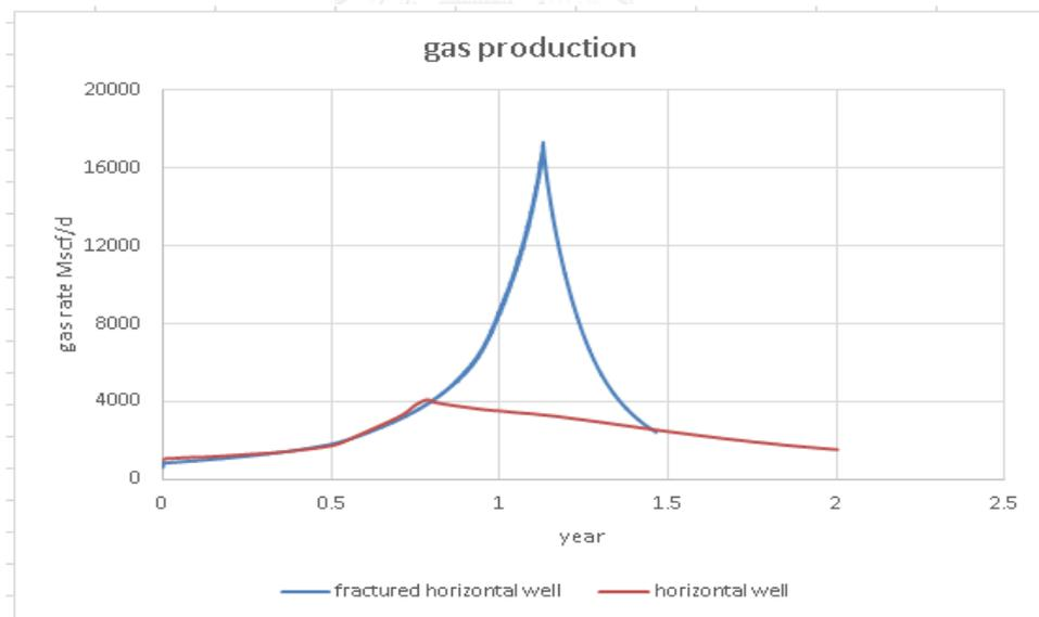
Figure 5.22 Gas production for different well types in a tight reservoir under natural depletion
