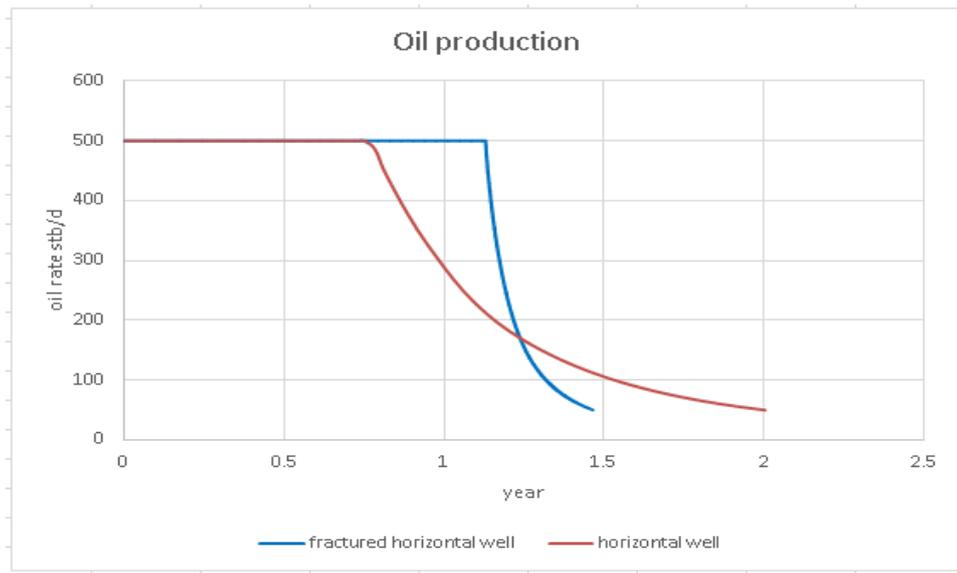
Figure 5.21 Oil production for different well types in a tight reservoir under natural depletion
