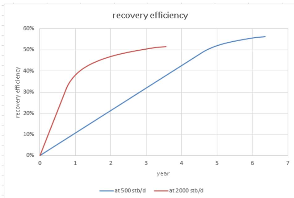
Figure 5.109 Field oil efficiency for horizontal wells: production constrained at  $GOR < 160$  Mscf/stb
