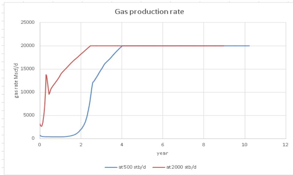
Figure 5.69 Gas production rate for vertical wells under gas reinjection at pressure lower than 1500 psi
