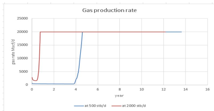
Figure 5.39 Gas production rate for horizontal well under gas reinjection at different oil rates
