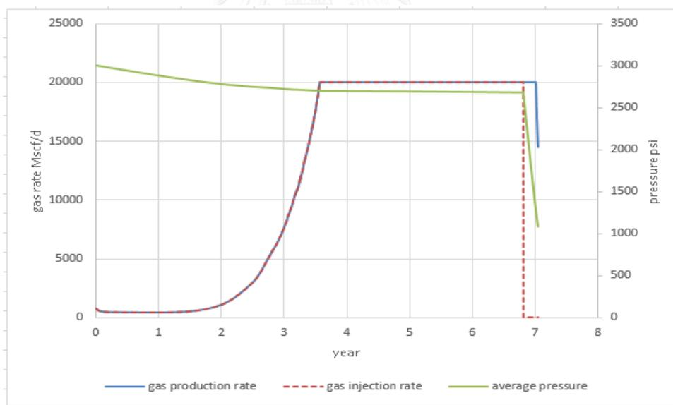
Figure 5.102 Trends of gas injection, gas production and average pressure for vertical well producer at 500 stb/d: gas injection constrained at GOR<160 Mscf/stb
