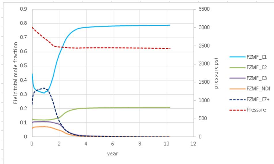
Figure B-3 Field total mole fraction and reservoir pressure vs time for the case of gas injection when pressure drops below 2500 psi using vertical well at 500 stb/d
