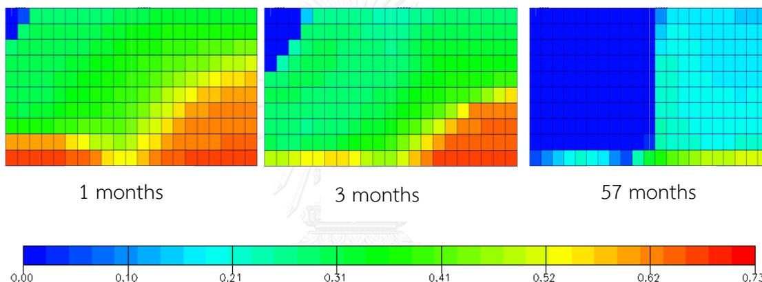
Figure A-37 Oil saturation versus time for grid plane  $i = 10$ : gas injection constrained at  $GOR < 160$  Mscf/stb and vertical production well at 2000 stb/d (yz plane view)
