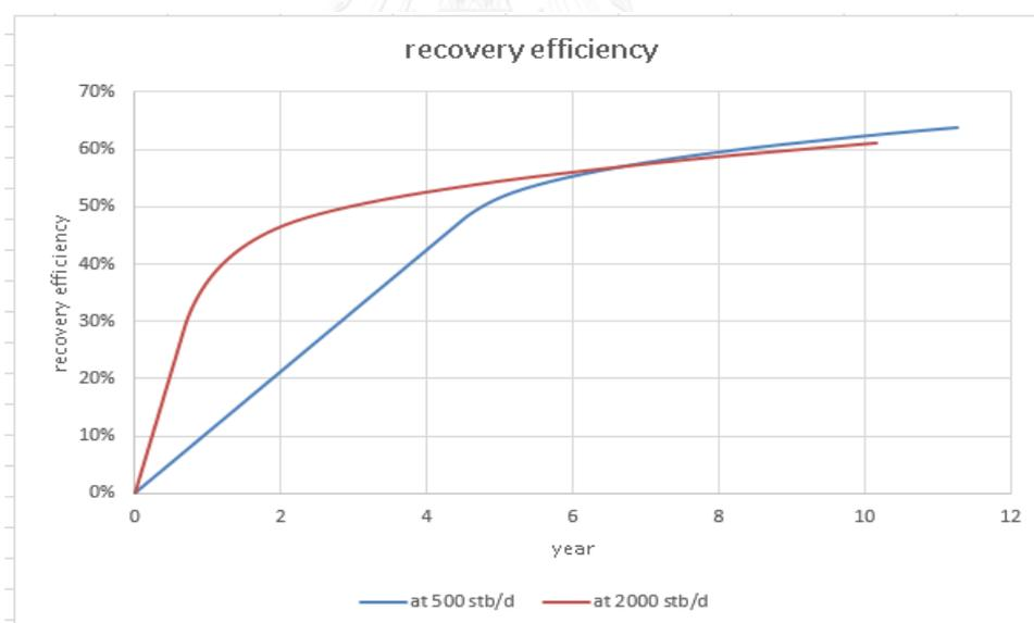
Figure 6.10 Field oil efficiency for horizontal well at position 2 under produced gas reinjection
