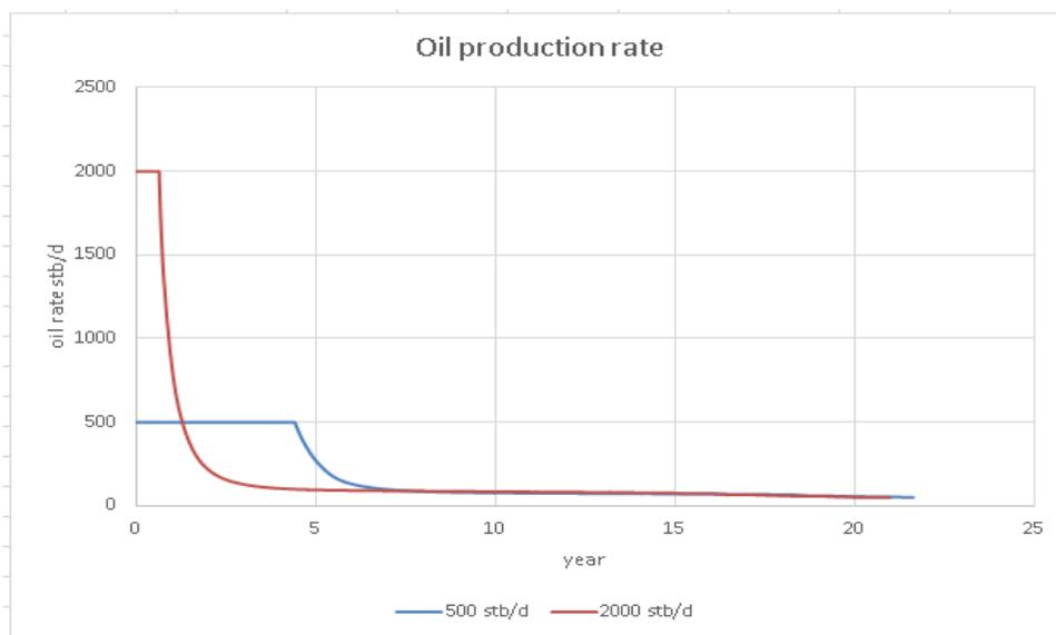
Figure 5.122 Oil production rate for horizontal well at position 1 under produced gas reinjection
