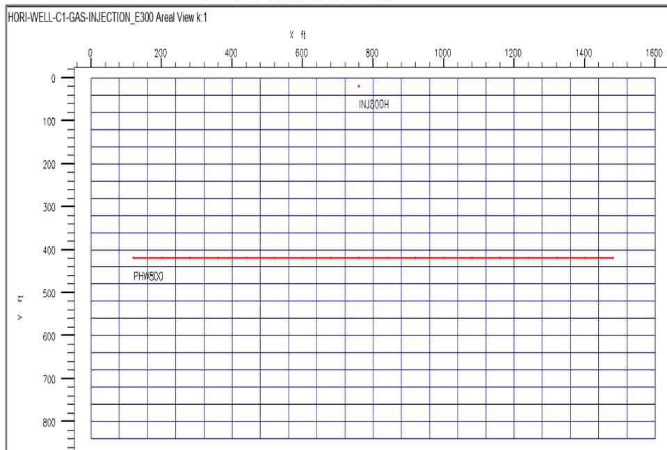
Figure 4.10 Top view (xy plane) for one horizontal producing well (PHW800) and one vertical gas injection well (INJ800H).
