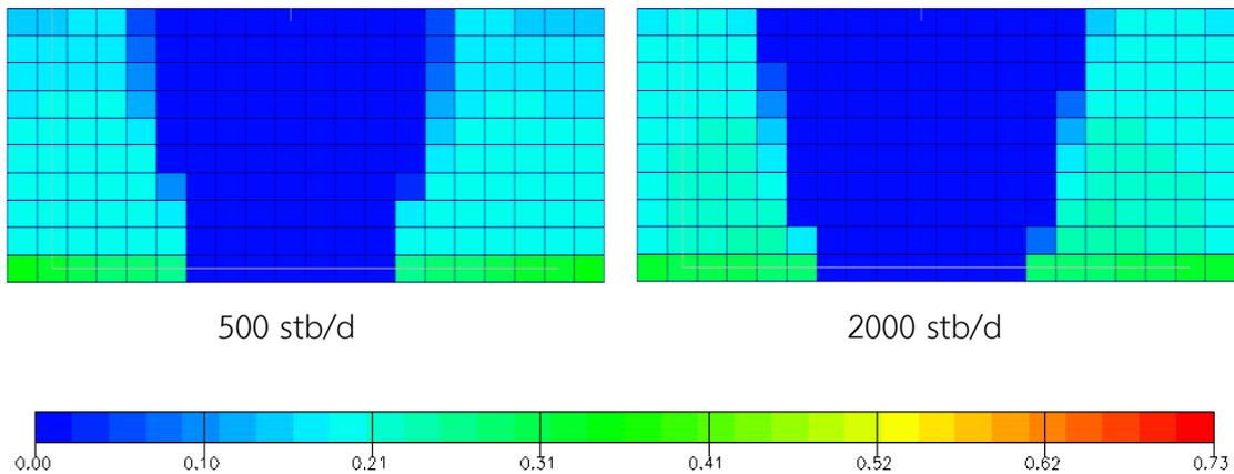
Figure A-48 Oil saturation at end of production for plane  $j = 11$ : gas injection scenario and horizontal production well in position 2 for different oil rates (xz plane view)
