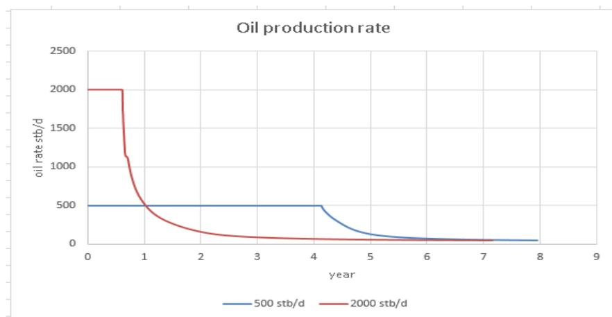
Figure 5.77 Oil production rate for horizontal well under gas reinjection at pressure lower than 1500 psi
