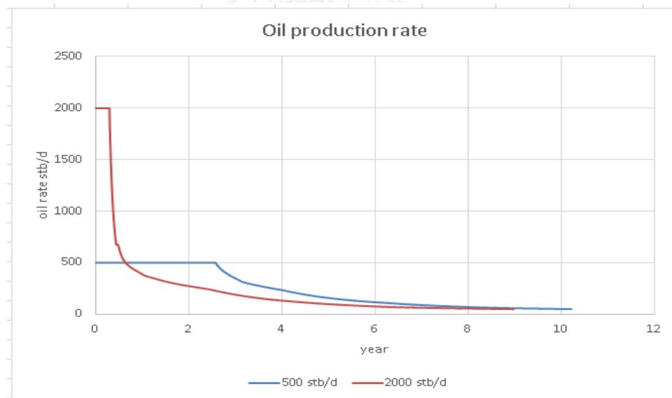
Figure 5.68 Oil production rate for vertical well under gas reinjection at pressure lower than 1500 psi
