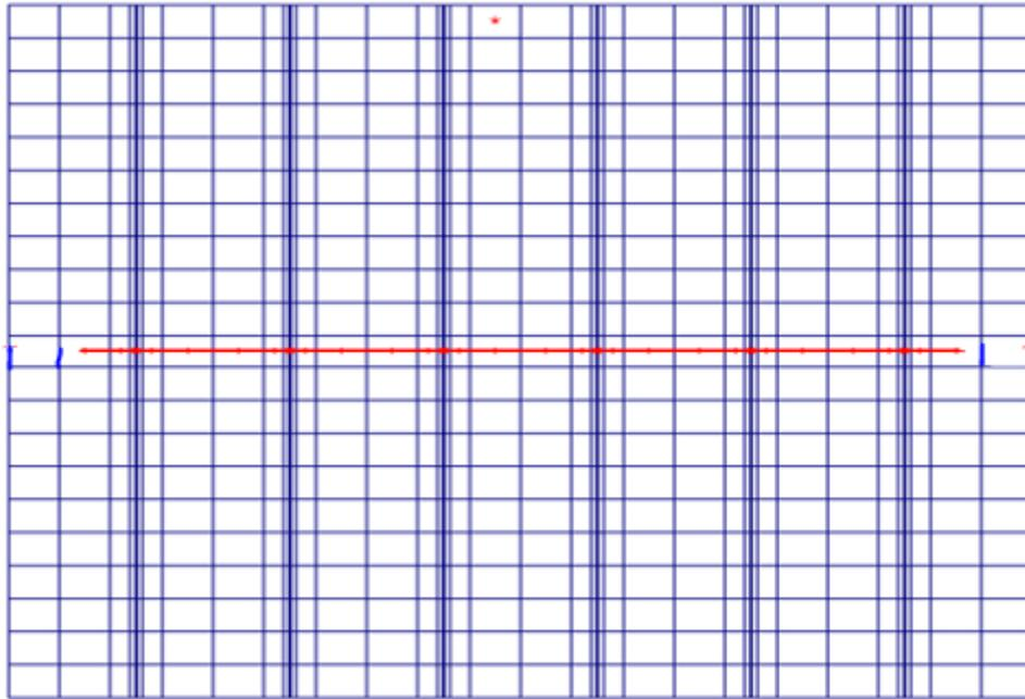
Figure 4.11 Top view (xy plane) one fractured horizontal producing well and one vertical gas injection well.
