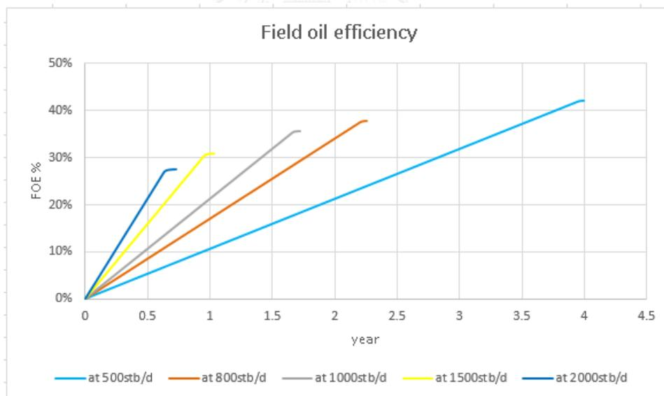
Figure 5.9 Field oil efficiency of horizontal well under natural depletion different oil rates
