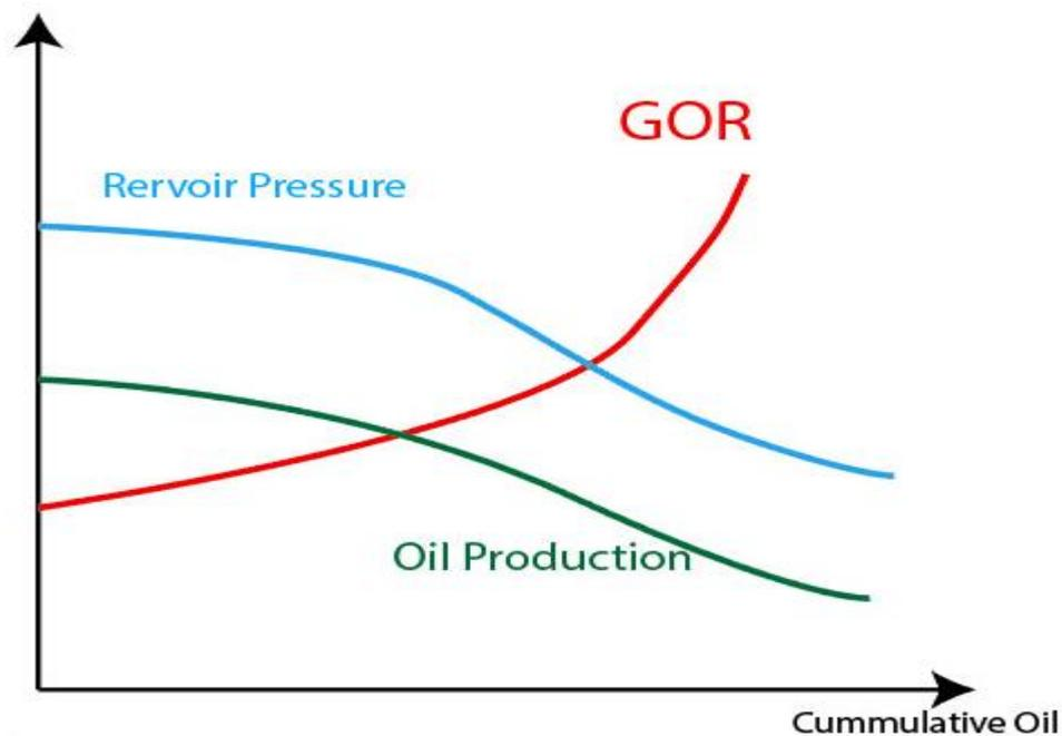
Figure 2.2 Typical production GOR, pressure and water cut profile for gas cap reservoirs [4]
