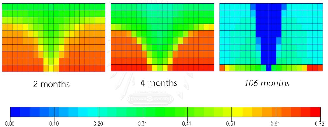
Figure 5.34 Oil saturation versus time for grid plane  $j = 11$  gas injection with vertical production well at 2000 stb/d (xz plane view)
