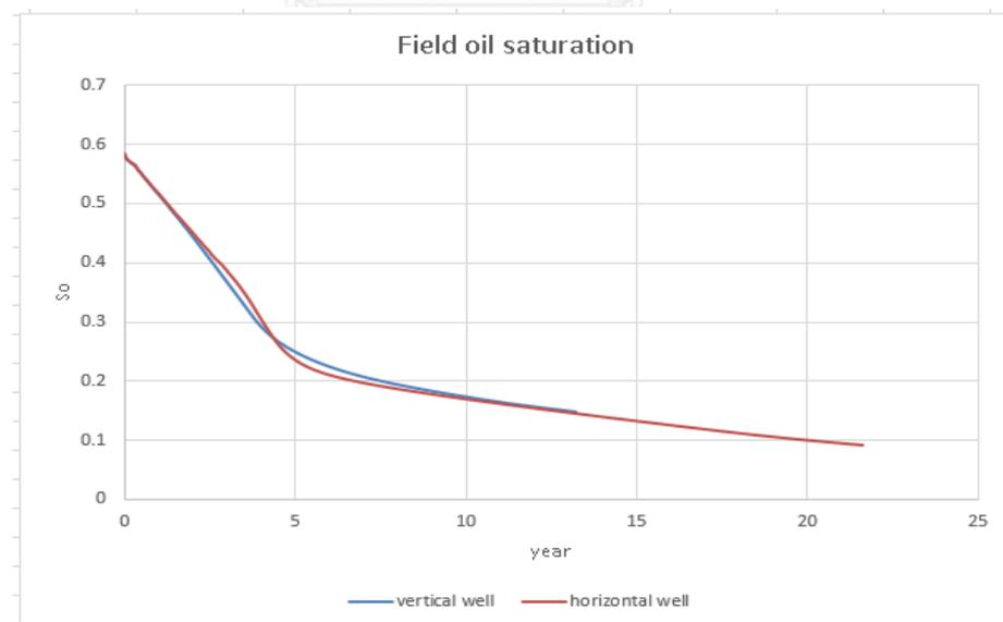
Figure 5.127 Average field oil saturation versus time for reservoir under gas injection: position 1 configuration
