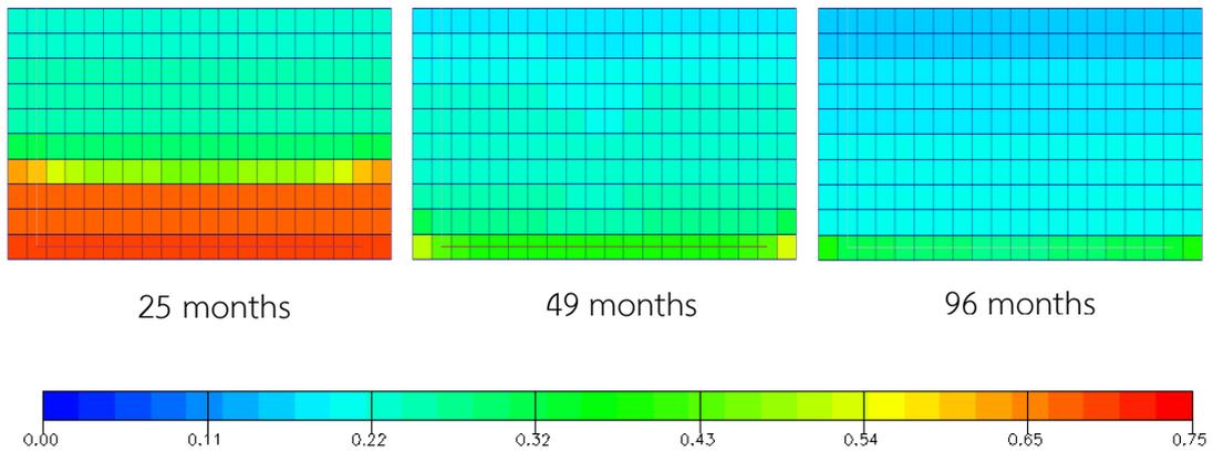
Figure 5.81 Oil saturation versus time for grid plane  $j = 11$ : gas injection when  $P < 1500$  psi with horizontal production well at 500 stb/d (xz plane view)
