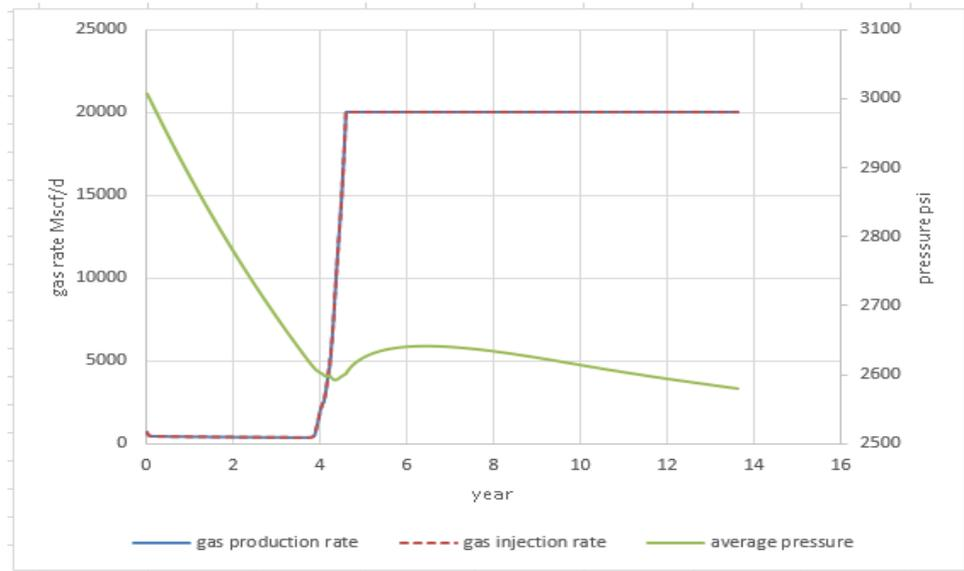
Figure 5.42 Trends of gas injection, gas production and average pressure for horizontal well producer at 500 stb/d: gas injection scenario
