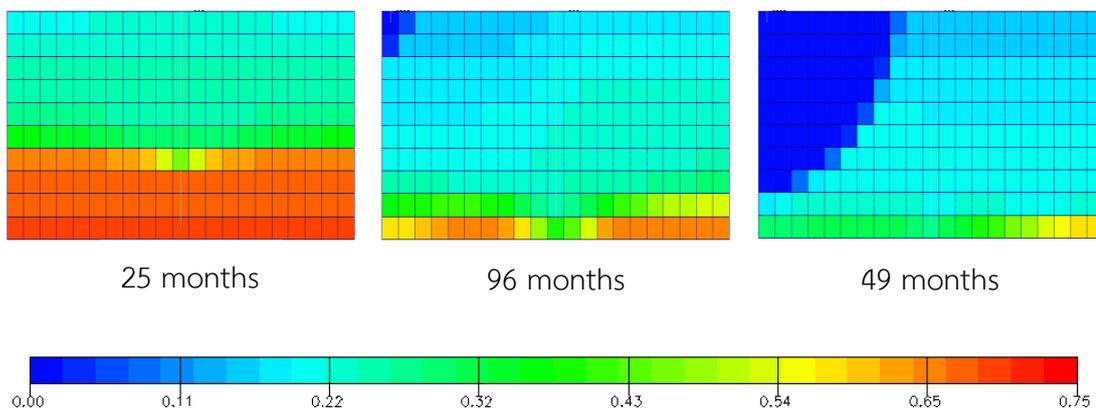
Figure A-24 Oil saturation versus time for grid plane  $i = 10$ : gas injection when  $P < 1500$  psi and horizontal production well at 500 stb/d (yz plane view)
