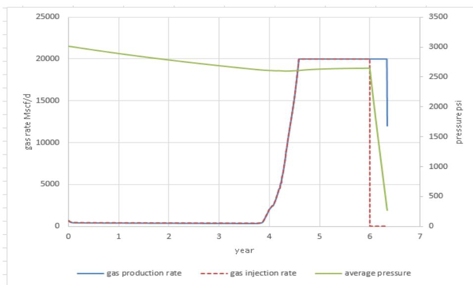
Figure 5.105 Trends of gas injection, gas production and average pressure for horizontal well producer at 500 stb/d: gas injection constrained at  $GOR < 160$  Mscf/stb
