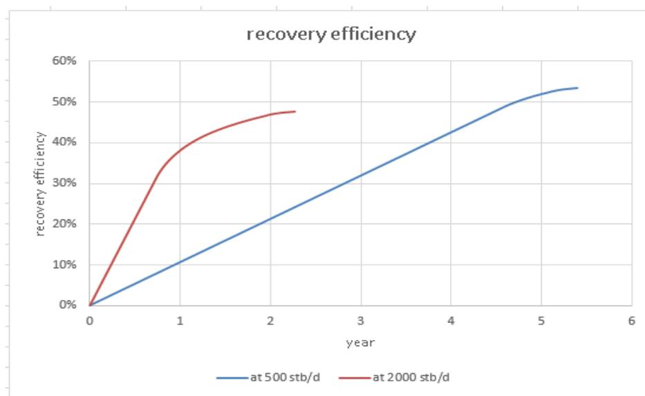
Figure 5.96 Field oil efficiency for horizontal wells for production constrained at GOR<80 Mscf/stb
