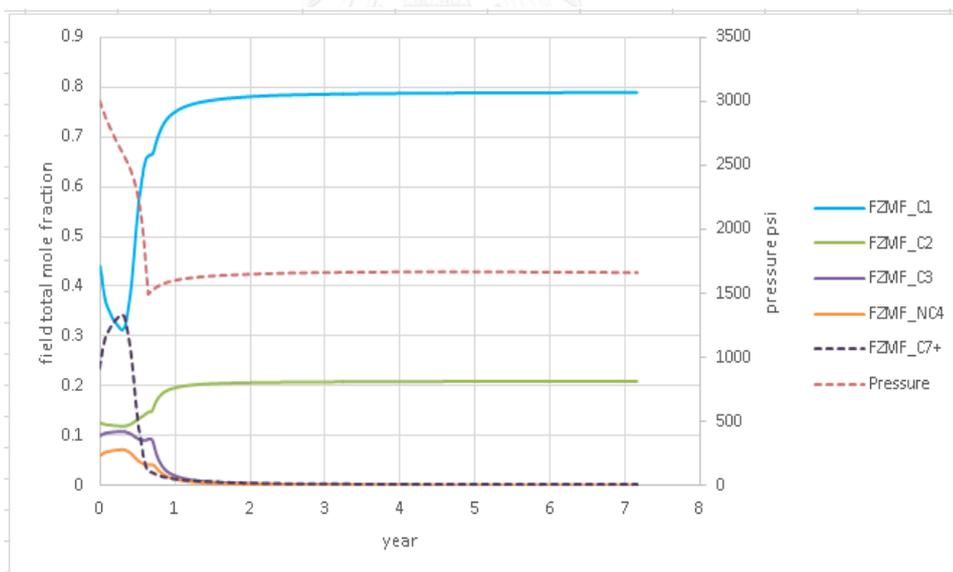
Figure B-10 Field total mole fraction and reservoir pressure vs time for the case of gas injection when pressure drops below 1500 psi using horizontal well at 2000 stb/d
