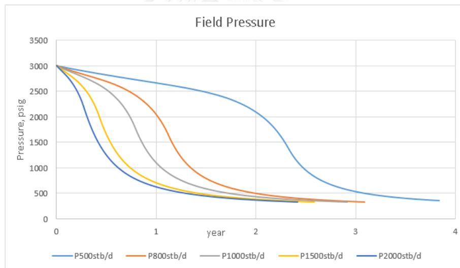
Figure 5.3 Field pressure of the vertical well under natural depletion at different oil rates.
