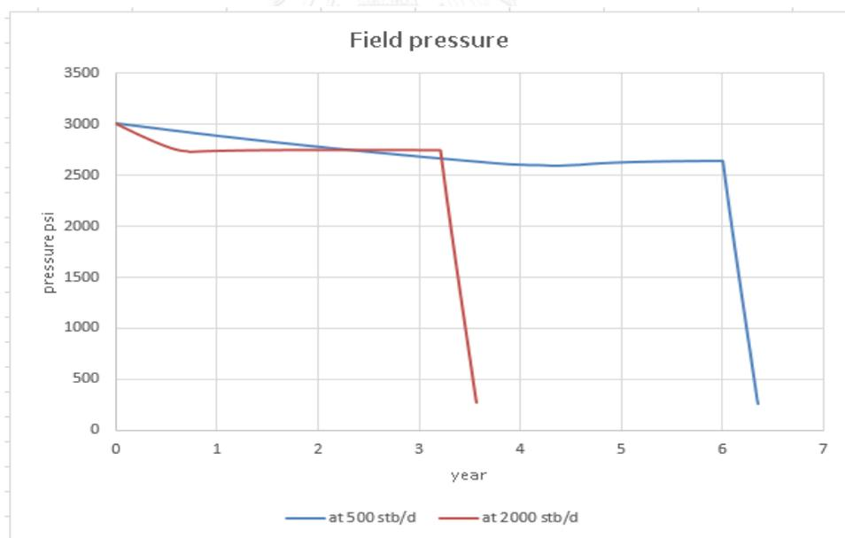
Figure 5.108 Field pressure for horizontal wells: production constrained at GOR<160 Mscf/stb
