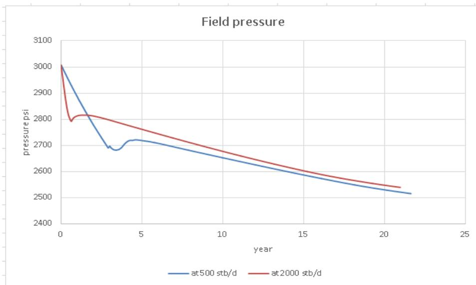
Figure 5.124 Field pressure for horizontal well at position 1 under produced gas reinjection
