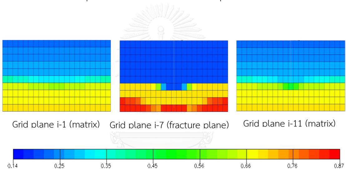
Figure 5.18 Comparison of oil saturation of a fractured plane and non-fractured plane at mid plateau of production for fractured horizontal well at 500 stb/d ( $yz$  plane view)
