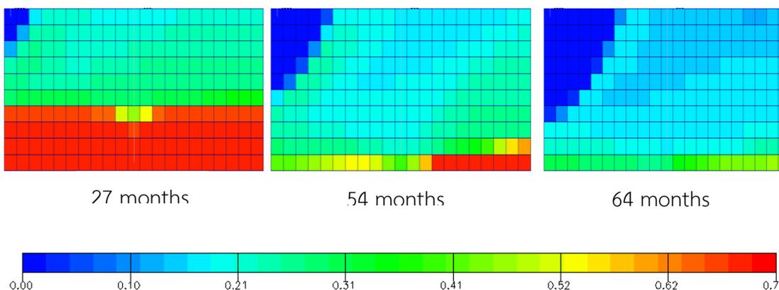
Figure A-32 Oil saturation versus time for grid plane  $i = 10$ : gas injection constrained at  $GOR < 80$  Mscf/stb and horizontal production well at 500 stb/d (yz plane view)
