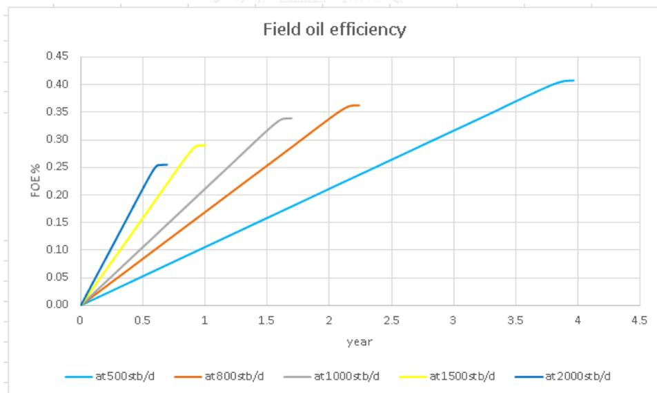
Figure 5.16 Field oil efficiency of fractured horizontal well under natural depletion at different oil rates
