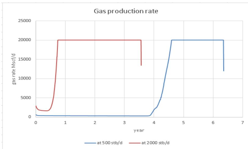
Figure 5.107 Gas production rate for horizontal wells: production constrained at GOR<160 Mscf/stb
