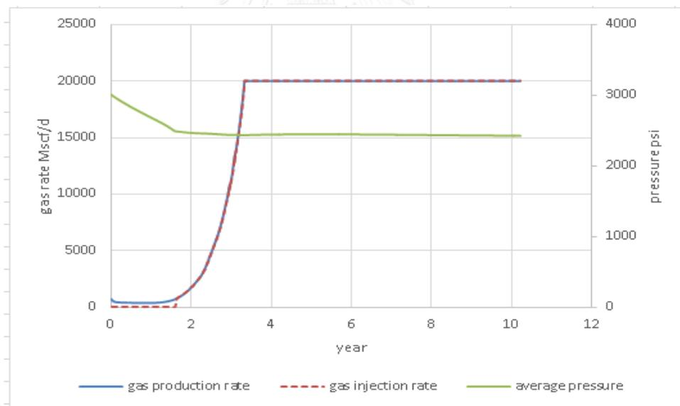
Figure 5.55 Trends of gas injection, gas production and average pressure for vertical well producer at 500 stb/d: gas injection when  $P < 2500$  psi scenario
