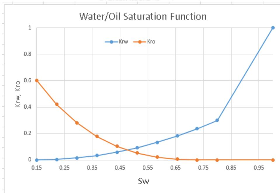
Figure 4.6 Water/Oil Saturation Function
