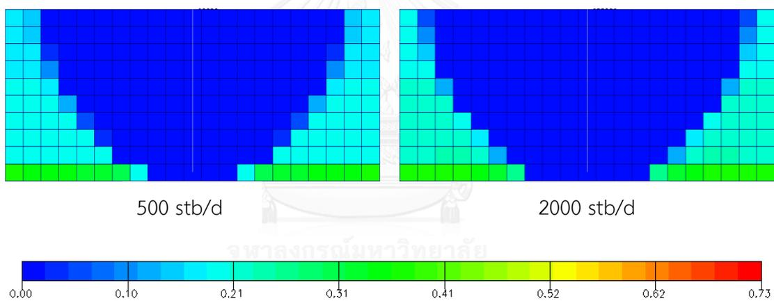
Figure A-49 Oil saturation at end of production for plane  $i = 10$ : gas injection scenario and horizontal production well in position 2 for different oil rates (yz plane view)
