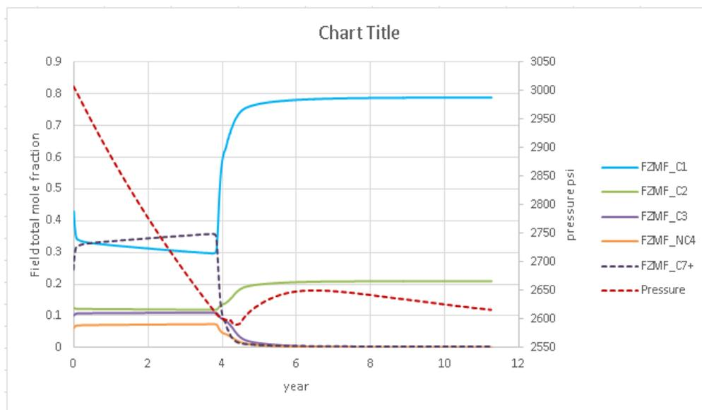
Figure B-19 Field total mole fraction and reservoir pressure vs time for the case of gas injection with production using well position 2 using horizontal well at 500 stb/d
