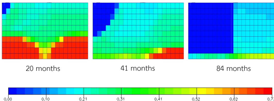
Figure A-36 Oil saturation versus time for grid plane  $i = 10$ : gas injection constrained at  $GOR < 160$  Mscf/stb and vertical production well at 500 stb/d (yz plane view)
