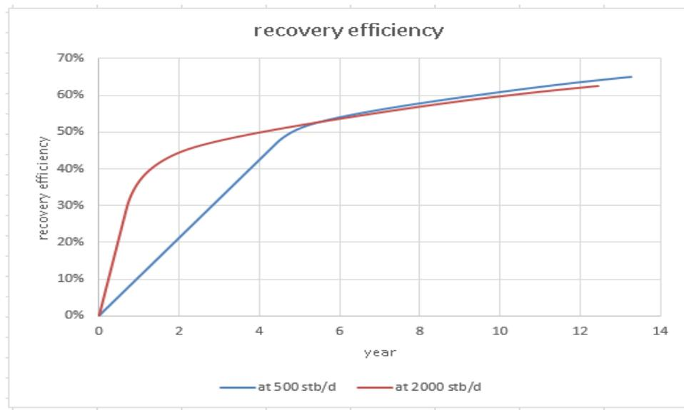
Figure 5.62 Field oil efficiency for horizontal well under gas reinjection at pressure lower than 2500 psi
