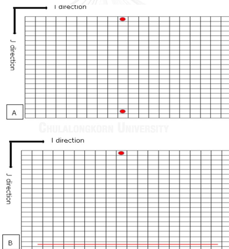
Figure 5.114 Top view for A) one vertical producer and one vertical injector and B) one horizontal producer and one vertical injector.
