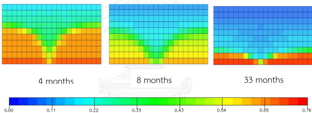
Figure A-2 Oil saturation versus time for grid plane  $j = 11$ : vertical production well under natural depletion at 1000 stb/d (xz plane view)
