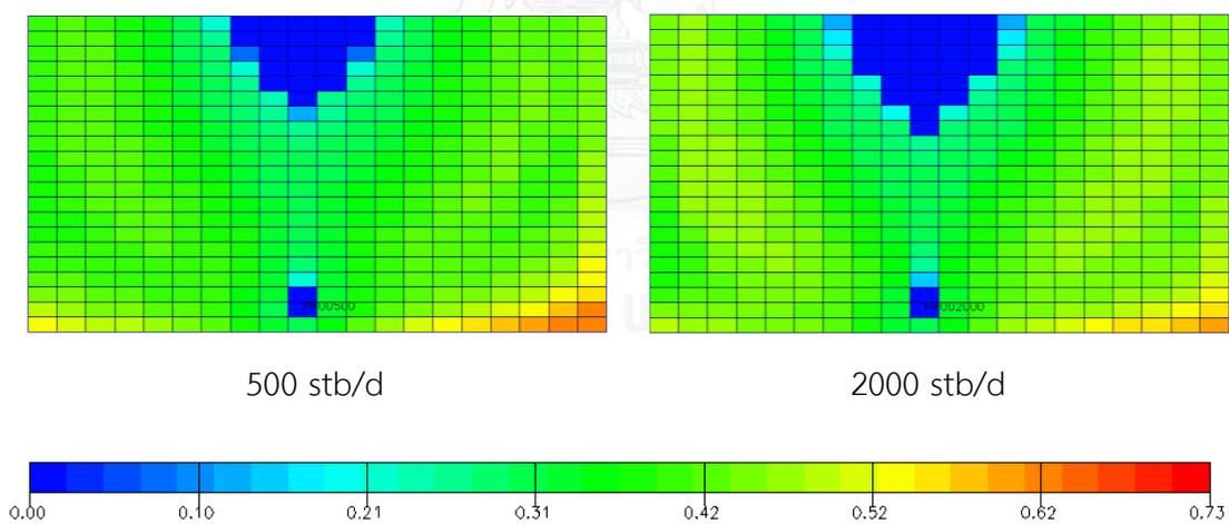
Figure 5.121 Oil saturation profile for grid plane k-10 at abandonment for vertical well at position 1 (xy plane view)
