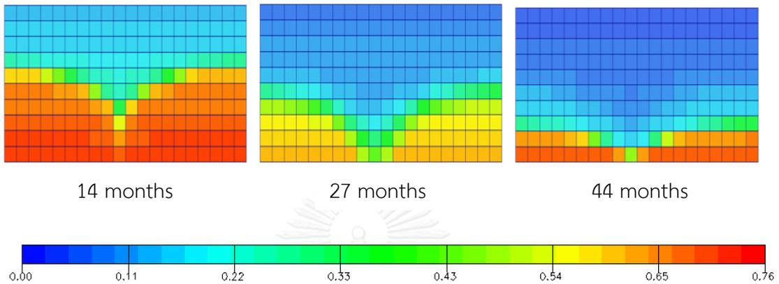
Figure 5.4 Oil saturation versus time for grid plane  $j = 11$ : vertical production well at 500 stb/d (xz plane view)
