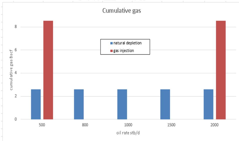
Figure 5.47 Cumulative gas produced by horizontal well under natural depletion and gas reinjection at different oil rates
