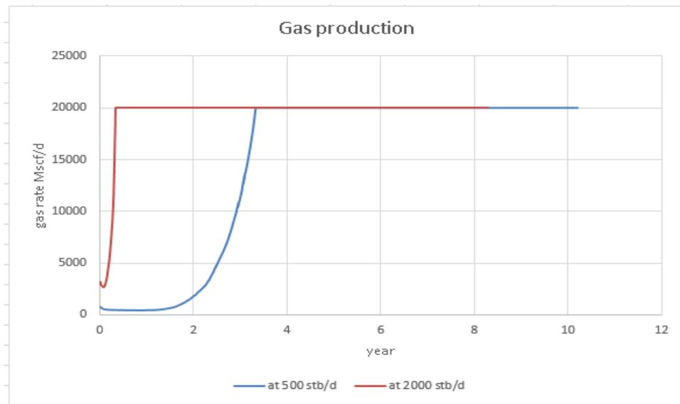
Figure 5.52 Gas production rate for vertical well under gas reinjection at pressure lower than 2500 psi
