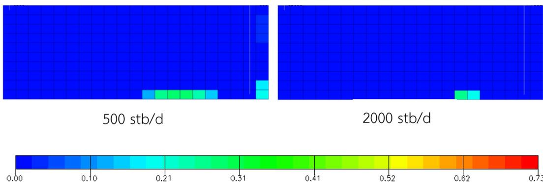
Figure A-45 Oil saturation at end of production for plane  $i = 10$ : gas injection scenario and horizontal production well in position 1 for different oil rates (yz plane view)
