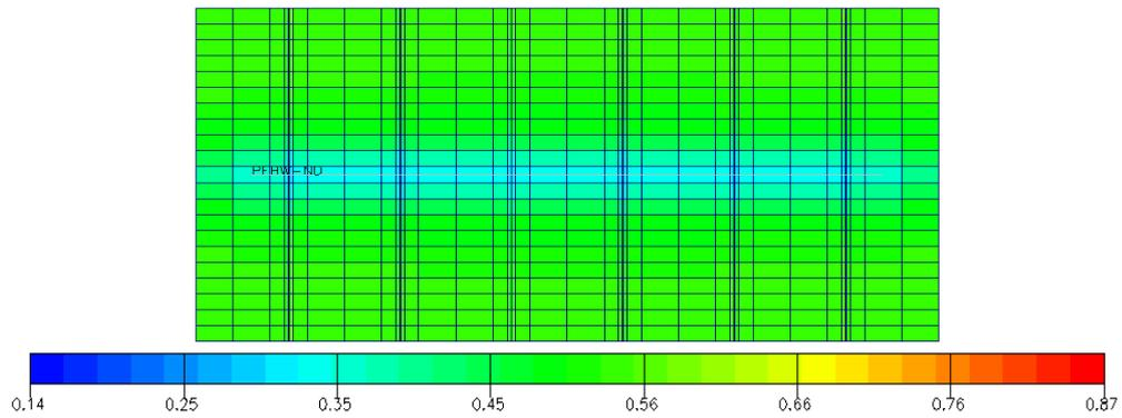
Figure 5.27 Oil saturation at abandonment for reservoir with a fractured horizontal well under natural depletion at 500 stb/d (xy plane view)
