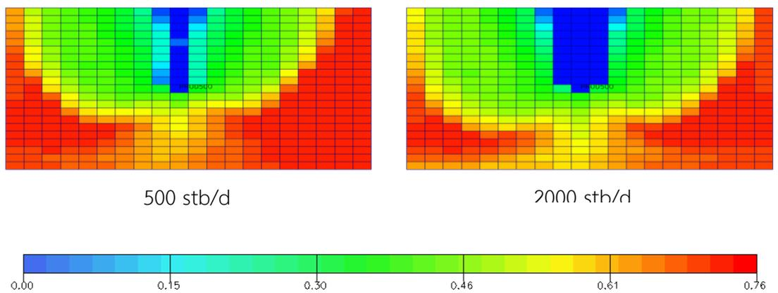
Figure 5.35 Oil saturation of plane  $k = 10$  at abandonment for vertical well under gas injection at different oil rates (xy plane view)
