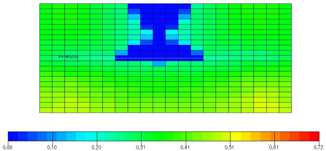
Figure 5.50 Oil saturation at abandonment for reservoir with a horizontal well under gas injection at 500 stb/d (xy plane view)
