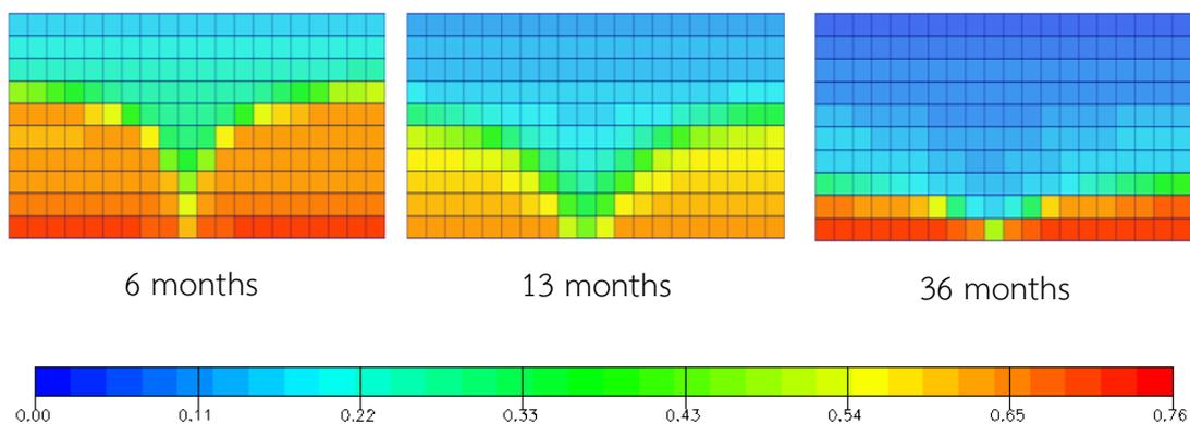
Figure A-1 Oil saturation versus time for grid plane  $j = 11$ : vertical production well under natural depletion at 800 stb/d (xz plane view)
