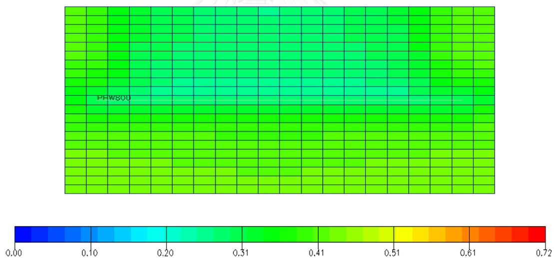
Figure 5.113 Oil saturation at abandonment for reservoir with a horizontal well under gas injection constrained at  $GOR < 160$  Mscf/stb at 500 stb/d (xy plane view)
