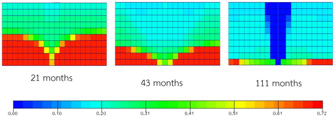
Figure 5.33 Oil saturation versus time for grid plane  $j = 11$  gas injection with vertical production well at 500 stb/d (xz plane view)
