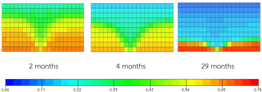
Figure A-3 Oil saturation versus time for grid plane  $j = 11$ : vertical production well under natural depletion at 1500 stb/d (xz plane view)
