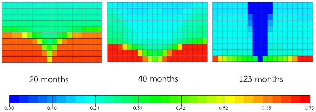
Figure 5.56 Oil saturation versus time for grid plane  $j = 11$ : gas injection when  $P < 2500$  psi with vertical production well at 500 stb/d (xz plane view)
