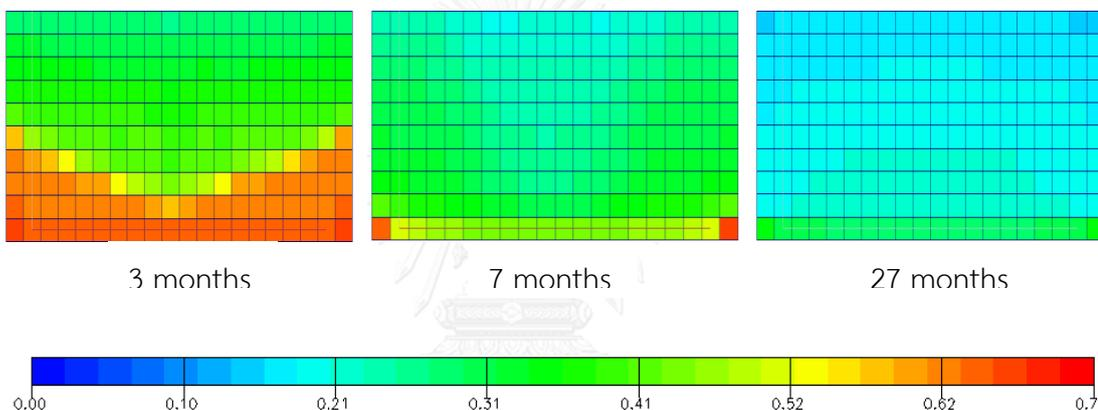
Figure A-31 Oil saturation versus time for grid plane  $j = 11$ : gas injection constrained at  $GOR < 80$  Mscf/stb and horizontal production well at 2000 stb/d (xz plane view)
