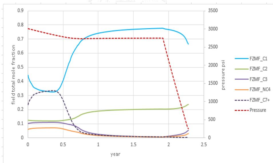
Figure B-14 Field total mole fraction and reservoir pressure vs time for the case of gas injection terminated when  $GOR > 80$  Mscf/stb using horizontal well at 2000 stb/d
