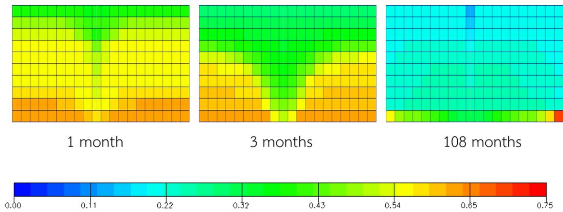
Figure 5.75 Oil saturation versus time for grid plane  $j = 11$ : gas injection when  $P < 1500$  psi with vertical production well at 2000 stb/d (xz plane view)
