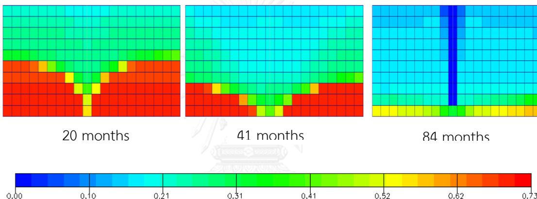
Figure A-34 Oil saturation versus time for grid plane  $j = 11$ : gas injection constrained at  $GOR < 160$  Mscf/stb and vertical production well at 500 stb/d (xz plane view)
