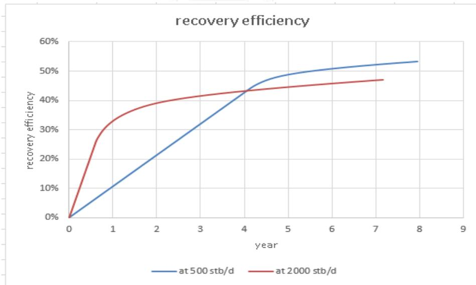
Figure 5.80 Field oil efficiency for horizontal well under gas reinjection at pressure lower than 1500 psi
