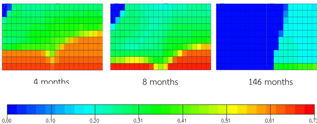
Figure A-17 Oil saturation versus time for grid plane  $i = 10$ : gas injection and horizontal production well at 2000 stb/d (yz plane view)
