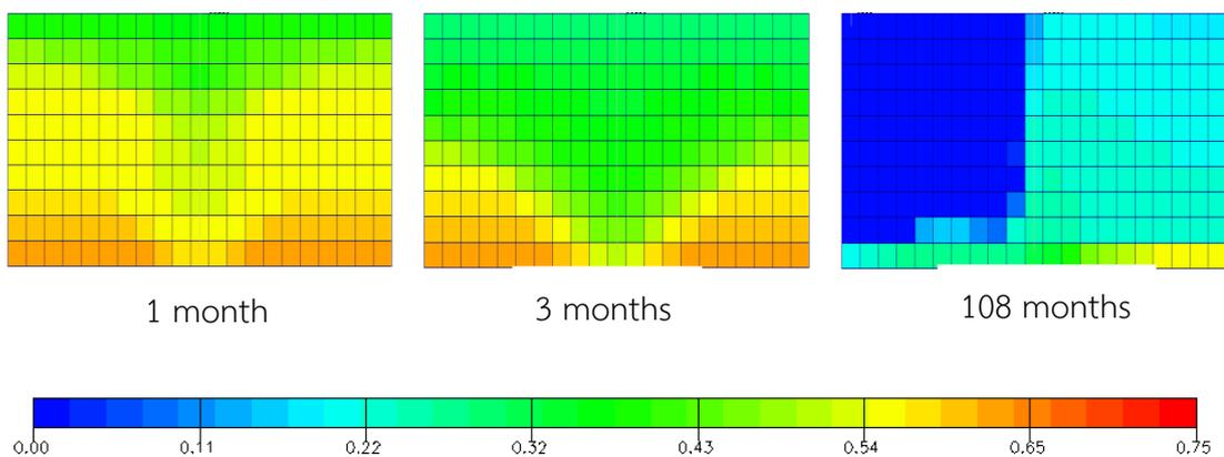
Figure A-23 Oil saturation versus time for grid plane  $i = 10$ : gas injection when  $P < 1500$  psi and vertical production well at 2000 stb/d (yz plane view)
