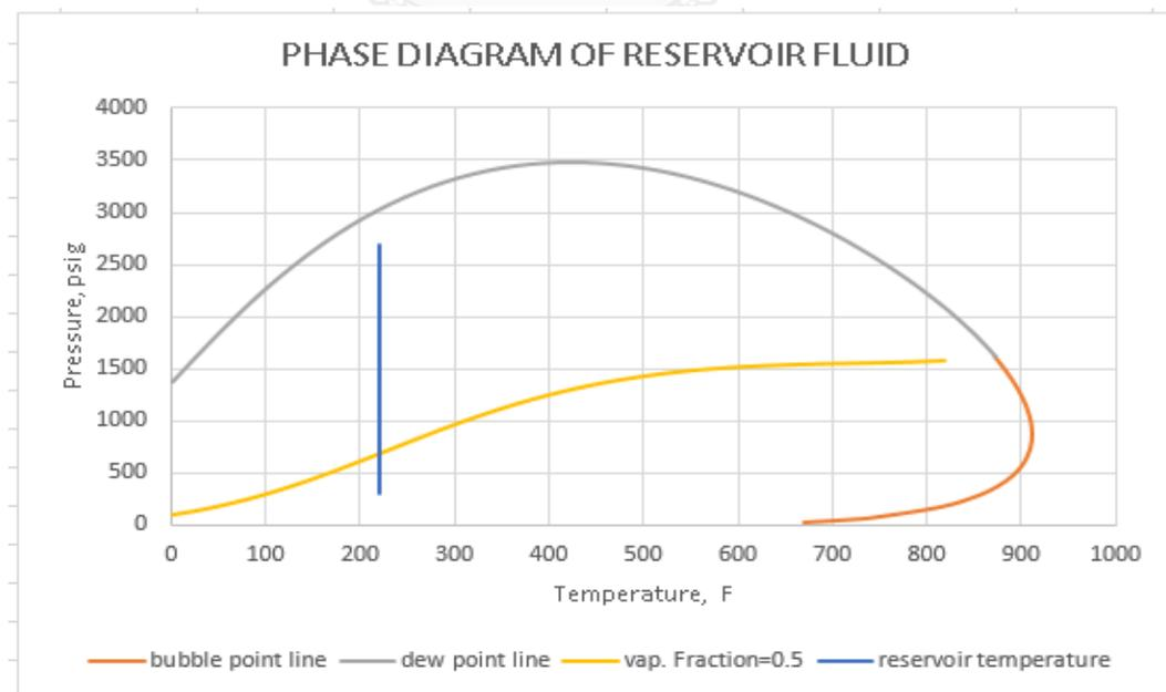
Figure 4.4 Phase diagram of the reservoir oil phase
