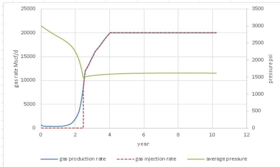
Figure 5.73 Trends of gas injection, gas production and average pressure for vertical well producer at 500 stb/d: gas injection when  $P < 1500$  psi scenario
