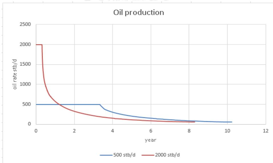
Figure 5.51 Oil production rate for vertical well under gas reinjection at pressure lower than 2500psi
