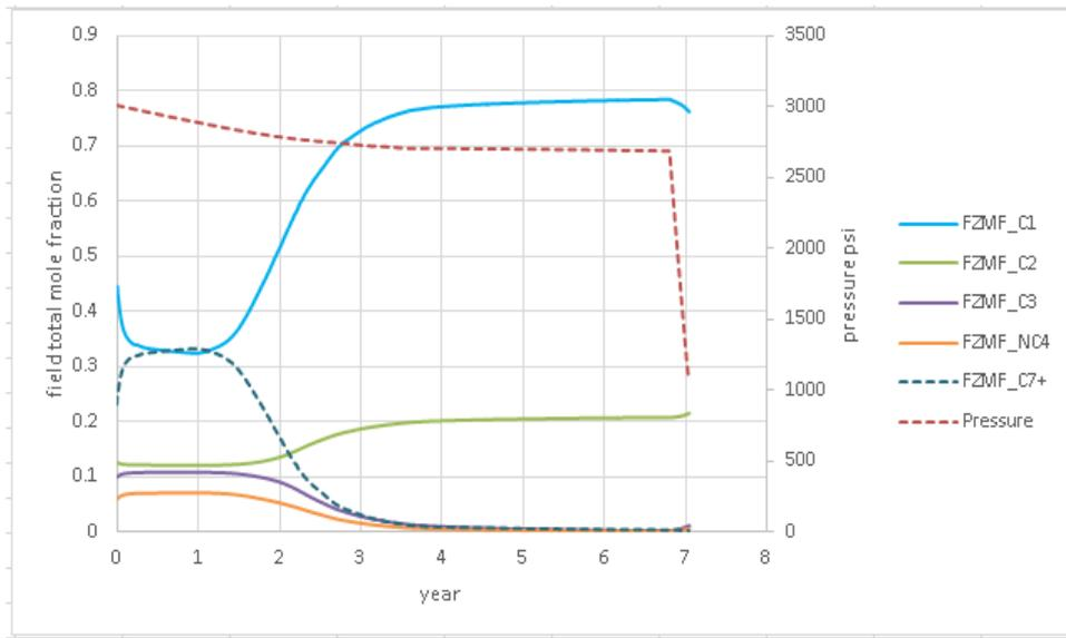
Figure B-15 Field total mole fraction and reservoir pressure vs time for the case of gas injection terminated when GOR>160 Mscf/stb using vertical well at 500 stb/d
