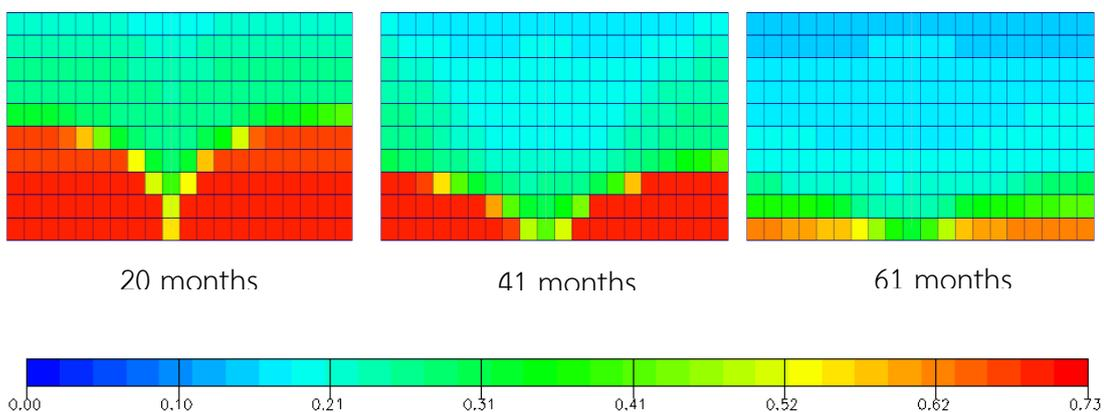
Figure A-26 Oil saturation versus time for grid plane  $j = 11$ : gas injection constrained at  $GOR < 80$  Mscf/stb and vertical production well at 500 stb/d (xz plane view)
