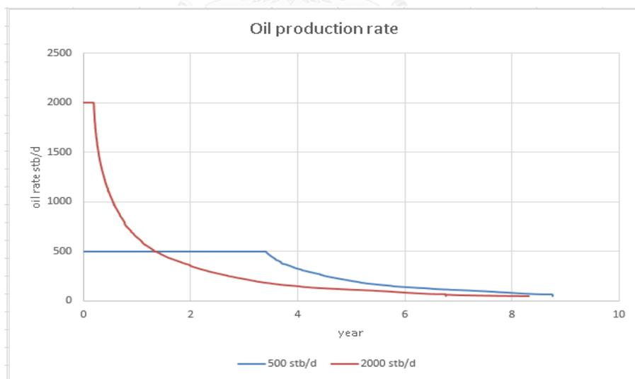
Figure 6.2 Oil production rate for vertical well at position 2 under produced gas reinjection
