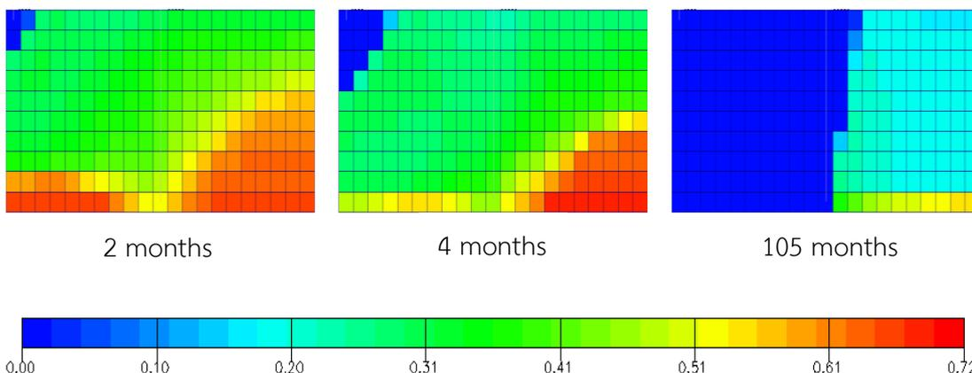
Figure A-15 Oil saturation versus time for grid plane  $i = 10$ : gas injection and vertical production well at 2000 stb/d (yz plane view)
