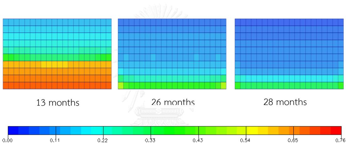
Figure A-5 Oil saturation versus time for grid plane  $j = 11$ : Horizontal production well under natural depletion at 800 stb/d (xz plane view)
