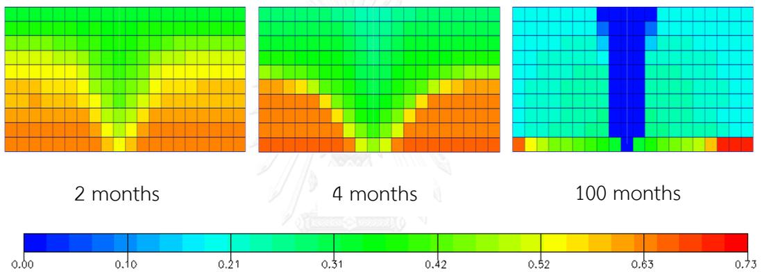
Figure 5.57 Oil saturation versus time for grid plane  $j = 11$ : gas injection when  $P < 2500$  psi with vertical production well at 2000 stb/d (xz plane view)
