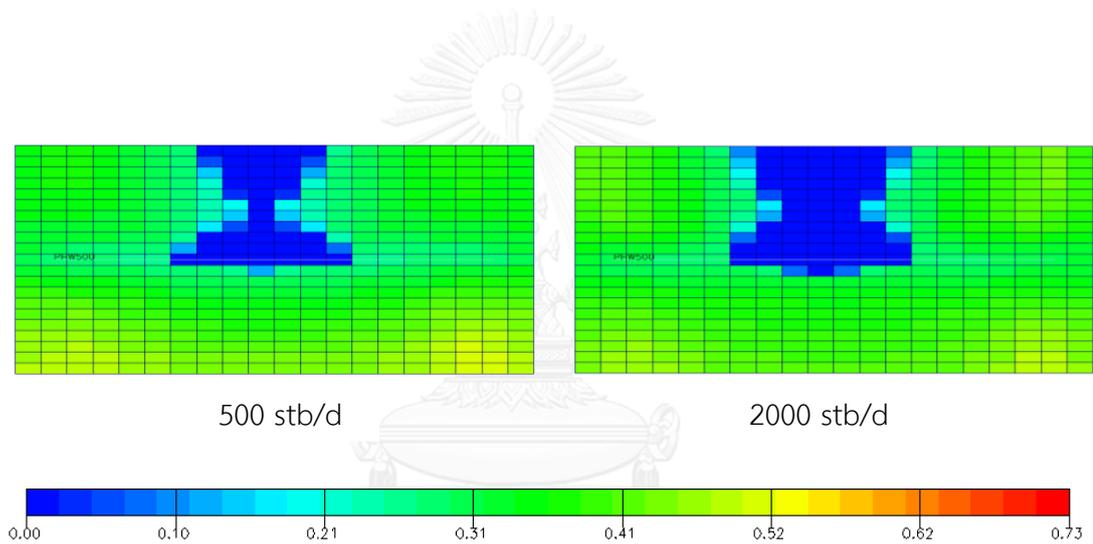
Figure 5.45 Oil saturation of plane  $k = 10$  at abandonment for horizontal well under gas injection at different oil rates (xy plane view)
