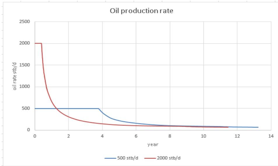
Figure 5.116 Oil production rate for vertical well at position 1 under produced gas reinjection
