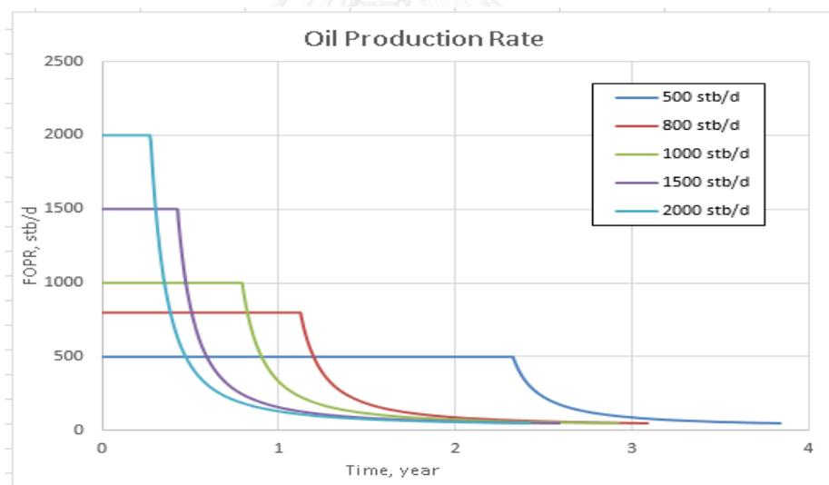
Figure 5.1 Oil production rates of vertical well under natural depletion.
