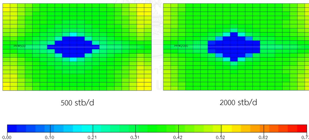
Figure 6.12 Oil saturation profile for grid plane k-10 at abandonment for horizontal well at position 2 (xy plane view)
