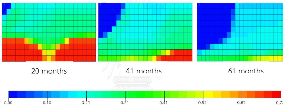
Figure A-28 Oil saturation versus time for grid plane  $i = 10$ : gas injection constrained at  $GOR < 80$  Mscf/stb and vertical production well at 500 stb/d (yz plane view)
