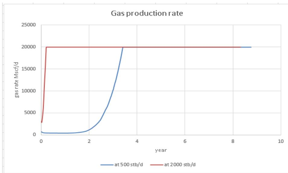
Figure 6.3 Gas production rate for vertical well at position 2 under produced gas reinjection
