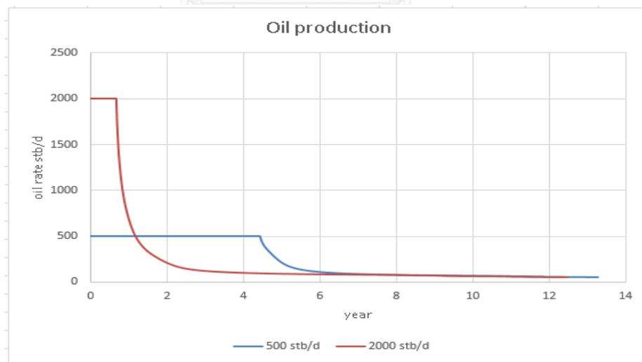
Figure 5.59 Oil production rate for horizontal well under gas reinjection at pressure lower than 2500 psi
