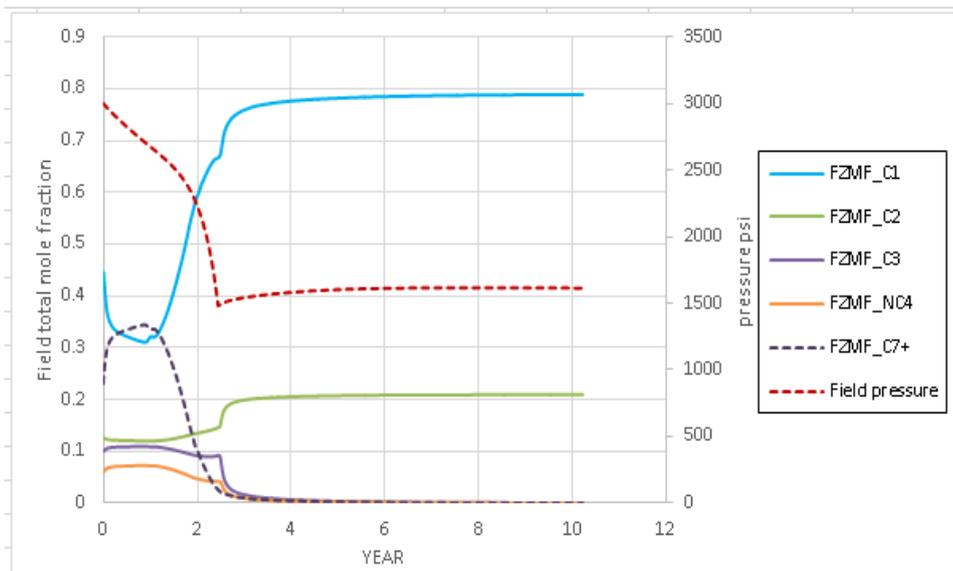
Figure B-7 Field total mole fraction and reservoir pressure vs time for the case of gas injection when pressure drops below 1500 psi using vertical well at 500 stb/d
