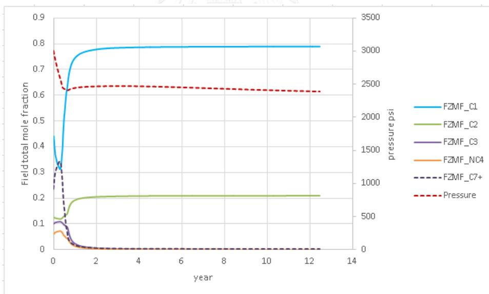
Figure B-6 Field total mole fraction and reservoir pressure vs time for the case of gas injection when pressure drops below 2500 psi using horizontal well at 2000 stb/d
