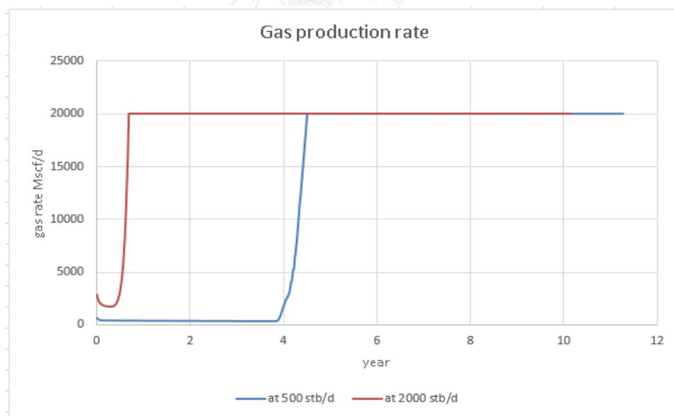
Figure 6.8 Gas production rate for horizontal well at position 2 under produced gas reinjection
