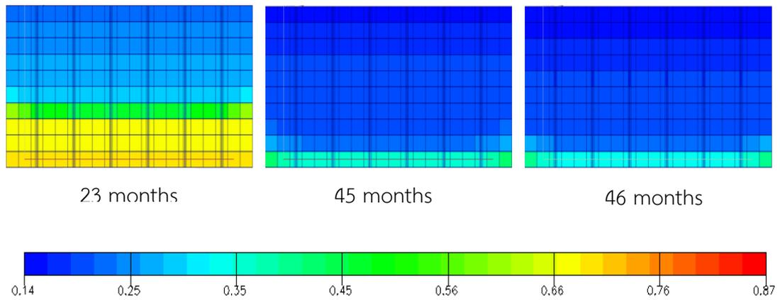
Figure 5.17 Oil saturation versus time for grid plane  $j = 11$ : Fracture horizontal production well at 500 stb/d ( $xz$  plane view)
