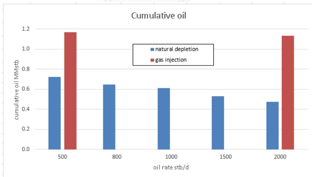
Figure 5.46 Cumulative oil produced by horizontal well under natural depletion and gas reinjection at different oil rates
