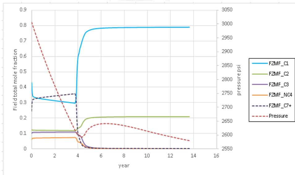
Figure B-2 Field total mole fraction and reservoir pressure vs time for the case of gas injection from the start of production using horizontal well at 500 stb/d
