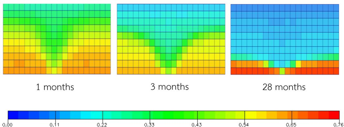
Figure A-4 Oil saturation versus time for grid plane  $j = 11$ : vertical production well under natural depletion at 2000 stb/d (xz plane view)
