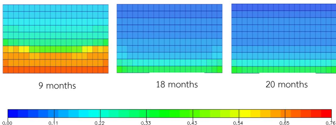
Figure A-6 Oil saturation versus time for grid plane  $j = 11$ : Horizontal production well under natural depletion at 1000 stb/d (xz plane view)
