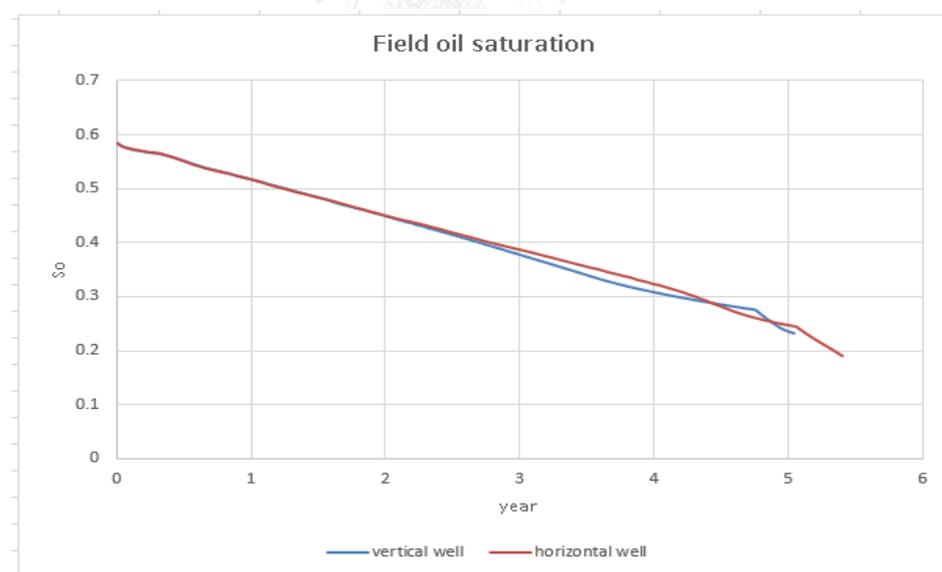
Figure 5.98 Average field oil saturation versus time for reservoir under gas injection constrained at  $GOR < 80$  Mscf/stb using different well types
