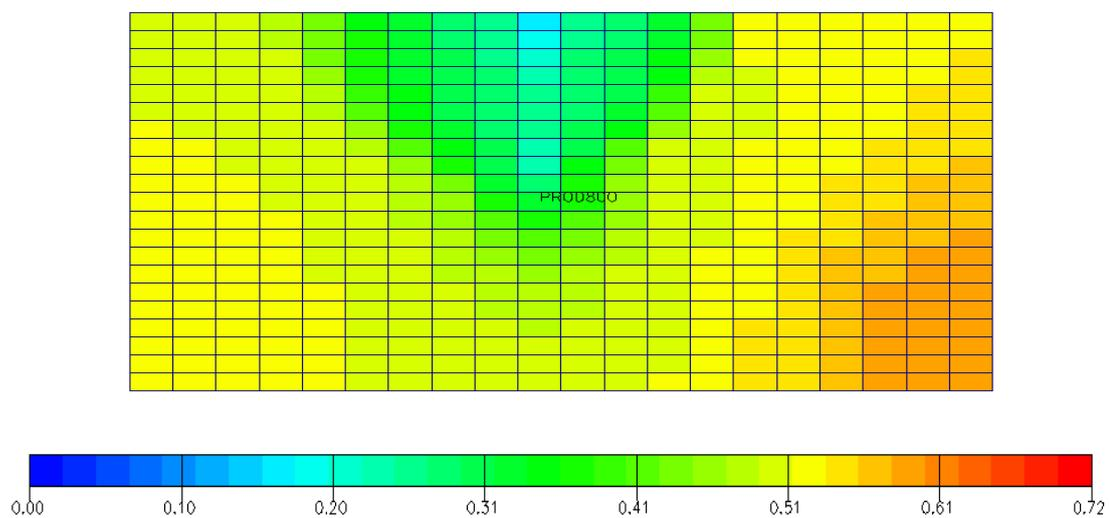
Figure 5.112 Oil saturation at abandonment for reservoir with a vertical well under gas injection constrained at  $GOR < 160$  Mscf/stb at 500 stb/d (xy plane view)
