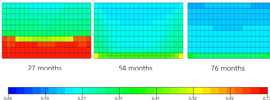
Figure A-38 Oil saturation versus time for grid plane  $j = 11$ : gas injection constrained at  $GOR < 160$  Mscf/stb and horizontal production well at 500 stb/d (xz plane view)
