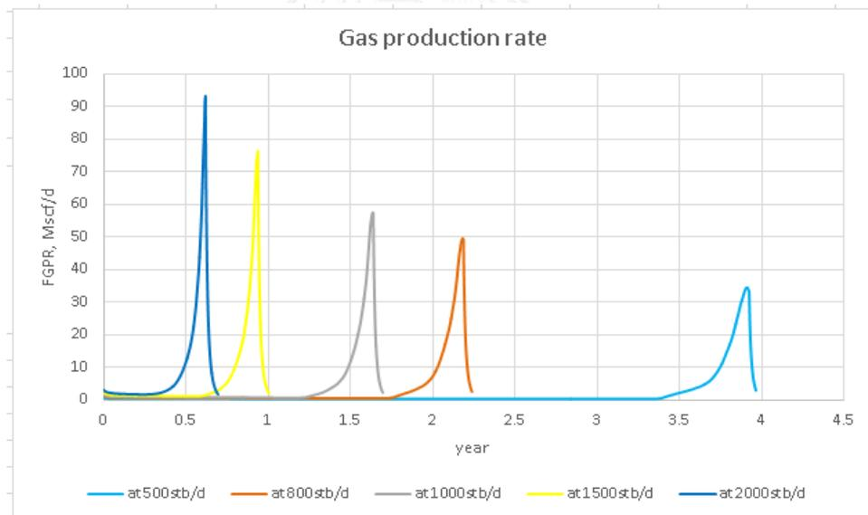
Figure 5.14 Gas production rate of fractured horizontal well under natural depletion at different oil rates
