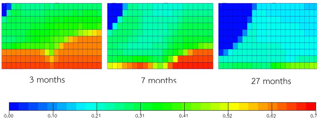
Figure A-33 Oil saturation versus time for grid plane  $i = 10$ : gas injection constrained at  $GOR < 80$  Mscf/stb and horizontal production well at 2000 stb/d (yz plane view)
