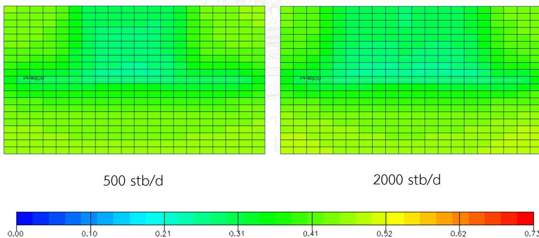
Figure 5.97 Oil saturation of plane  $k = 10$  at abandonment for horizontal well under gas injection constrained at GOR<80 Mscf/stb at different oil rates (xy plane view)
