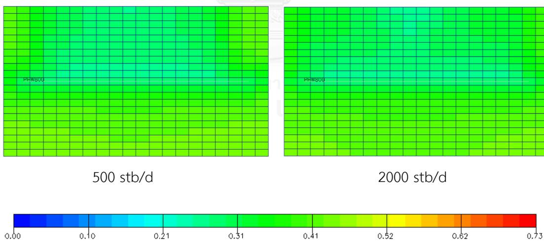
Figure 5.110 Oil saturation of plane  $k = 10$  at abandonment for horizontal well under gas injection constrained at  $GOR < 160$  Mscf/stb at different oil rates (xy plane view)
