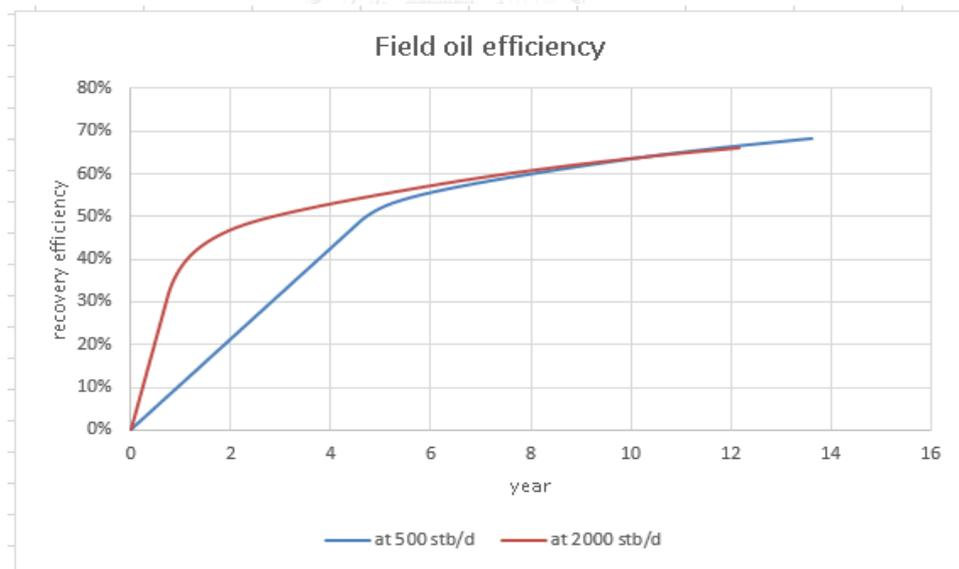
Figure 5.41 Field oil recovery efficiency for horizontal well under gas reinjection at different oil rates
