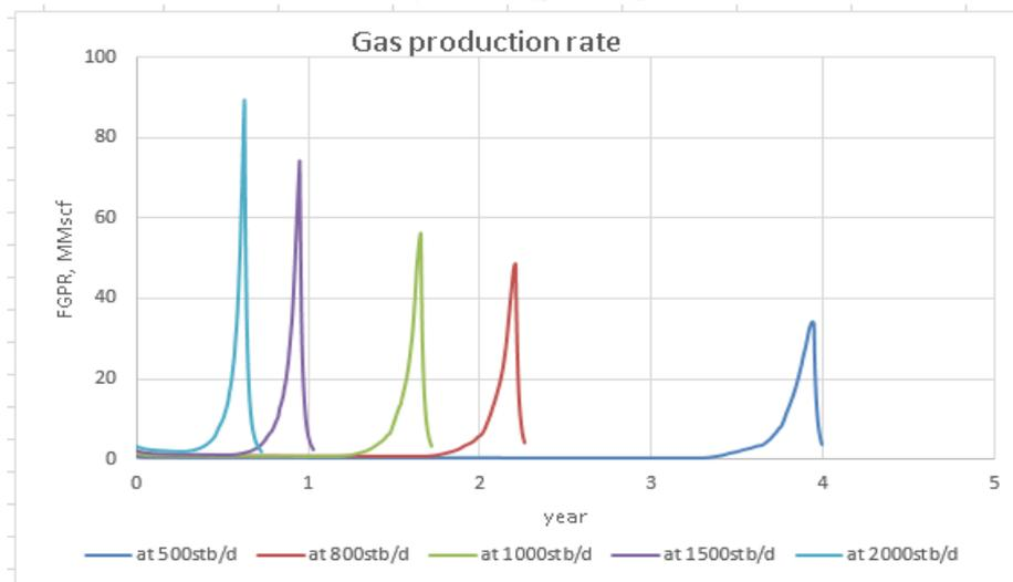
Figure 5.7 Gas production rate of horizontal well under natural depletion at different oil rates
