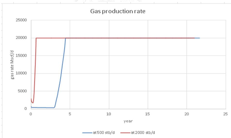
Figure 5.123 Gas production rate for horizontal well at position 1 under produced gas reinjection
