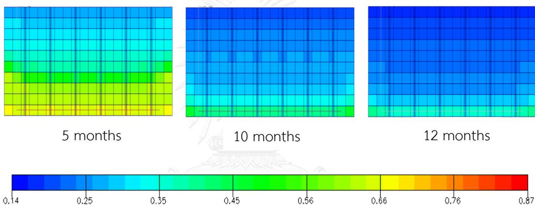
Figure A-11 Oil saturation versus time for grid plane  $j = 11$ : Fracture horizontal production well under natural depletion at 1500 stb/d (xz plane view)
