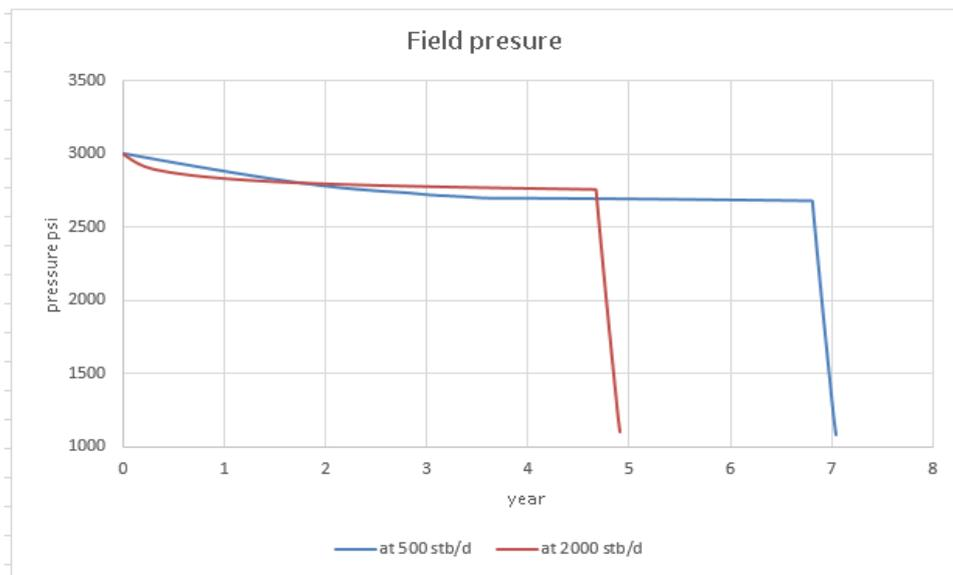
Figure 5.101 Field pressure for vertical wells: production constrained at GOR<160 Mscf/stb
