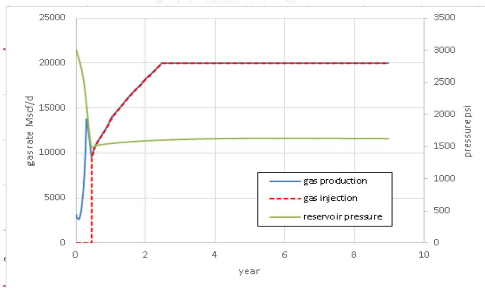
Figure 5.70 Trends of gas injection, gas production and average pressure for vertical well producer at 2000 stb/d: gas injection when  $P < 1500$  psi scenario
