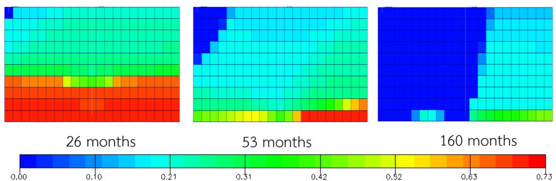
Figure A-20 Oil saturation versus time for grid plane  $i = 10$ : gas injection when  $P < 2500$  psi and horizontal production well at 500 stb/d (yz plane view)
