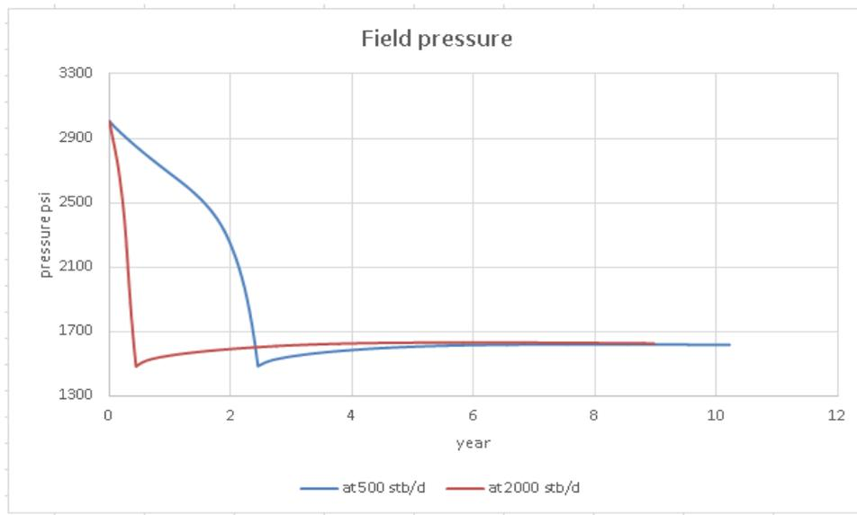
Figure 5.71 Field pressure for vertical wells under gas reinjection at pressure lower than 1500 psi
