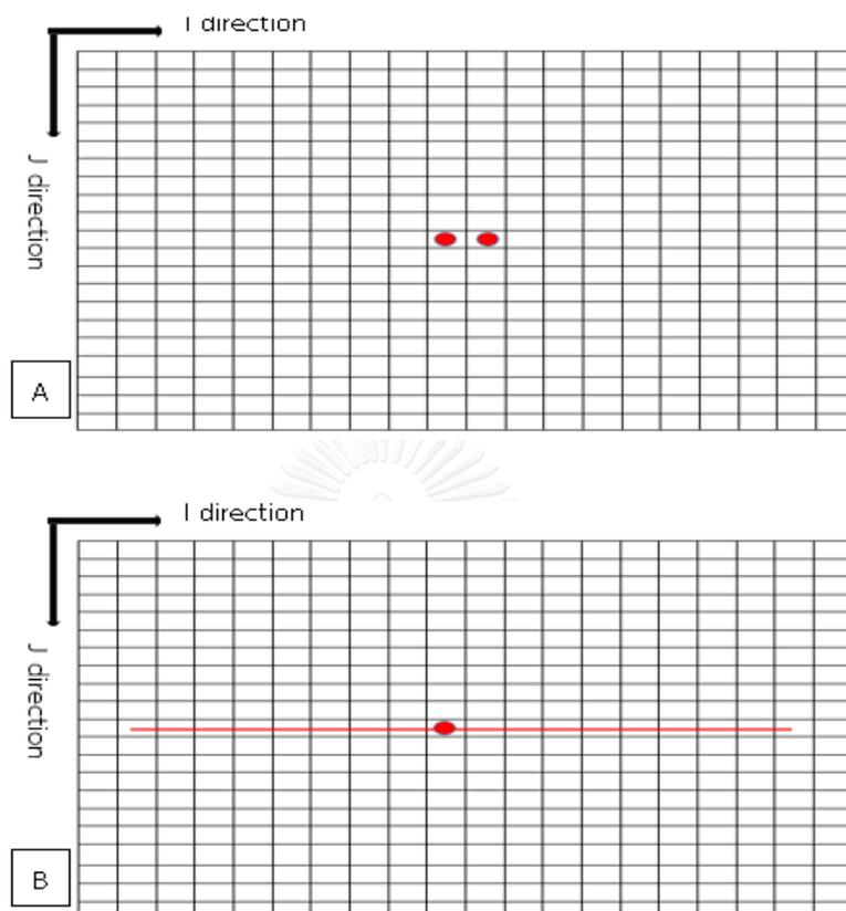
Figure 5.115 Top view for A) one vertical producer and one vertical injector and B) one horizontal producer and one vertical injector.
