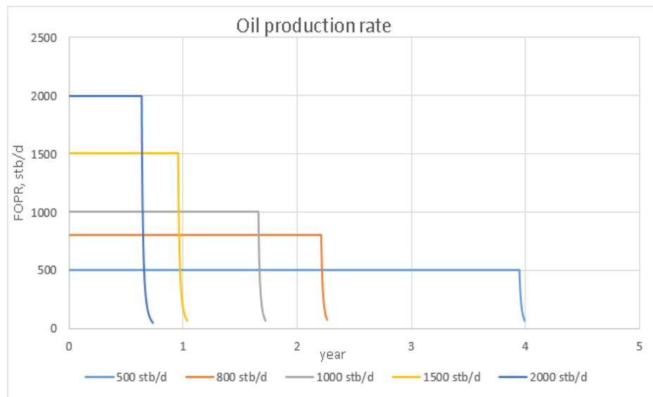
Figure 5.6 Oil production rate of horizontal well under natural depletion
