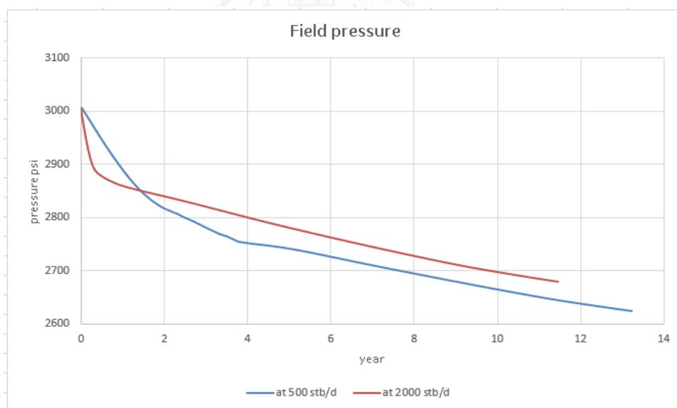
Figure 5.119 Field pressure for vertical well at position 1 under produced gas reinjection
