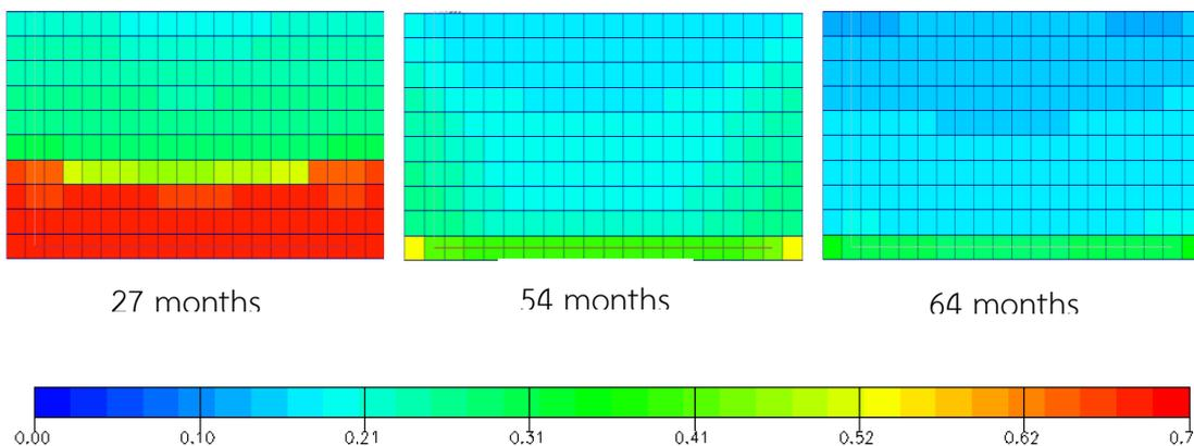
Figure A-30 Oil saturation versus time for grid plane  $j = 11$ : gas injection constrained at  $GOR < 80$  Mscf/stb and horizontal production well at 500 stb/d (xz plane view)
