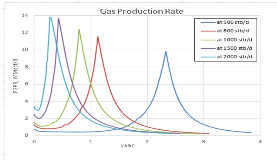
Figure 5.2 Gas production rate of vertical well under natural depletion at different oil rates.
