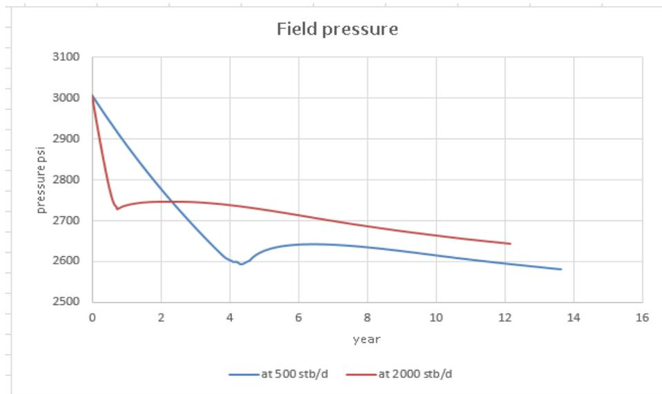
Figure 5.40 Field pressure for horizontal well under gas reinjection at different oil rates
