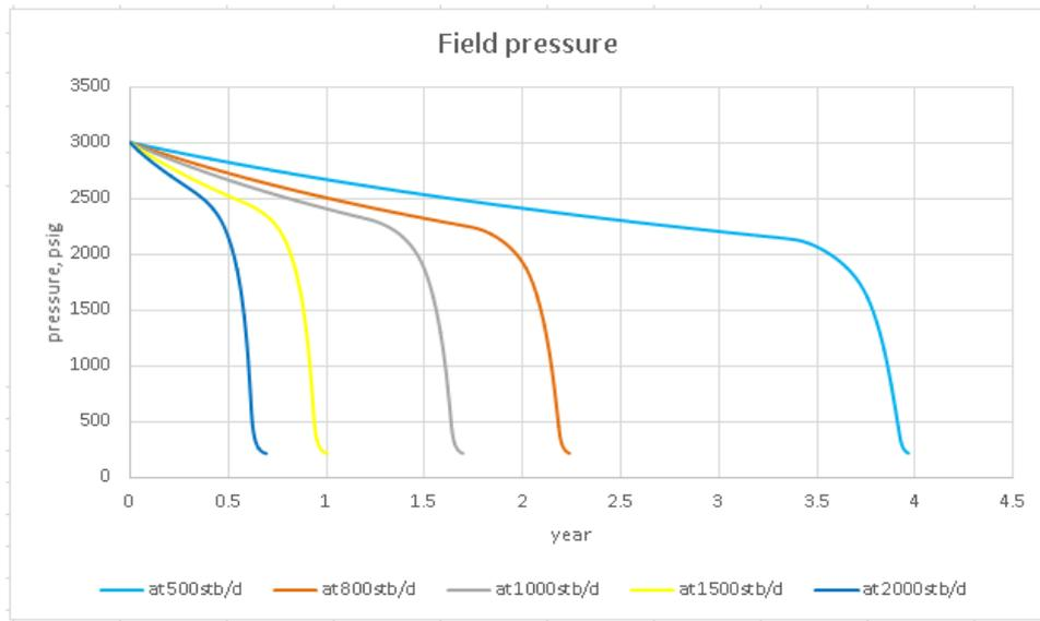
Figure 5.15 Field pressure of fractured horizontal well under natural depletion at different oil rates
