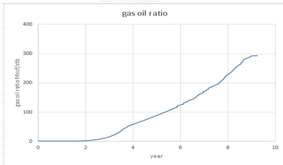
Figure 5.85 Gas-oil ratio for gas injection case with vertical well producing at 500 stb/d
