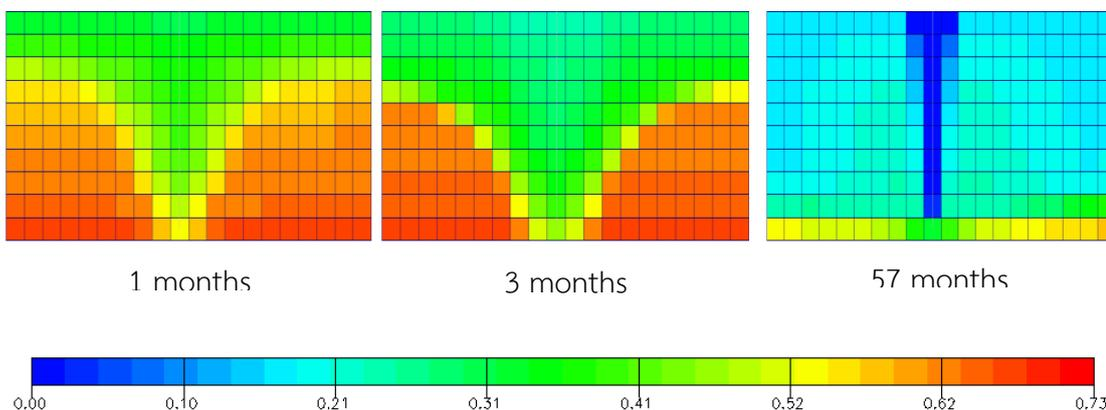
Figure A-35 Oil saturation versus time for grid plane  $j = 11$ : gas injection constrained at  $GOR < 160$  Mscf/stb and vertical production well at 2000 stb/d (xz plane view)
