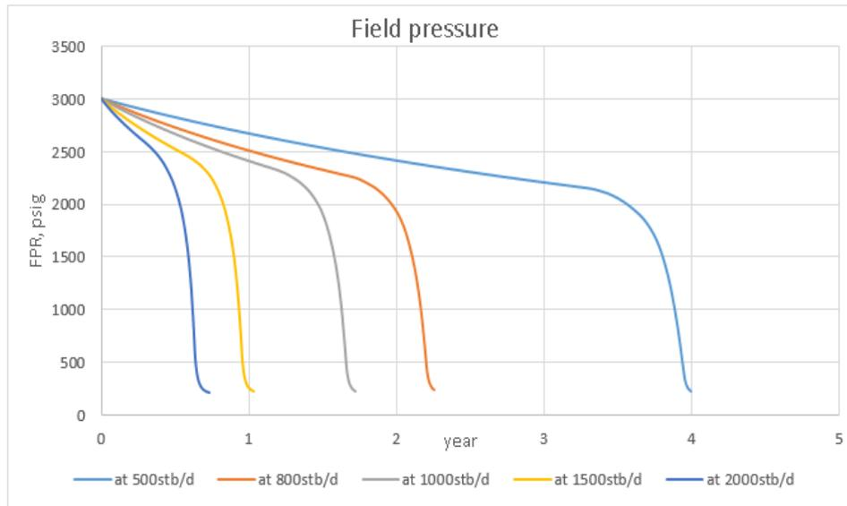
Figure 5.8 Field pressure of horizontal well under natural depletion at different oil rates
