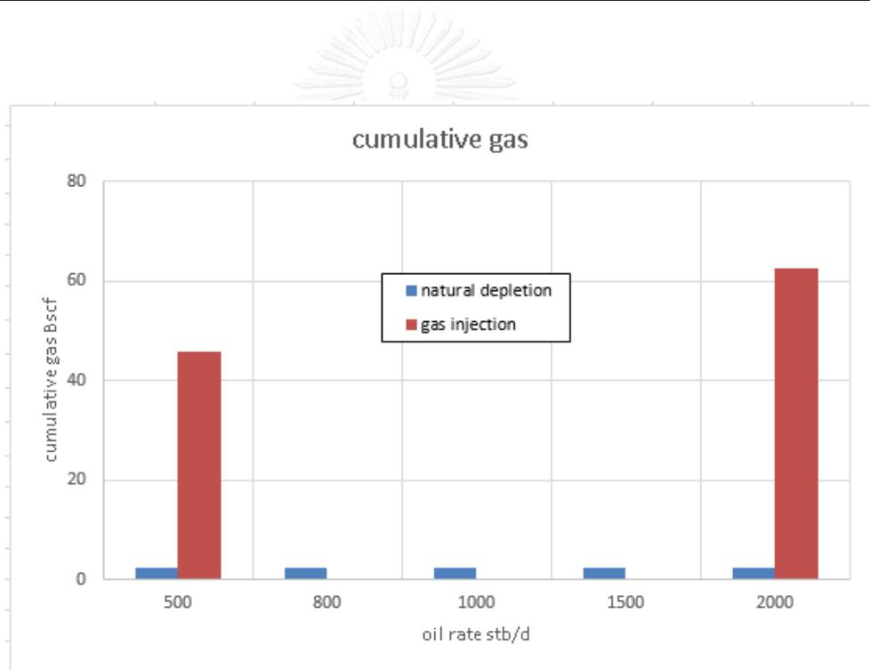
Figure 5.37 Cumulative gas for vertical well under natural depletion and gas injection
