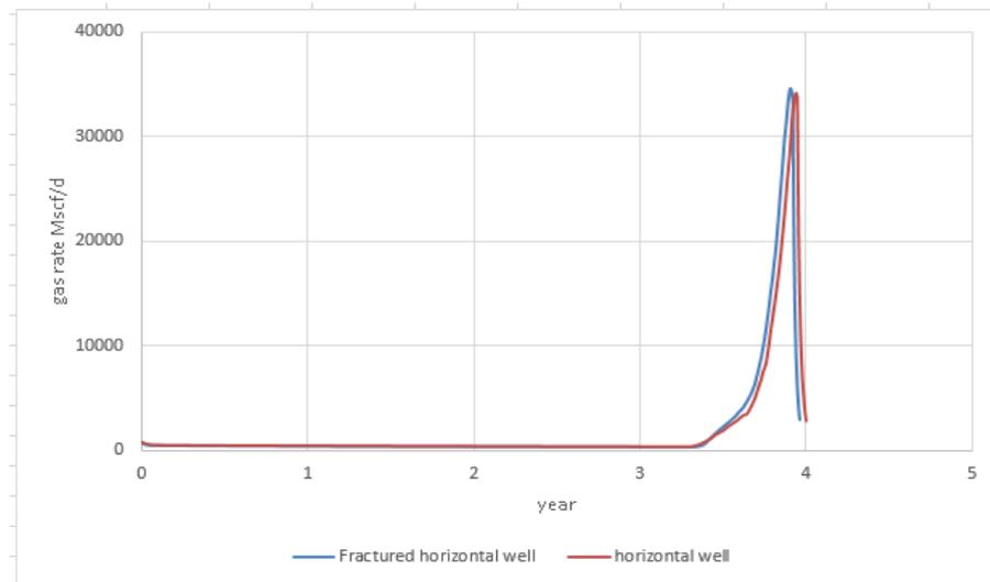
Figure 5.20 Comparison of gas rate for fractured horizontal well and horizontal well at 500 stb/d
