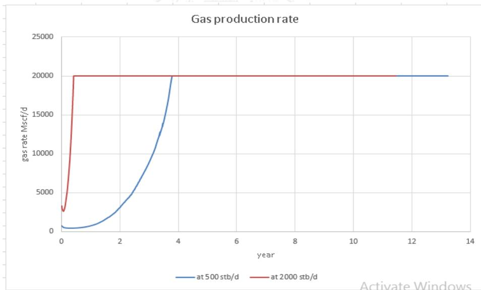
Figure 5.117 Gas production rate for vertical well at position 1 under produced gas reinjection
