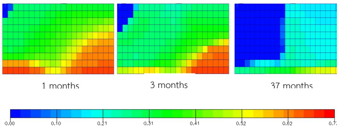
Figure A-29 Oil saturation versus time for grid plane  $i = 10$ : gas injection constrained at  $GOR < 80$  Mscf/stb and vertical production well at 2000 stb/d (yz plane view)
