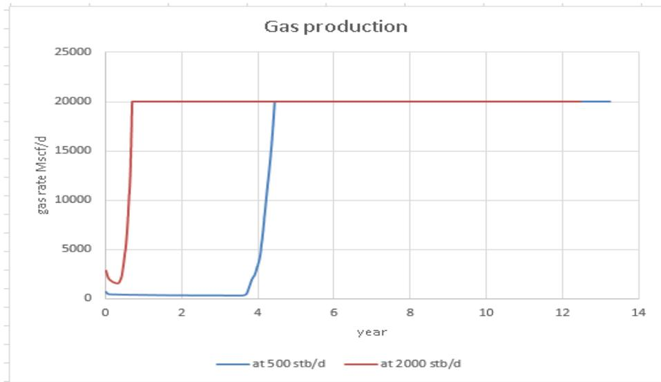
Figure 5.60 Gas production rate for horizontal well under gas reinjection at pressure lower than 2500 psi
