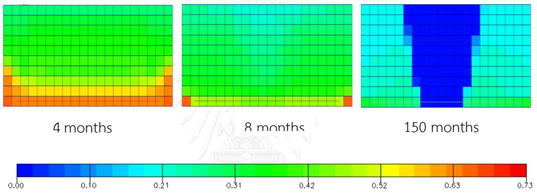
Figure 5.65 Oil saturation versus time for grid plane  $j = 11$ : gas injection when  $P < 2500$  psi with horizontal production well at 2000 stb/d (xz plane view)
