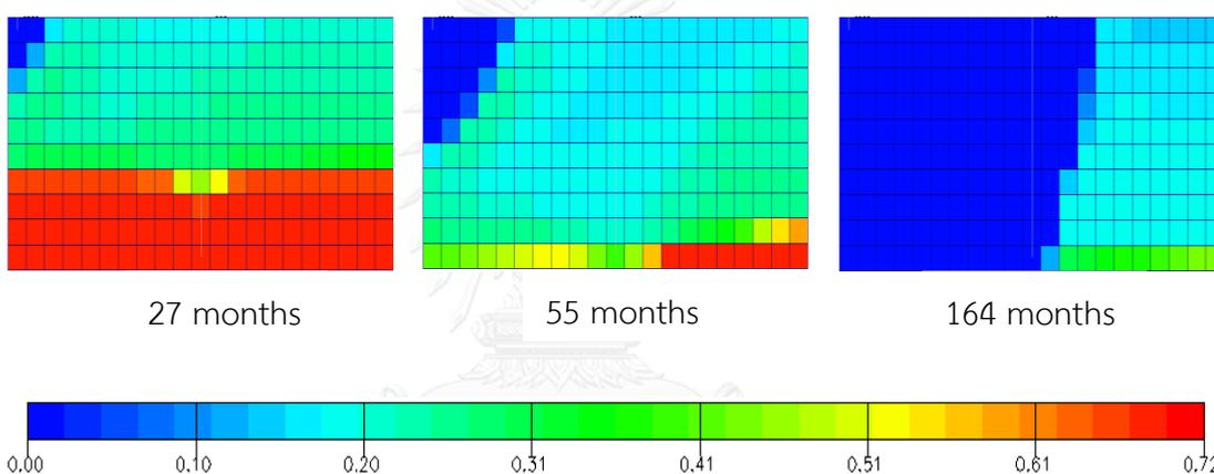
Figure A-16 Oil saturation versus time for grid plane  $i = 10$ : gas injection and horizontal production well at 500 stb/d (yz plane view)
