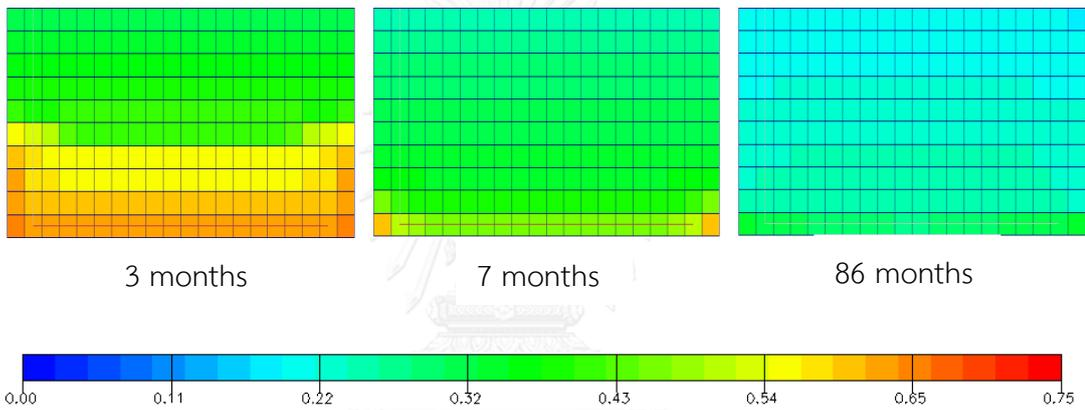
Figure 5.82 Oil saturation versus time for grid plane  $j = 11$ : gas injection when  $P < 1500$  psi with horizontal production well at 2000 stb/d (xz plane view)
