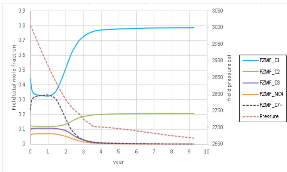
Figure B-1 Field total mole fraction and reservoir pressure vs time for the case of gas injection from the start of production using vertical well at 500 stb/d
