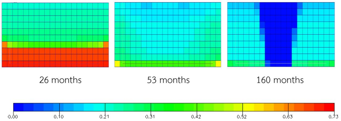
Figure 5.64 Oil saturation versus time for grid plane  $j = 11$ : gas injection when  $P < 2500$  psi with horizontal production well at 500 stb/d (xz plane view)
