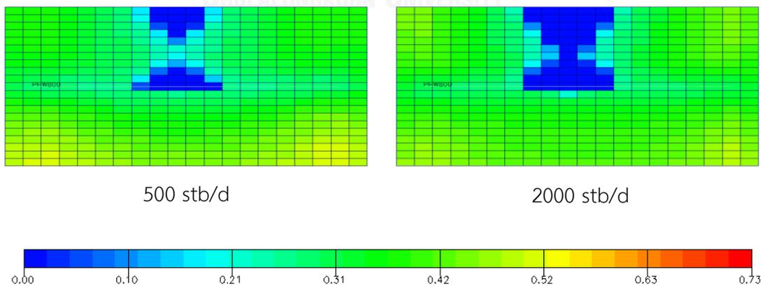
Figure 5.66 Oil saturation of plane  $k = 10$  at abandonment for horizontal well under gas injection when  $P < 2500$  psi at different oil rates (xy plane view)
