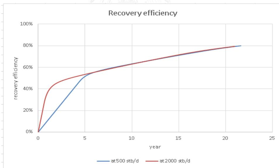
Figure 5.125 Field oil efficiency for horizontal well at position 1 under produced gas reinjection
