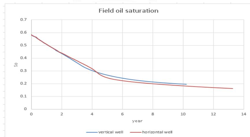
Figure 5.67 Average field oil saturation versus time for reservoir under gas injection when  $P < 2500$  psi using different well types
