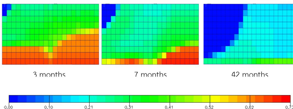
Figure A-41 Oil saturation versus time for grid plane  $i = 10$ : gas injection constrained at  $\text{GOR} < 160$  Mscf/stb and horizontal production well at 2000 stb/d (yz plane view)
