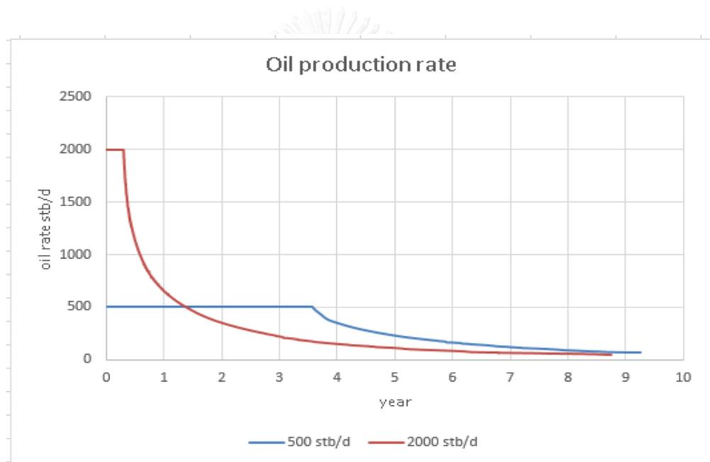
Figure 5.28 Oil production rate for vertical well under gas reinjection
