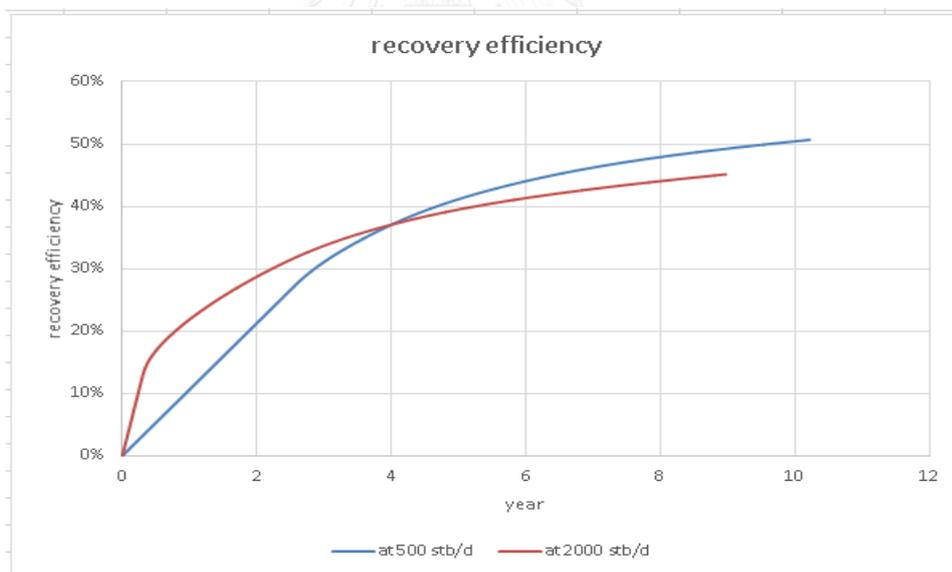
Figure 5.72 Field oil efficiency for vertical wells under gas reinjection at pressure lower than 1500 psi
