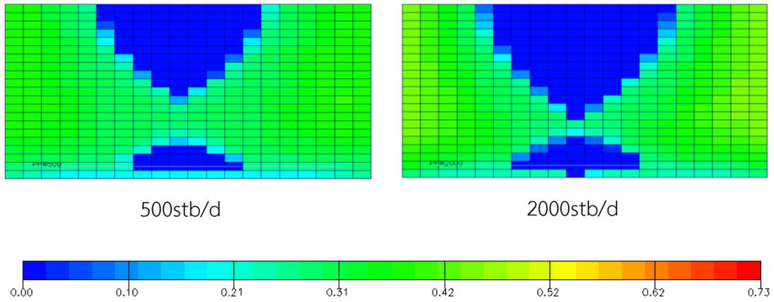
Figure 5.126 Oil saturation profile for grid plane k-10 at abandonment for horizontal well at position 1 (xy plane view)
