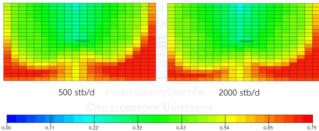
Figure 5.76 Oil saturation of plane  $k = 10$  at abandonment for vertical well under gas injection when  $P < 1500$  psi at different oil rates (xy plane view)
