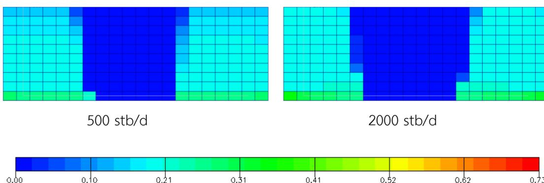
Figure A-44 Oil saturation at end of production for plane  $j = 20$ : gas injection scenario and horizontal production well in position 1 for different oil rates (xz plane view)
