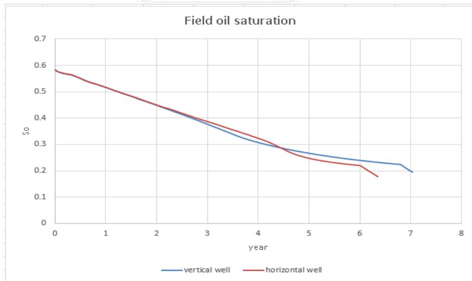
Figure 5.111 Average field oil saturation versus time for reservoir under gas injection constrained at  $GOR < 160$  Mscf/stb using different well types
