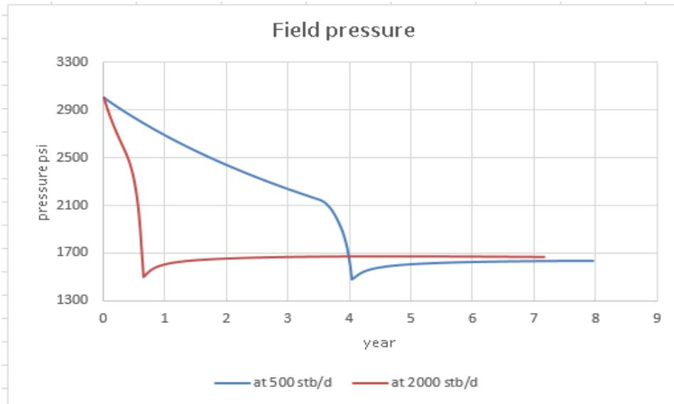
Figure 5.79 Field pressure for horizontal well under gas reinjection at pressure lower than 1500 psi
