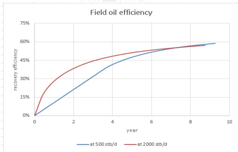
Figure 5.32 Field oil recovery efficiency for vertical well under gas reinjection at different oil flow rates
