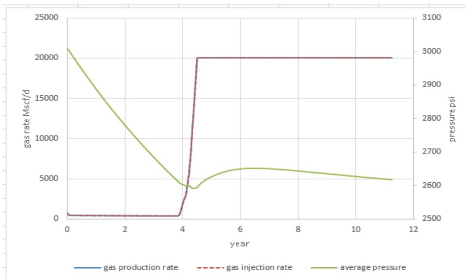
Figure 6.11 Trends of gas injection, gas production and average pressure for horizontal well producer at 500 stb/d: production well on position 2
