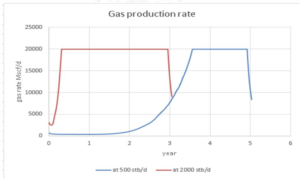
Figure 5.87 Gas production rate for vertical wells: production constrained at GOR<80
