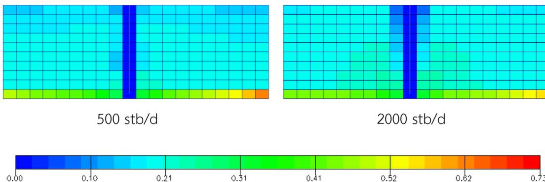
Figure A-42 Oil saturation at end of production for plane  $j = 20$ : gas injection scenario and vertical production well in position 1 for different oil rates (xz plane view)
