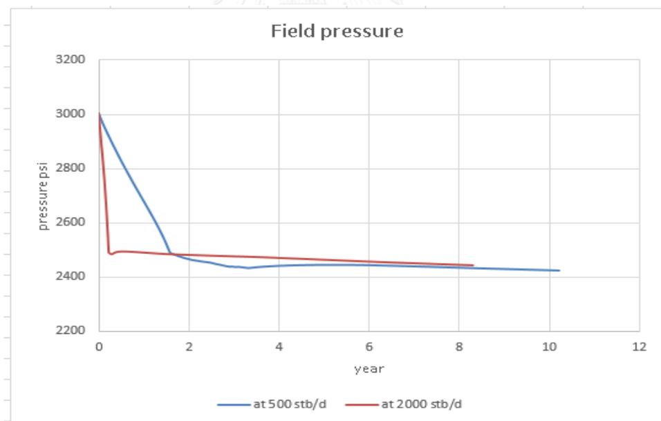
Figure 5.53 Field pressure for vertical well under gas reinjection at pressure lower than 2500 psi
