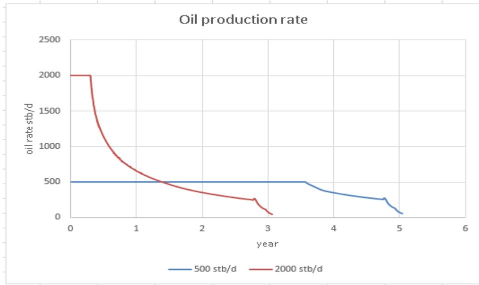
Figure 5.86 Oil production rate for vertical wells: production constrained at GOR<80
