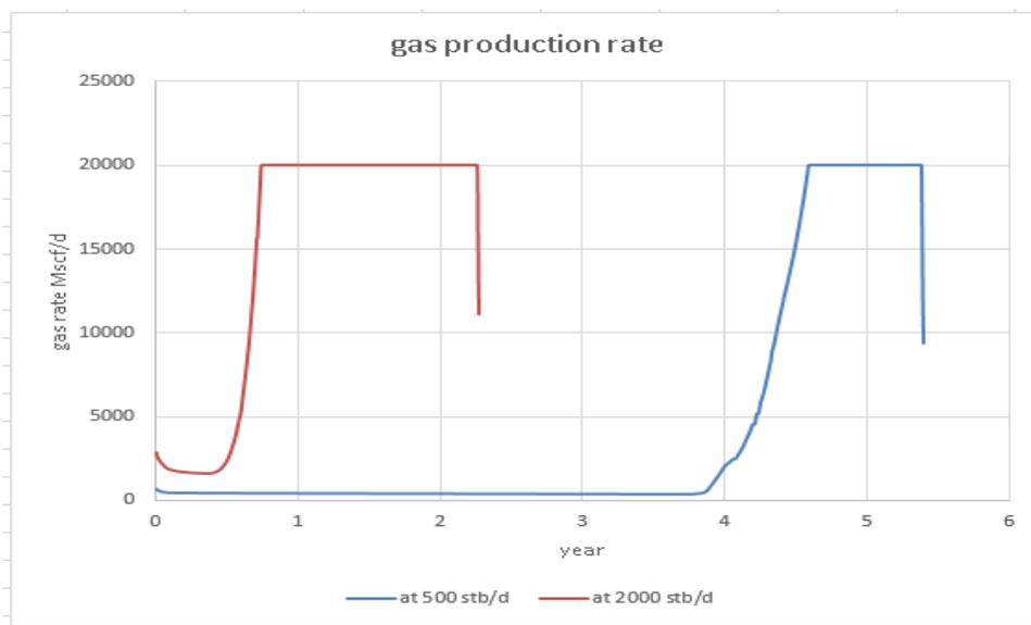
Figure 5.94 Gas production rate for horizontal wells for production constrained at GOR < 80 Mscf/stb
