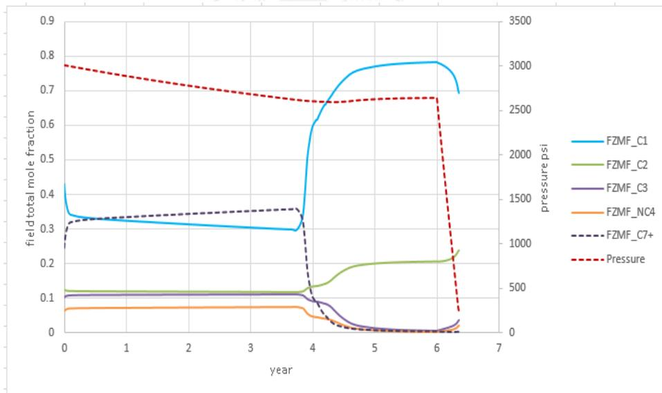
Figure B-16 Field total mole fraction and reservoir pressure vs time for the case of gas injection terminated when GOR>160 Mscf/stb using horizontal well at 500 stb/d
