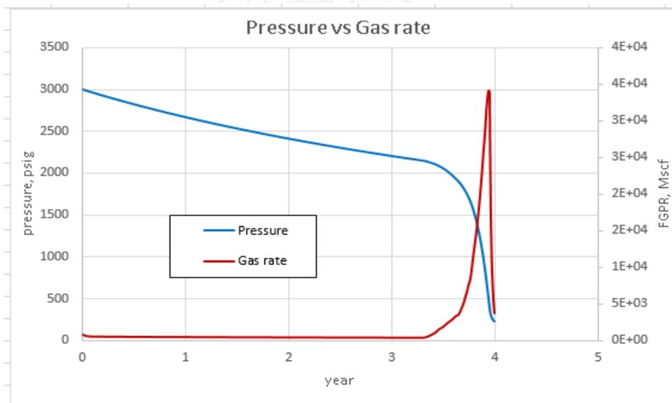
Figure 5.11 Field pressure profile, and gas rate profile of horizontal well producing at 500 stb/d
