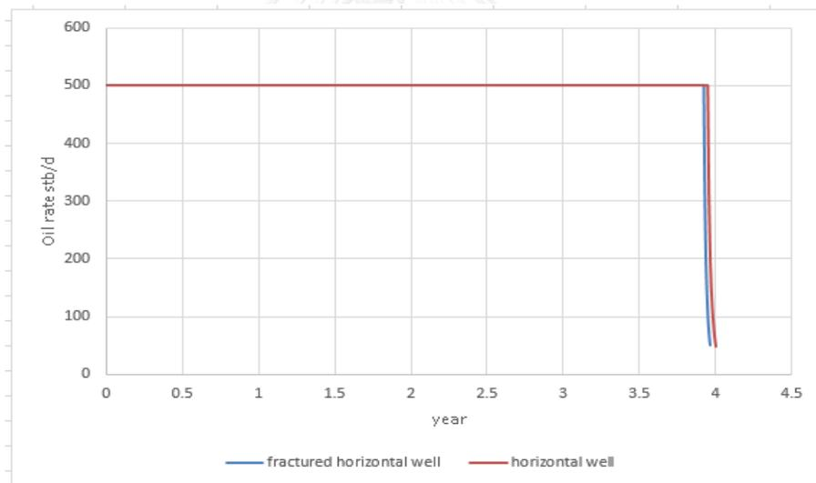
Figure 5.19 Comparison of oil rate for fractured horizontal well and horizontal well at 500 stb/d
