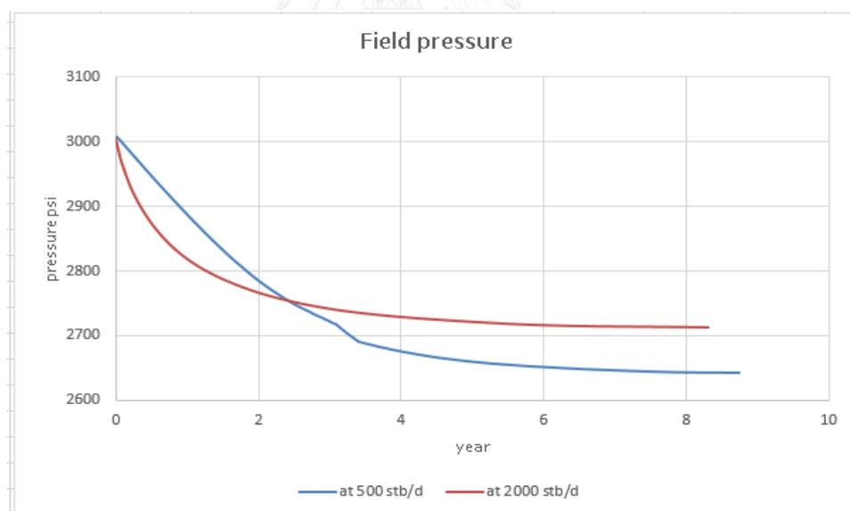
Figure 6.4 Field pressure for vertical well at position 2 under produced gas reinjection
