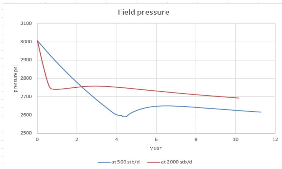
Figure 6.9 Field pressure for horizontal well at position 2 under produced gas reinjection
