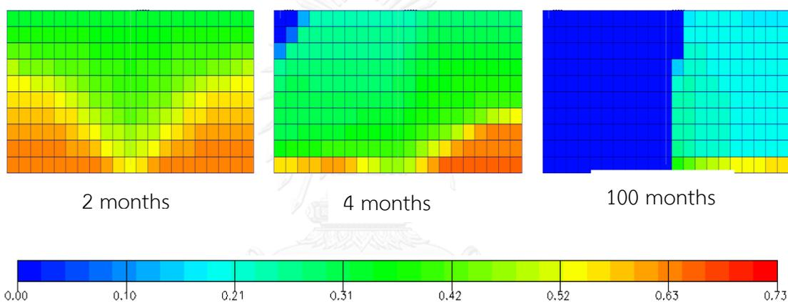
Figure A-19 Oil saturation versus time for grid plane  $i = 10$ : gas injection when  $P < 2500$  psi and vertical production well at 2000 stb/d (yz plane view)
