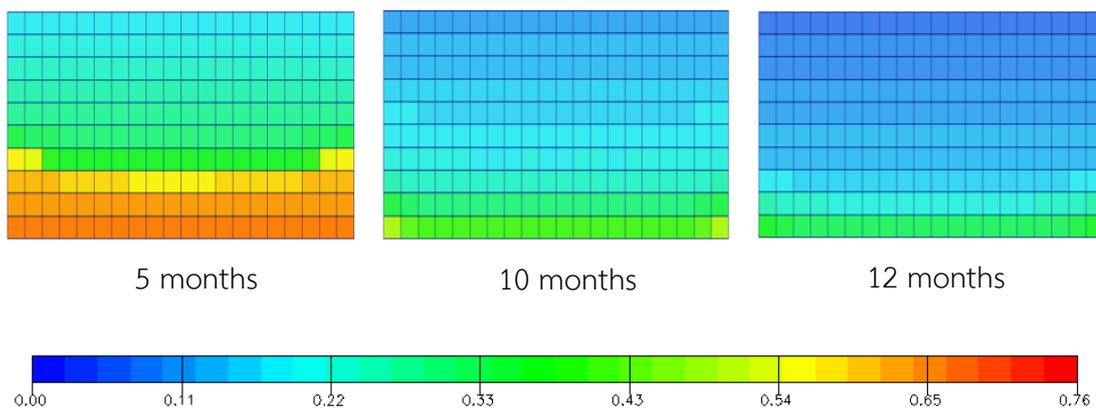
Figure A-7 Oil saturation versus time for grid plane  $j = 11$ : Horizontal production well under natural depletion at 1500 stb/d (xz plane view)
