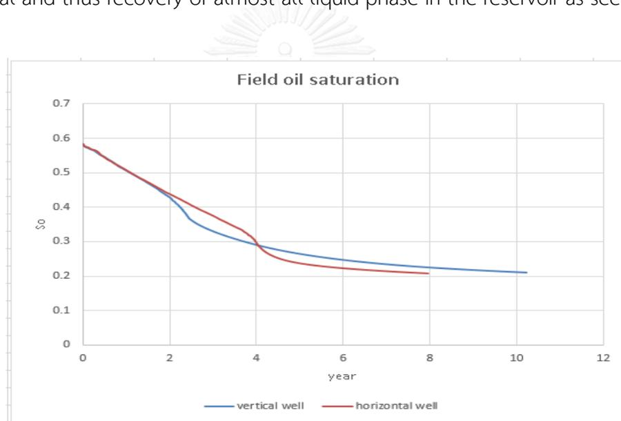
Figure 5.84 Average field oil saturation versus time for reservoir under gas injection when  $P < 1500$  psi using different well types
