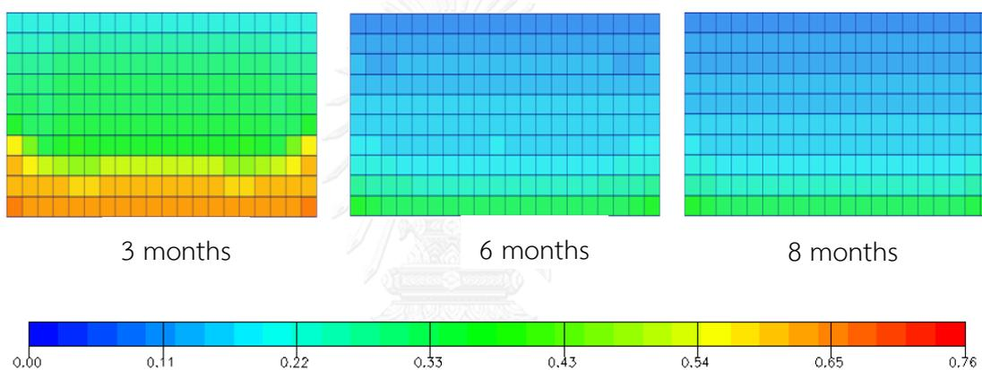
Figure A-8 Oil saturation versus time for grid plane  $j = 11$ : Horizontal production well under natural depletion at 2000 stb/d (xz plane view)
