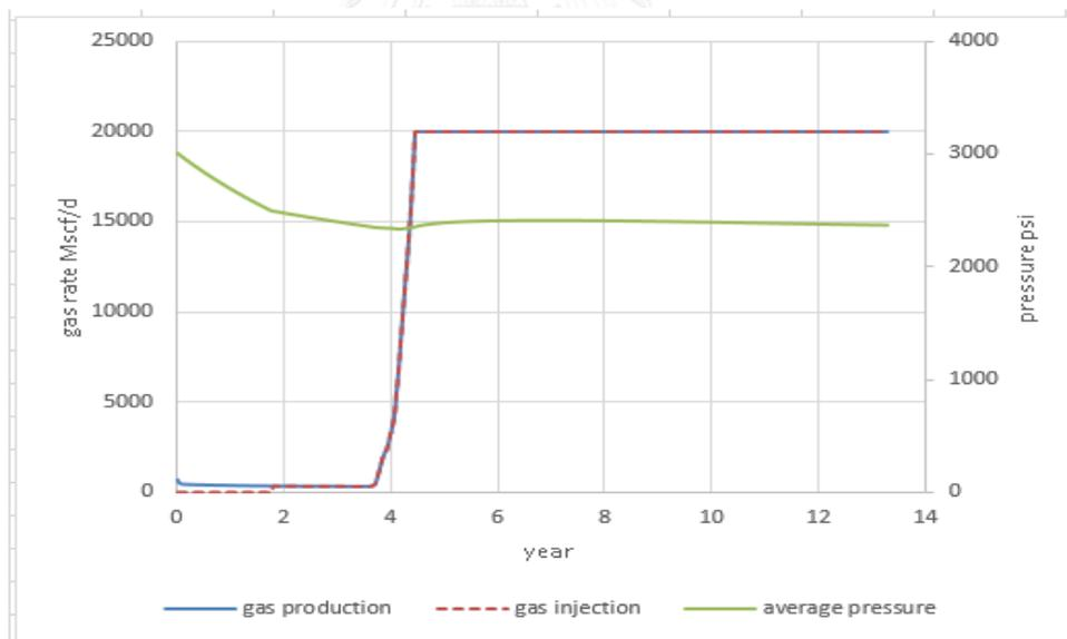
Figure 5.63 Trends of gas injection, gas production and average pressure for horizontal well producer at 500 stb/d: gas injection when  $P < 2500$  psi scenario
