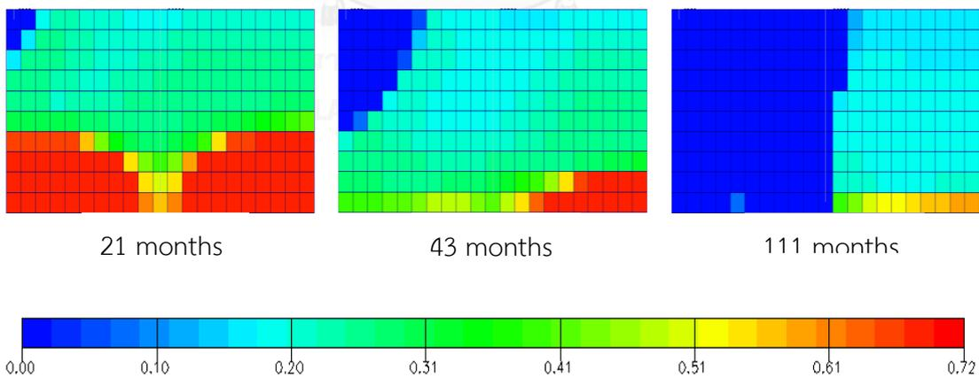
Figure A-14 Oil saturation versus time for grid plane  $i = 10$ : gas injection and vertical production well at 500 stb/d (yz plane view)
