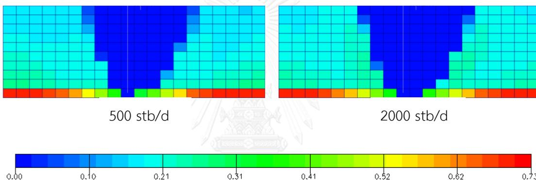
Figure A-46 Oil saturation at end of production for plane  $j = 11$ : gas injection scenario and vertical production well in position 2 for different oil rates (xz plane view)
