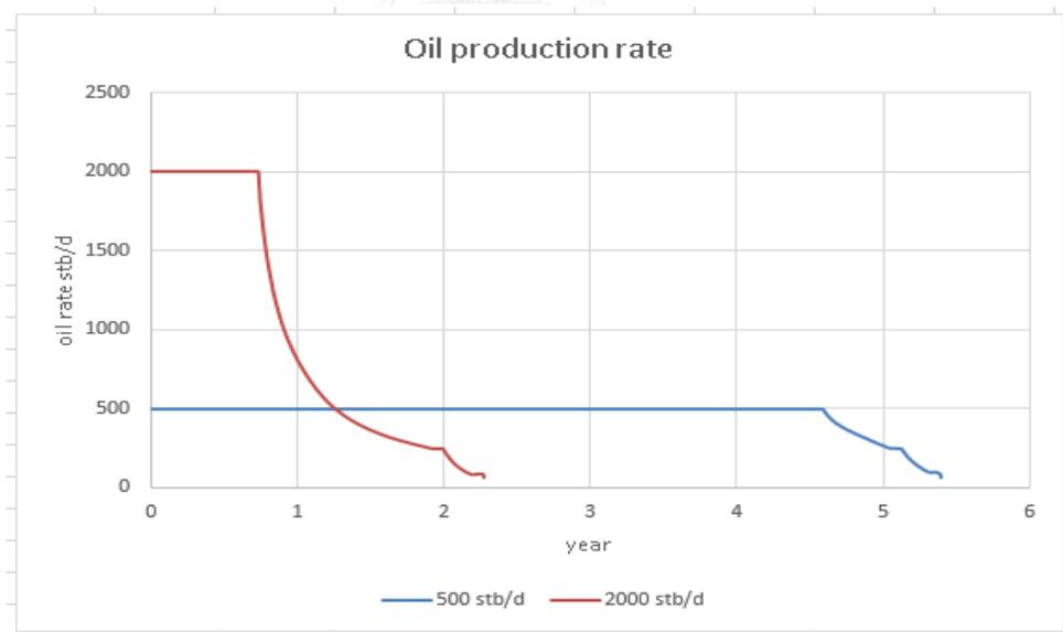
Figure 5.93 Oil production rate for horizontal wells for production constrained at GOR<80 Mscf/stb
