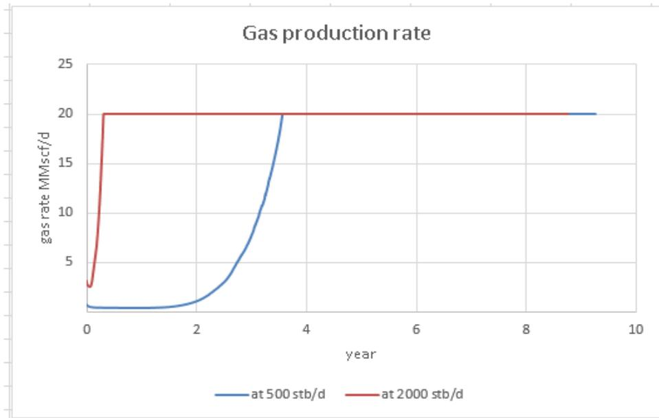
Figure 5.29 Gas production rate for vertical well under gas reinjection at different oil rates
