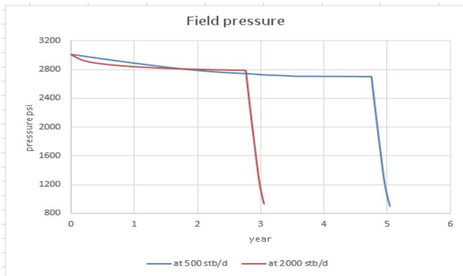
Figure 5.88 Field pressure for vertical wells: production constrained at GOR<80
