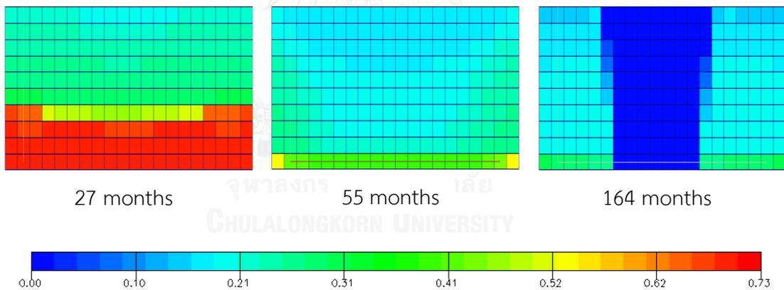
Figure 5.43 Oil saturation versus time for grid plane  $j = 11$ : gas injection with horizontal production well at 500 stb/d (xz plane view)
