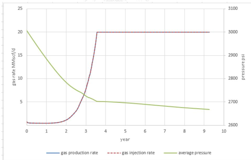
Figure 5.30 Trends of gas injection, gas production and average pressure for vertical well producer at 500 stb/d: gas injection scenario
