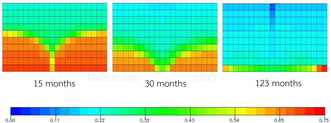
Figure 5.74 Oil saturation versus time for grid plane  $j = 11$ : gas injection when  $P < 1500$  psi with vertical production well at 500 stb/d (xz plane view)
