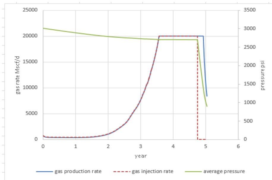
Figure 5.90 Trends of gas injection, gas production and average pressure for vertical well producer at 500 stb/d: gas injection constrained at GOR<80 Mscf/stb
