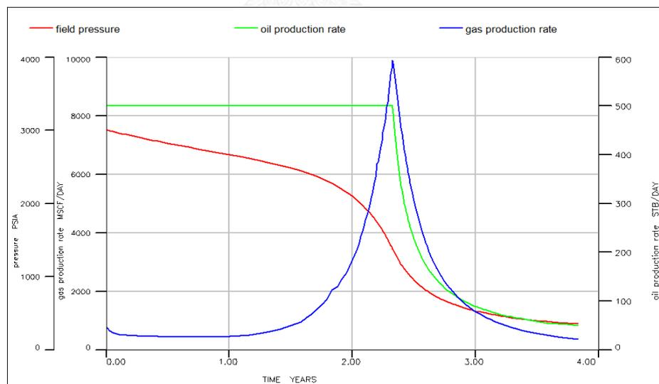
Figure 5.5 Trend of oil rate, gas rate and pressure of vertical well under natural depletion at 500 stb/d.
