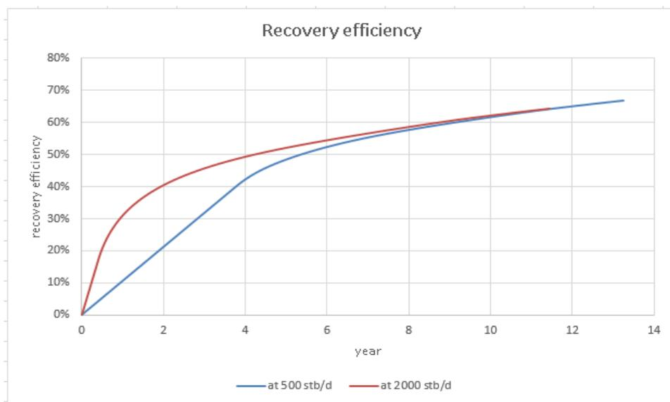
Figure 5.120 Field oil efficiency for vertical well at position 1 under produced gas reinjection
