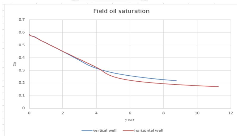
Figure 6.13 Average field oil saturation versus time for reservoir under gas injection: position 2 configuration
