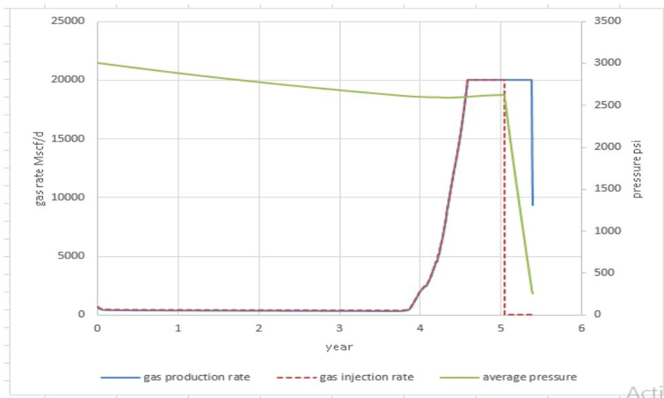
Figure 5.92 Trends of gas injection, gas production and average pressure for horizontal well producer at 500 stb/d for gas injection constrained at GOR<80 Mscf/stb
