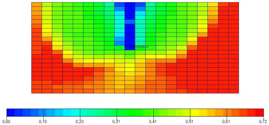
Figure 5.49 Oil saturation at abandonment for reservoir with a vertical well under gas injection at 500 stb/d (xy plane view)
