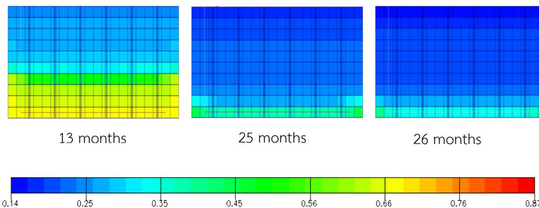
Figure A-9 Oil saturation versus time for grid plane  $j = 11$ : Fracture horizontal production well under natural depletion at 800 stb/d (xz plane view)
