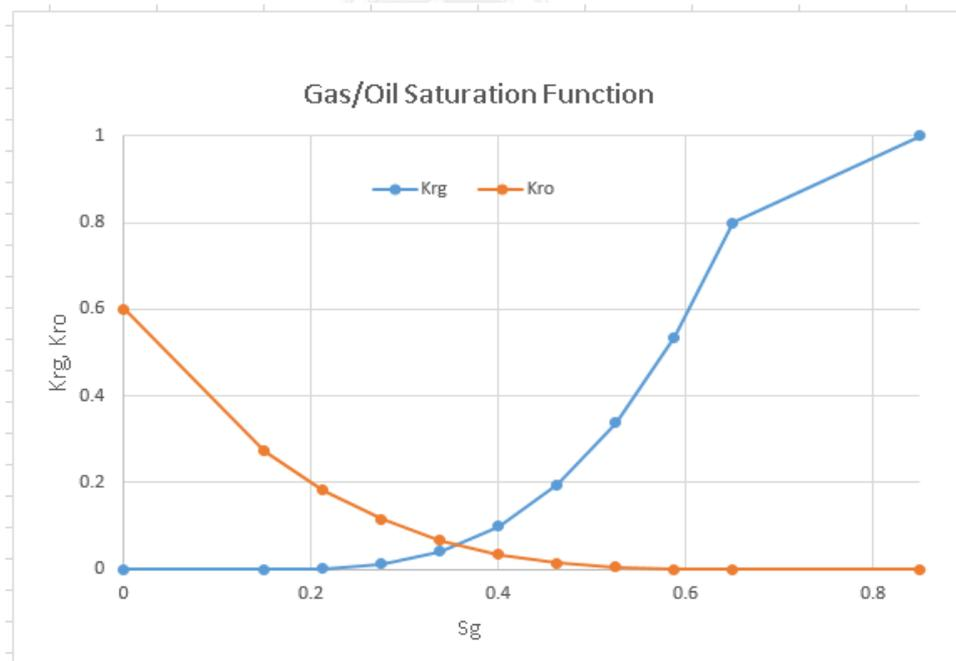
Figure 4.5 Gas/Oil Saturation function.
