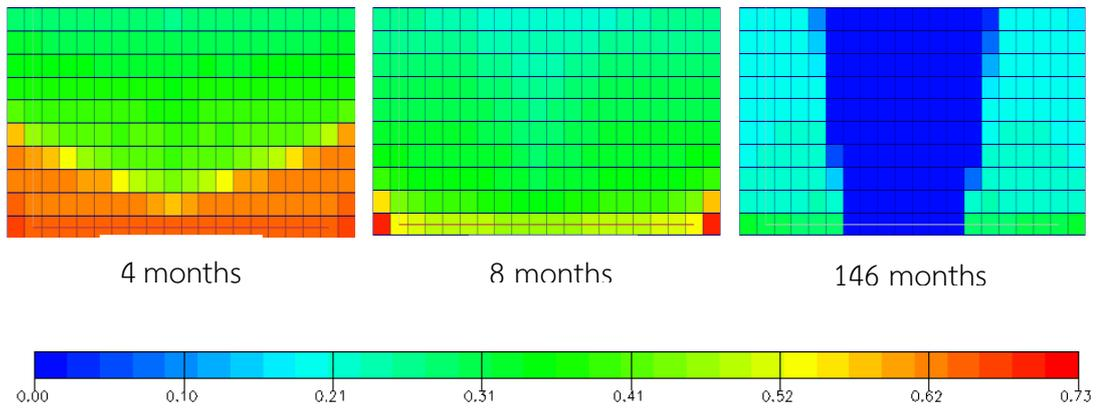
Figure 5.44 Oil saturation versus time for grid plane  $j = 11$ : gas injection with horizontal production well at 2000 stb/d (xz plane view)
