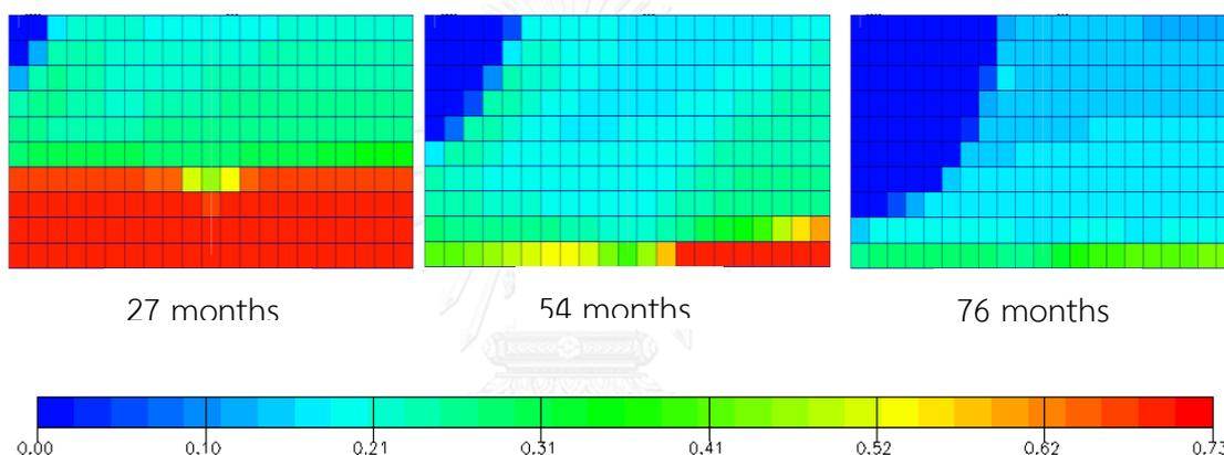
Figure A-40 Oil saturation versus time for grid plane  $i = 10$ : gas injection constrained at  $\text{GOR} < 160$  Mscf/stb and horizontal production well at 500 stb/d (yz plane view)
