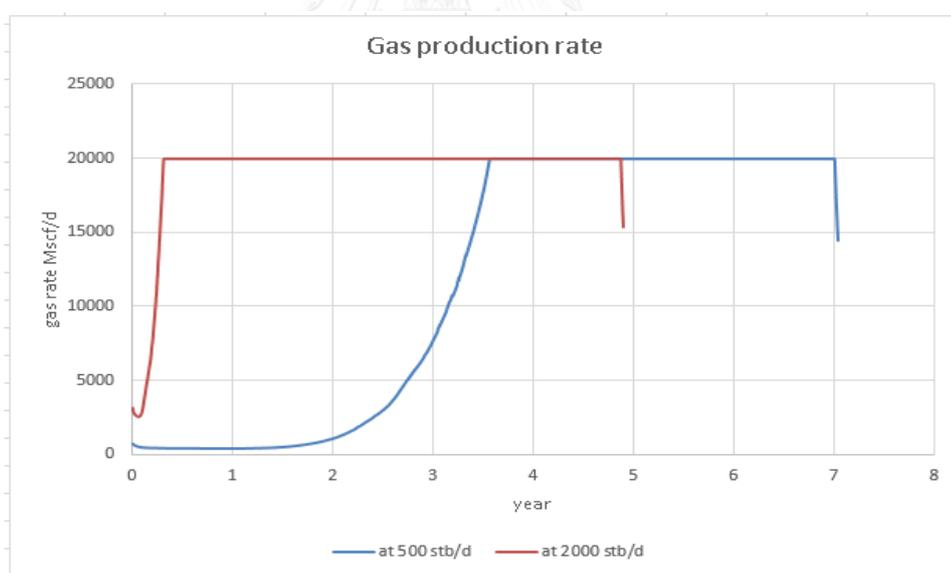
Figure 5.100 Gas production rate for vertical wells: production constrained at  $GOR < 160$  Mscf/stb
