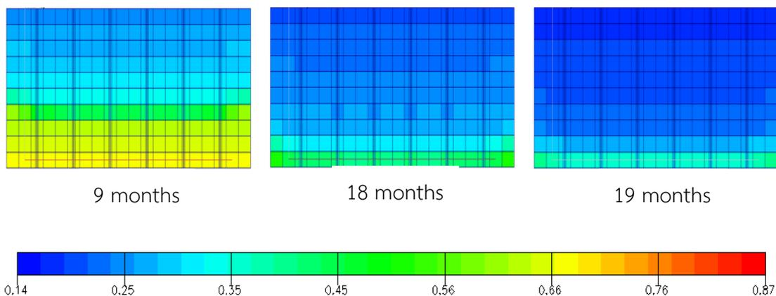
Figure A-10 Oil saturation versus time for grid plane  $j = 11$ : Fracture horizontal production well under natural depletion at 1000 stb/d (xz plane view)
