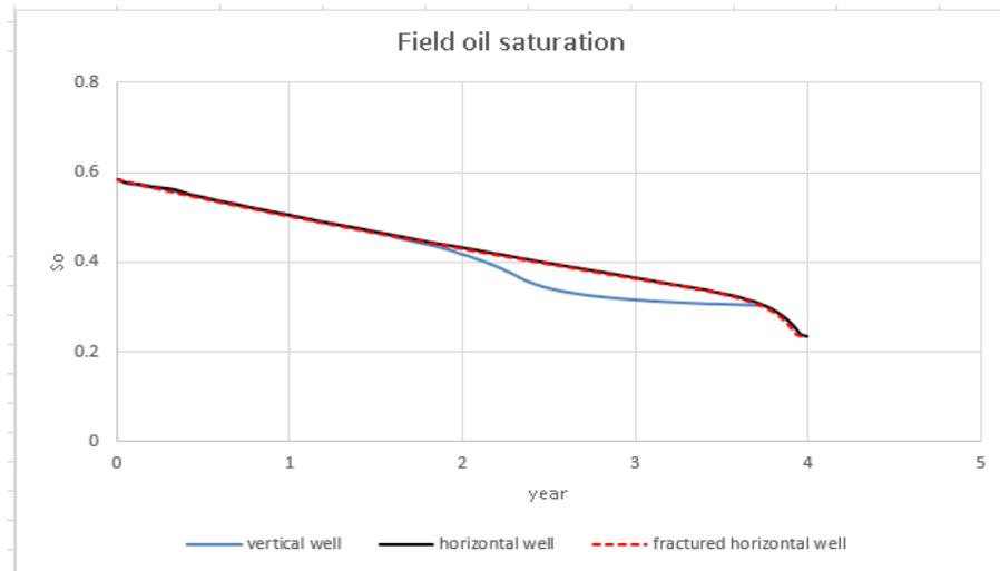
Figure 5.24 Average field oil saturation versus time for reservoir under natural depletion using different well types
