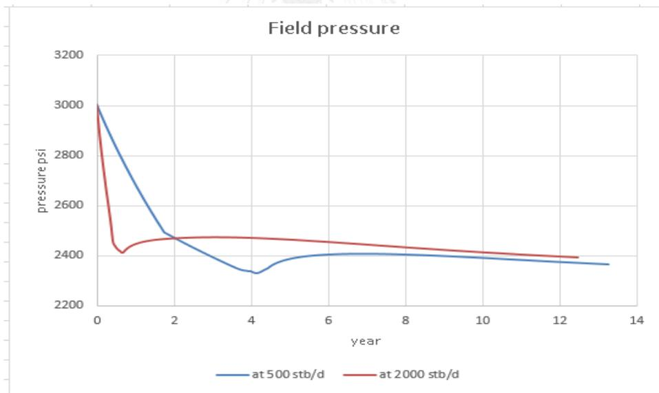
Figure 5.61 Field pressure for horizontal well under gas reinjection at pressure lower than 2500 psi
