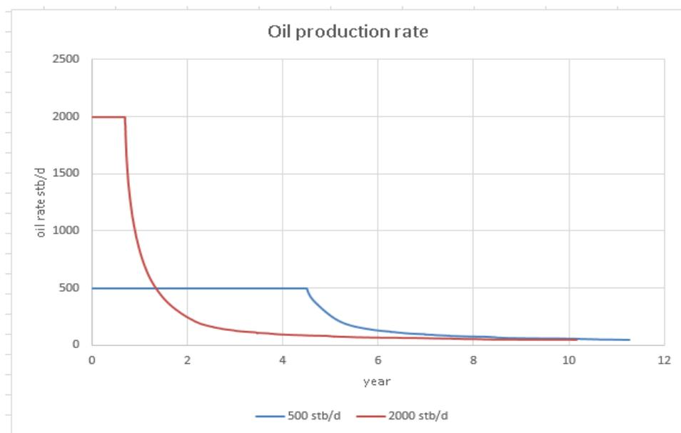
Figure 6.7 Oil production rate for horizontal well at position 2 under produced gas reinjection
