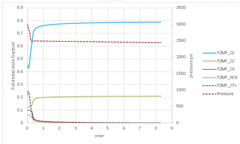
Figure B-4 Field total mole fraction and reservoir pressure vs time for the case of gas injection when pressure drops below 2500 psi using vertical well at 2000 stb/d
