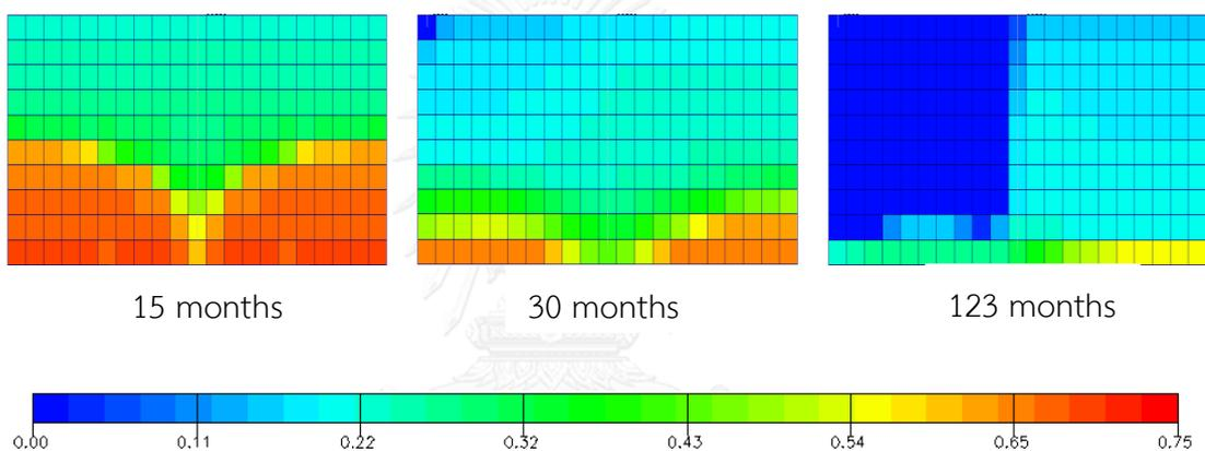
Figure A-22 Oil saturation versus time for grid plane  $i = 10$ : gas injection when  $P < 1500$  psi and vertical production well at 500 stb/d (yz plane view)
