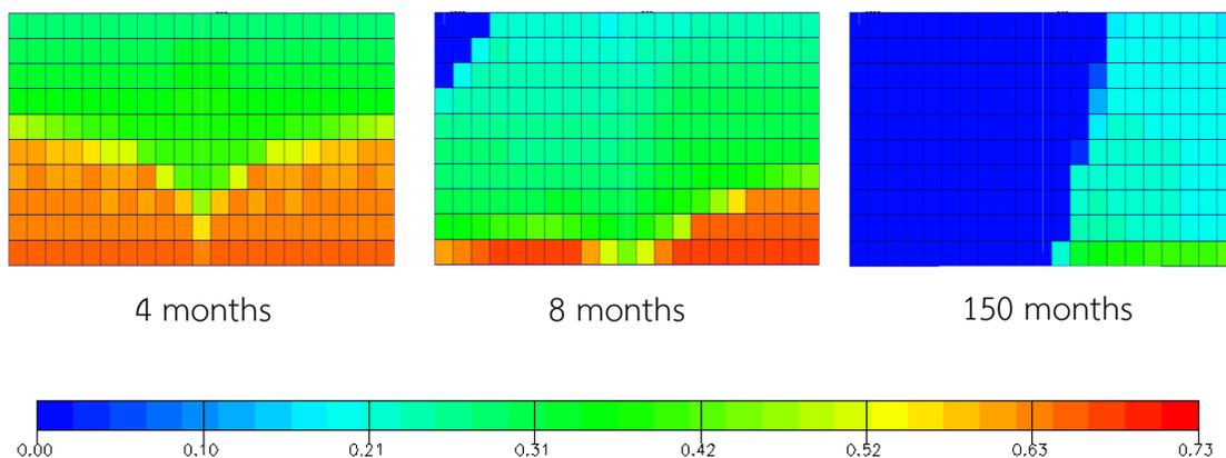
Figure A-21 Oil saturation versus time for grid plane  $i = 10$ : gas injection when  $P < 2500$  psi and horizontal production well at 2000 stb/d (yz plane view)
