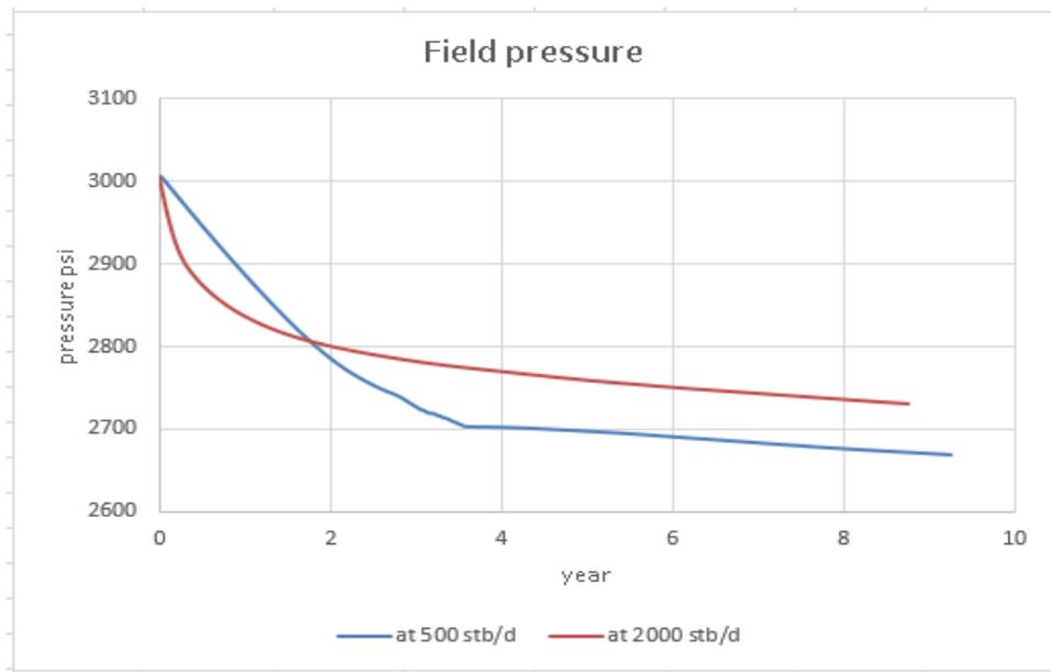
Figure 5.31 Field pressure for vertical well under gas reinjection at different oil rates
