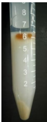
Figure 3.10. Work-up by using sat. \text{NaHCO}_3 (after centrifuge): emulsion phase of reaction at the top, aqueous phase at the middle, and precipitation at the bottom.
