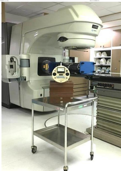
Figure 3.11 The NE2 detector at 1 m. in lateral and longitudinal direction far away from isocenter in the 23EX treatment room.
