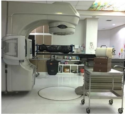
Figure 3.10 The Alderson RANDO phantom in AP head first position on the couch and the NE2 detectors at 1 m. in lateral and longitudinal far away from isocenter in the 23EX treatment room.
