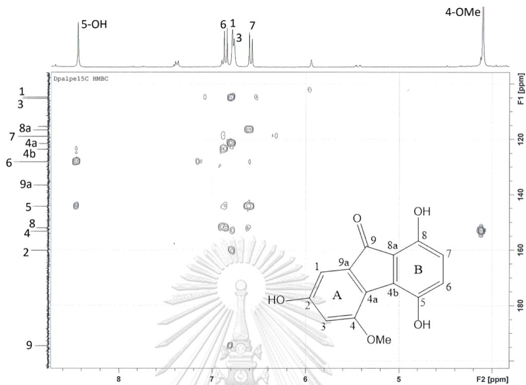
Figure 64 HMBC spectrum of compound DPB-10 (in acetone- $d_6$ )
