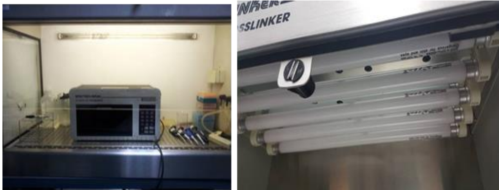
Figure 6 The UV irradiation machine (Spectrolinker™ XL-1000 UV crosslinker, USA), with UVB light at 312 nm. The exposure was performed in the laminar flow.
