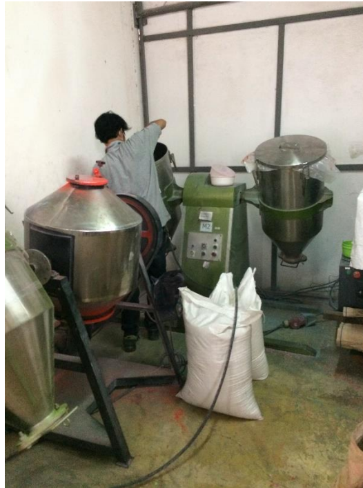
Figure 13: Color Mixing Machine
