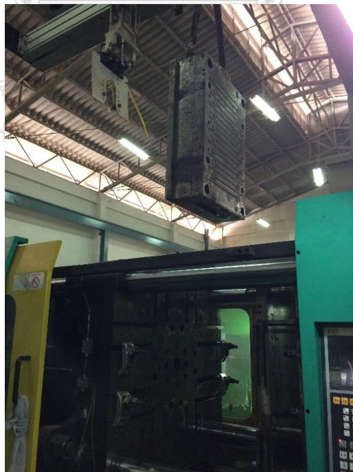
Figure 15: Mounting Mold with Crane System
