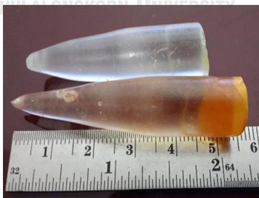
Figure 5.5 The CsI:Tl crystal ingots were grown with different CsI precursor purities of (a) 99.999% (colorless crystal) and (b) 99.9% (orange crystal).
