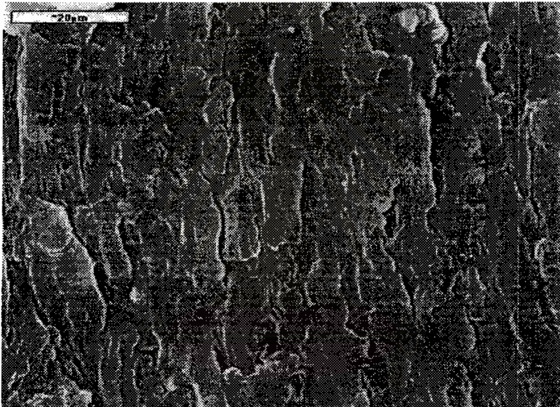
Figure 18. SEM micrograph of PP-cp/20 wt% EG/1.0 phr MAH-g-PP blends
