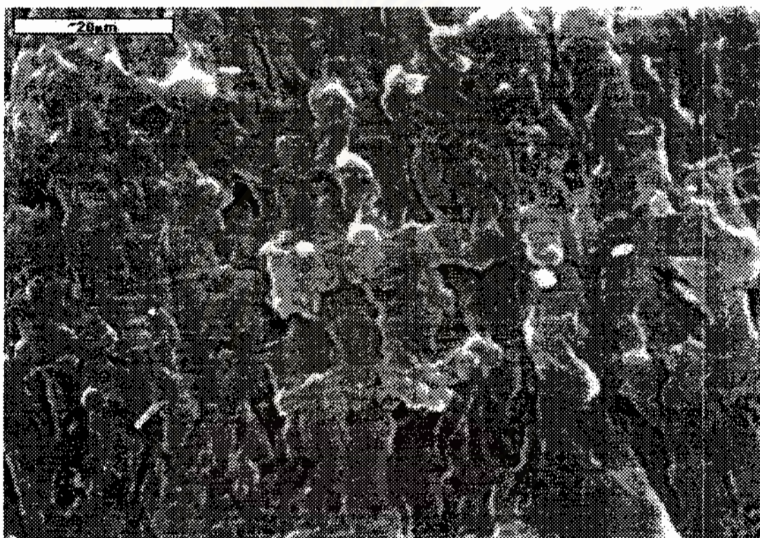
Figure 19. SEM micrograph of PP-cp/20 wt% EG/2.0 phr MAH-g-PP blends
