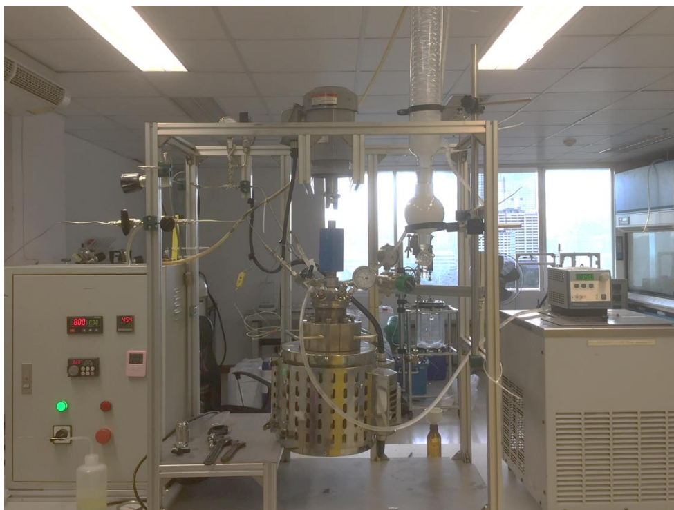
Figure 7 Illustration of pyrolysis semi-batch reactor instruments and control device
