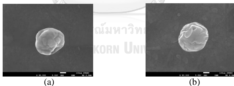
Figure 31 The SEM results of MPE-SLNs, (a) MPE-PA-SLNs, (b) MPE-SA-SLNs
