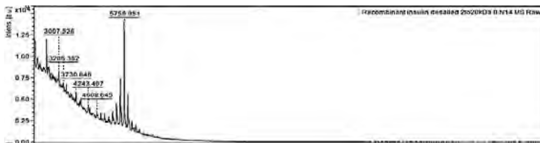
Figure 2.10: Typical MALDI-TOF mass spectra of supernatant of culture sample from P. pastoris KM71H (TP1). The highest peak was expected to be MIP ( m/z 5756.951)
