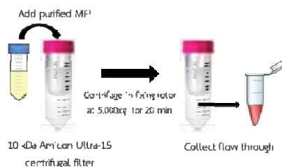
Figure 2.7: Purification of MIP by 10 kDa Amicon Ultra-15 Centrifugal Filter
