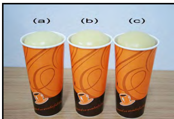
Figure 4.15 RPUR foams catalyzed by \text{Cu}(\text{OAc})_2(\text{en})_2:\text{Zn}(\text{OAc})_2(\text{en})_2 at different NCO indexes (a) 100; (b) 150; (c) 200
