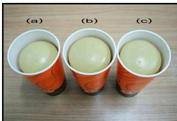
Figure 4.16 RPUR foams catalyzed by \text{Cu}(\text{OAc})_2(\text{en})_2:\text{Ni}(\text{OAc})_2(\text{en})_2 at different NCO indexes (a) 100; (b) 150; (c) 200
