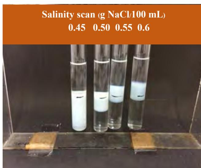
**Figure A6** Phase behavior of 6:4 by molar ratio of sodium dioctyl sulfosuccinate ,AOT, and internal olefins sulfonate ,IOS C<sub>19-23</sub>, using heptane as an oil phase.
