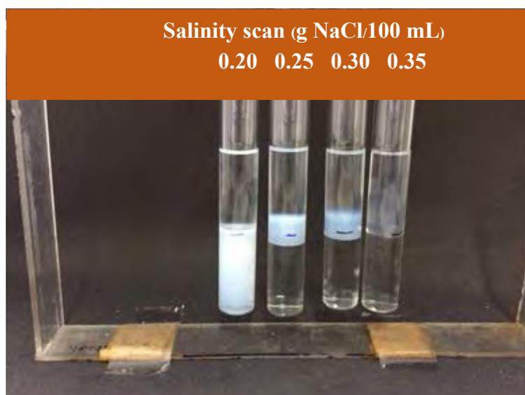
**Figure A17** Phase behavior of 9:1 by molar ratio of sodium dioctyl sulfosuccinate ,AOT, and internal olefins sulfonate ,IOS C<sub>19-23</sub>, using decane as an oil phase.
