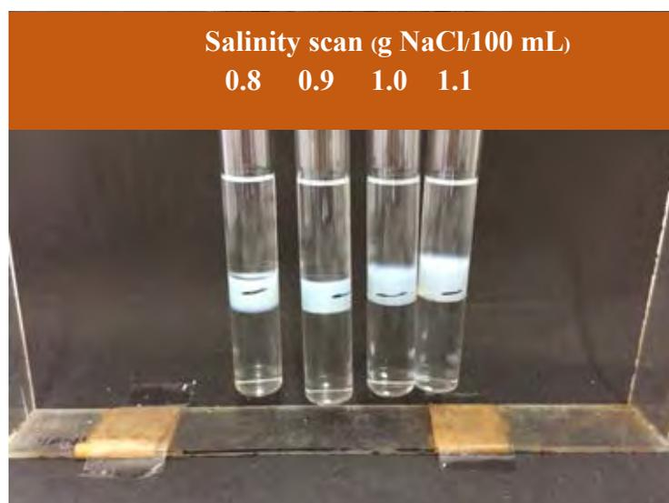
**Figure A14** Phase behavior of 6:4 by molar ratio of sodium dioctyl sulfosuccinate, AOT, and internal olefins sulfonate, IOS C<sub>19-23</sub>, using decane as an oil phase.
