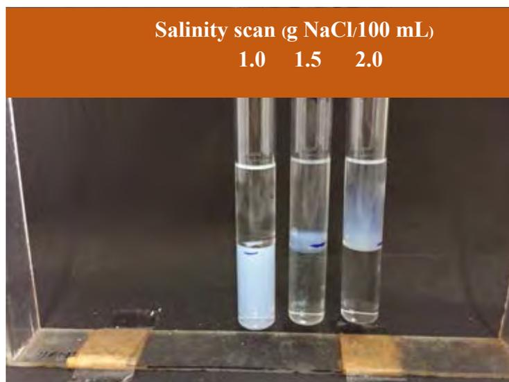
**Figure A9** Phase behavior of 6:4 by molar ratio of sodium dioctyl sulfosuccinate ,AOT, and internal olefins sulfonate ,IOS C<sub>15-18</sub>, using decane as an oil phase.
