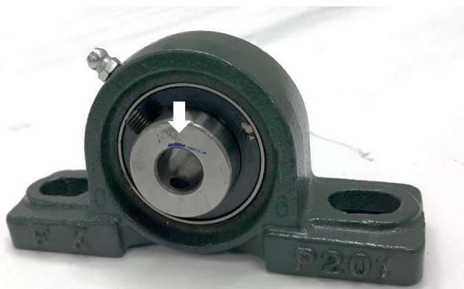
Figure 16 Bearing with set screws (white arrow) to lock with the axle shaft flat.
