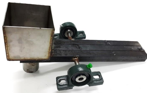
Figure 22 Both sides of the pivot axle were connected to both bearings
