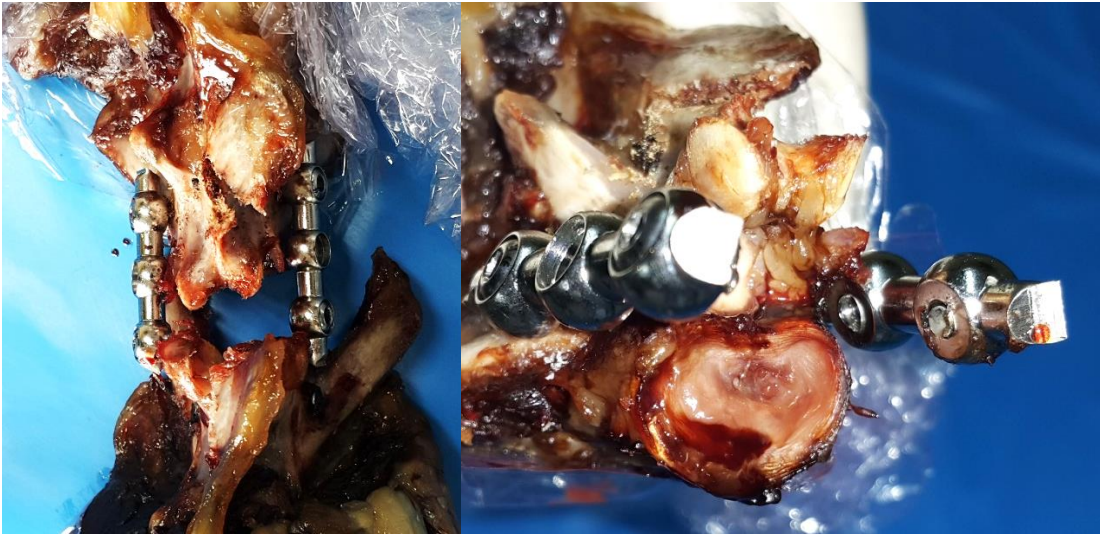
Figure 40 In the SOP group, construction failure occurred through the screw neck of both sides of the construction.
