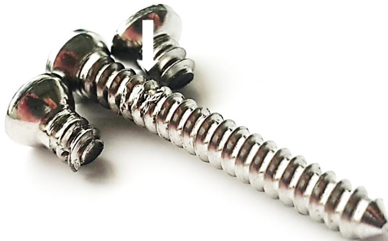
Figure 41 In the SOP group, crack formation fissure around the screw neck (white arrow) and broken screws.
