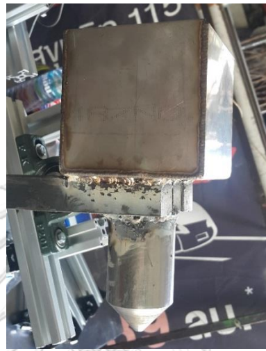
Figure 21 Welding all iron bars, conical wedge and loading unit together
