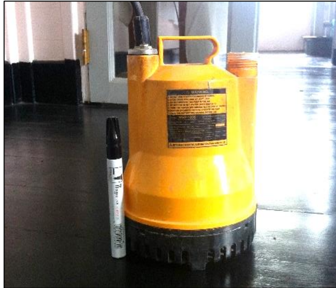
Figure 2.4 Submersible Pump for pumping test.
