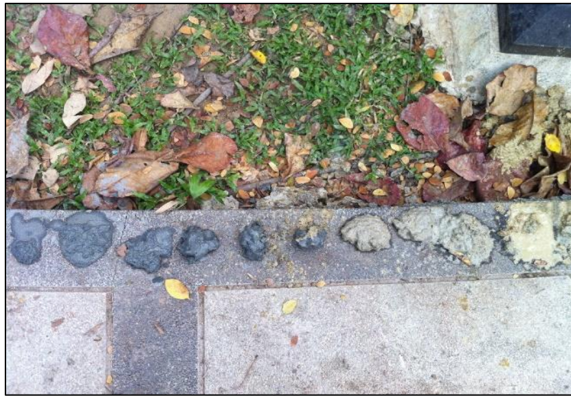
Figure 2.16 Samples of from well no.1 that's collected every 1 meter-depth.
