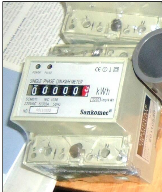
Figure 2.10 Electricity meter for measuring electricity consumption.
