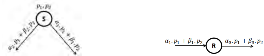
(a) Source encodes p_1, p_2 to product two encoded packets (b) Relay node catches a encoded packets and re-encodes it. by creating two independent linear equations for two transmission paths.
