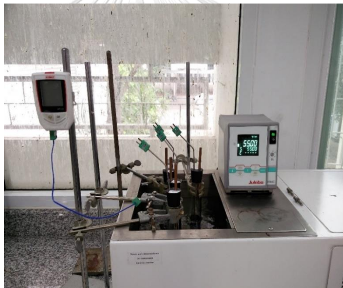
Figure 3-7: Equipment set up for wax deposition
