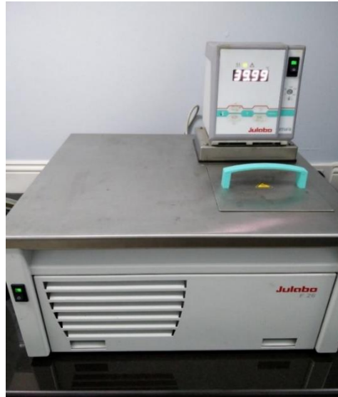
Figure 3-3: Julabo Glycol solution bath
