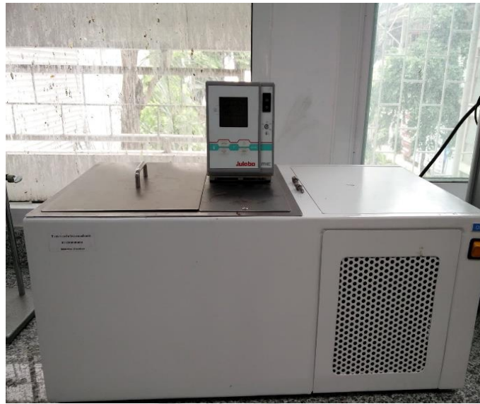
Figure 3-6: Julabo immersion circulator
