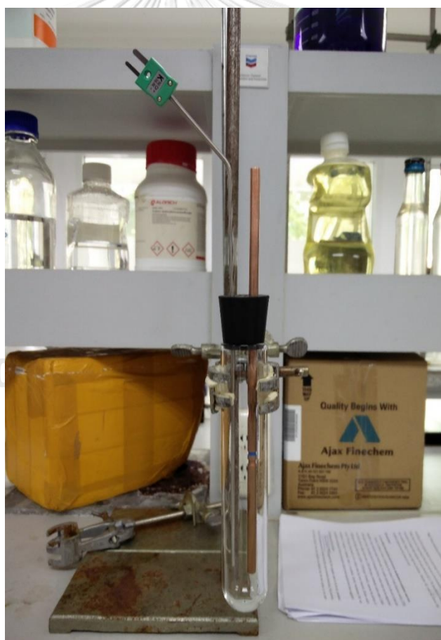
Figure 3-5: Rod finger for wax deposition test
