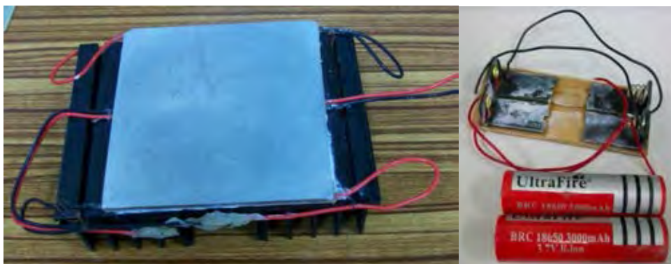
Figure 4.12 The TEG module set and Li-ion battery with 3,000 mAh capacity
