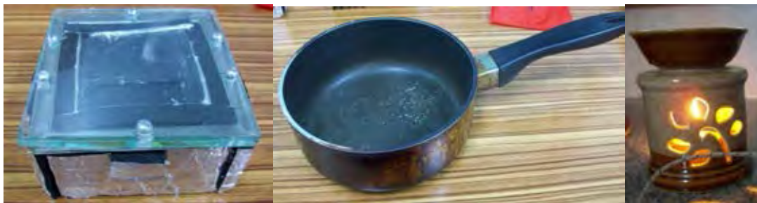
Figure 4.14 Various equipments for heat power input using in the research: (left) a solar-thermal power trap or “green house” module prototype; (middle) a cooking device heated from LPG burner; and (right) candle flame
