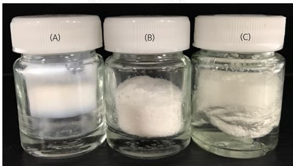
Figure 8 Physical appearance of water-entrapped silica particles containing 5% of R812S prepared with different methods: (A) Low shear mixer and adding water all at once, (B) High shear mixer and adding water all at once, and (C) High shear mixer with water atomization.
