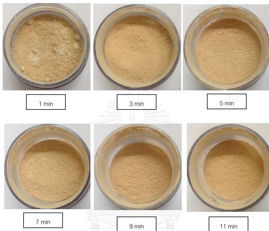
Figure 23 Physical appearance of loose face powder containing water-entrapped silica particles prepared with multiple step of different mixing time.
