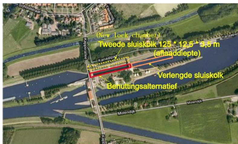
Figure 2.4 Dimensions of new chamber (RWS, 2010)
