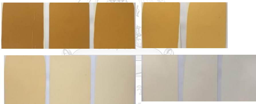
Figure B10 Spectrum reflectance (%) and calibrated color swatches of Yellow Oxide at different concentrations. From left to right; 99.99, 75.00, 50.00, 25.00, 12.50 (top), 5.00, 2.50, 1.25, 0.625, 0.315, and 0.156 (bottom).
