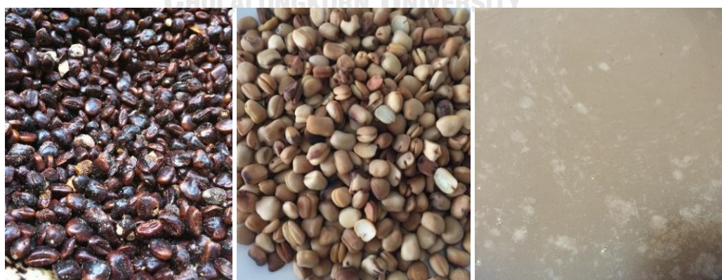
Figure 3.2 Tamarind seeds before roasting (left), light brown seeds before boiling and (middle) Tamarind Glue (right).
