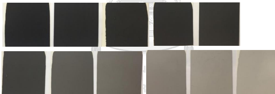
Figure B16 Spectrum reflectance (%) and calibrated color swatches of Black at different concentrations. From left to right; 99.99, 75.00, 50.00, 25.00, 12.50 (top), 5.00, 2.50, 1.25, 0.635, 0.315, and 0.156 (bottom).
