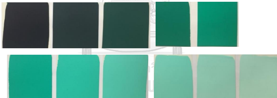
Figure B7 Spectrum reflectance (%) and calibrated color swatches of green at different concentrations. From left to right; 99.99, 75.00, 50.00, 25.00, 12.50 (top), 5.00, 2.50, 1.25, 0.635, 0.315, and 0.156 (bottom).
