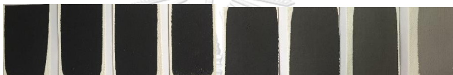
Figure B6 Spectrum reflectance (%) and calibrated color swatches at different concentrations of Black. % concentration from left to right; 99.99, 75, 50, and 25, 12.50, 5.00, 2.50, and 1.25, respectively Measurement performed in five places with X-Rite SP62, illuminant /observers: D65/2, SPEX.
