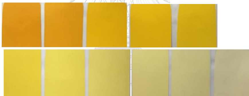
Figure B9 Spectrum reflectance (%) and calibrated color swatches of Yellow WF at different concentrations. From left to right; 99.99, 75.00, 50.00, 25.00, 12.50 (top), 5.00, 2.50, 1.25, 0.635, 0.315, and 0.156 (bottom).
