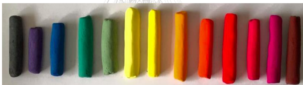
Figure 5.3 Sticks of pastel primary color (from left to right): Carbon Black, Violet RLS-EF, Blue-BX, Green GNX, Chrome Green, Oxide Yellow –BV02, Yellow F2G, Yellow M2R 70, Orange GR, Red D3G 70 Permanent Rubine Red, Pink EM25, and Brown HFR01.
