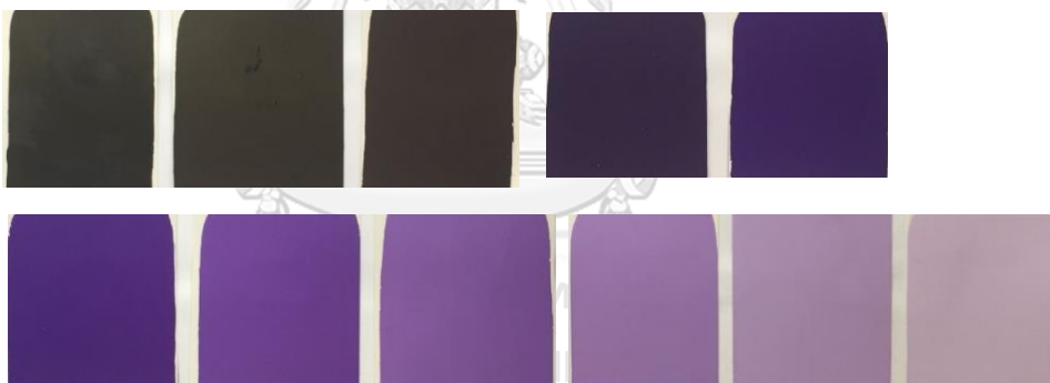
Figure B15 Spectrum reflectance (%) and calibrated color swatches of Violet at different concentrations. From left to right; 99.99, 75.00, 50.00, 25.00, 12.50 (top), 5.00, 2.50, 1.25, 0.635, 0.315, and 0.156 (bottom).
