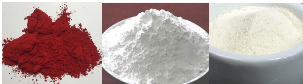
Figure 3.6 Hostoperm Permanent Rubine L4B (left), \text{CaCO}_3 (middle), and gum tragacanth powder (right).
