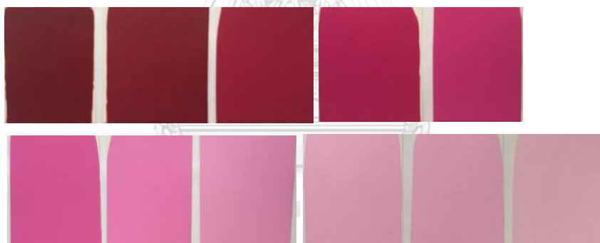
Figure B14 Spectrum reflectance (%) and calibrated color swatches of Pink E at different concentrations. From left to right; 99.99, 75.00, 50.00, 25.00, 12.50 (top), 5.00, 2.50, 1.25, 0.635, 0.315, and 0.156 (bottom).
