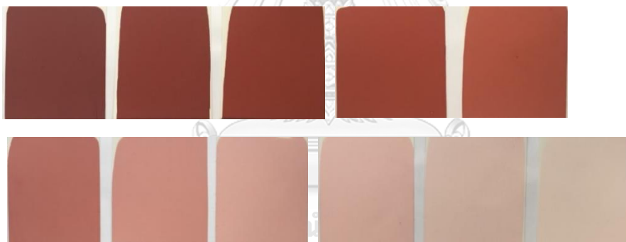
Figure B12 Spectrum reflectance (%) and calibrated color swatches of oxide red at different concentrations. From left to right; 99.99, 75.00, 50.00, 25.00, 12.50 (top), 5.00, 2.50, 1.25, 0.635, 0.315, and 0.156 (bottom).
