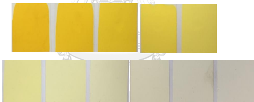
Figure B8 Spectrum reflectance (%) and calibrated color swatches of Yellow H3G at different concentrations. From left to right; 99.99, 75.00, 50.00, 25.00, 12.50 (top), 5.00, 2.50, 1.25, 0.625, 0.315, and 0.156 (bottom).
