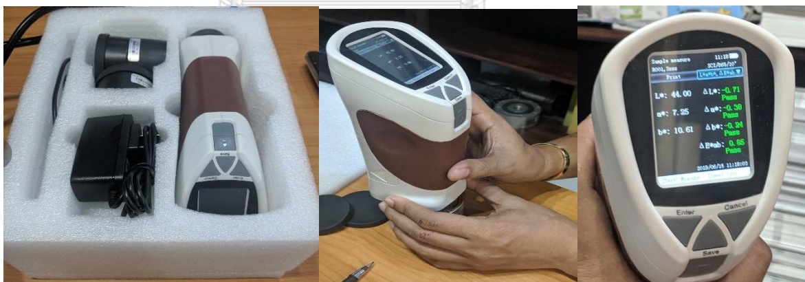
Figure 46 Figure CS-100 colourimeter measurement
