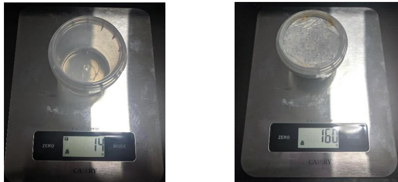
Figure 45 PP with safety lock Packaging weight is 14 and Gross is 160g
