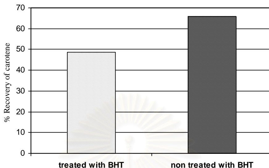
Figure 4.17 Effect of antioxidant on % recovery of carotene at 60 °C, 60 minutes, ratio of clay to palm oil = 1:5 and THF was used as eluting solvent.
