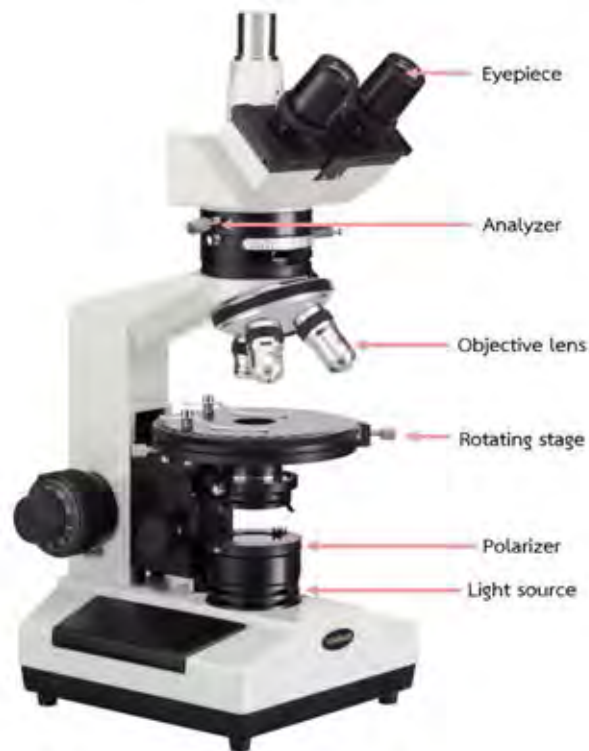
Figure 3.5 The basic component of polarized light microscope (modified from Amscope)
