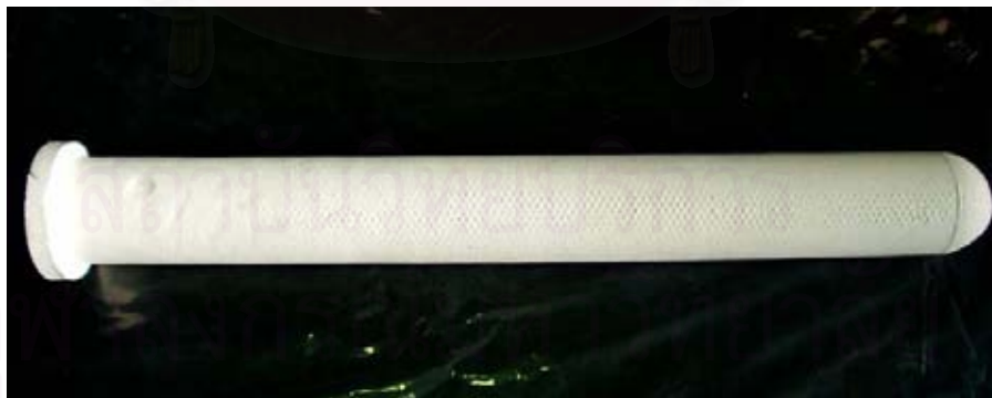
Fig. 4.2 Photo of ceramic candle filter using in experimental set-up
