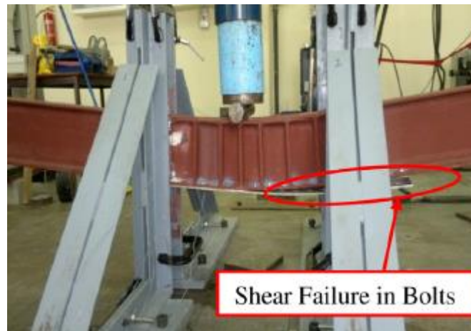
Figure 1.2 Plate end debonding failure of strengthened steel beam with anchoring bolts. [2]
