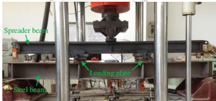
Figure 2.16 FRP-strengthened steel beam with a stiffener. [38]
