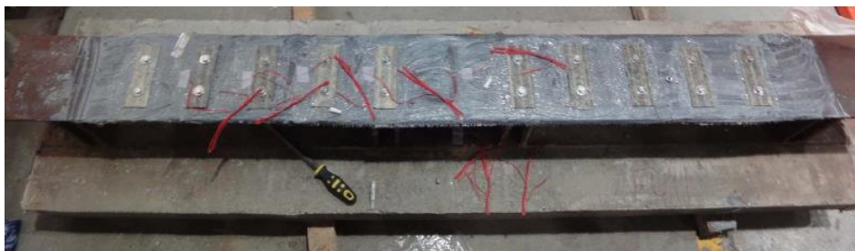
Figure 2.22 Anchorage system of the beam tested by Karam et al. [49]
