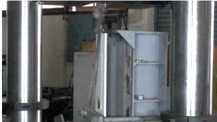
Figure 4.1 Visible failure of joints without initial bond defect (joint JMU400-0).
