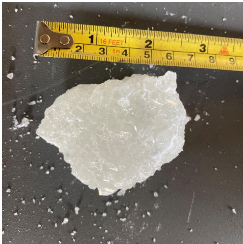
Figure 60: Biggest diameter of chopped rock sugar from machine
