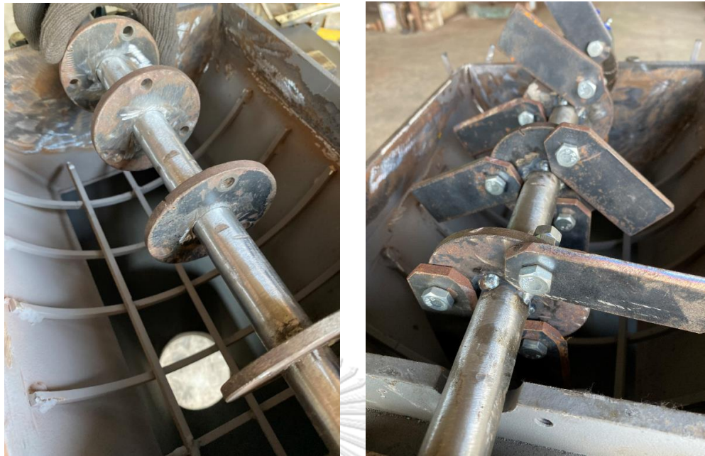
Figure 41: Assembly of hammer and shaft
