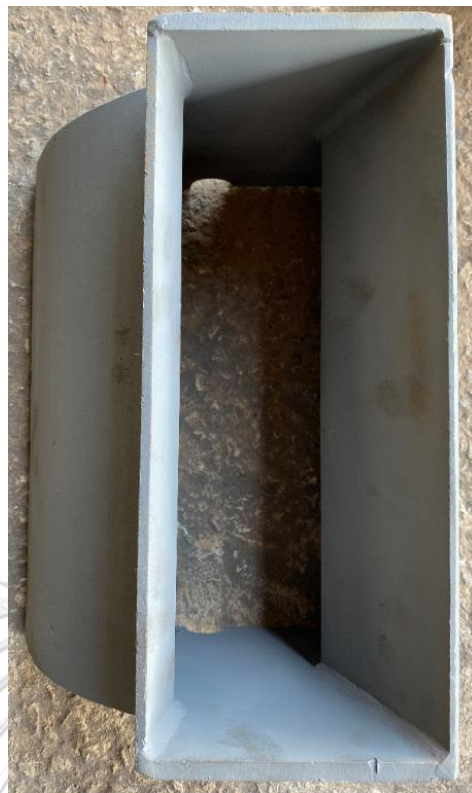
Figure 43: Hopper of rock sugar chopping machine
