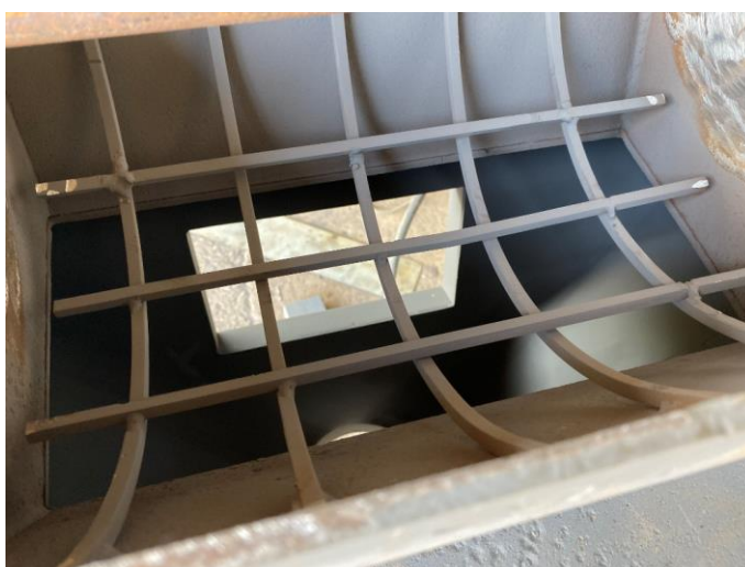
Figure 40 : Sieve in rock sugar chopping machine
