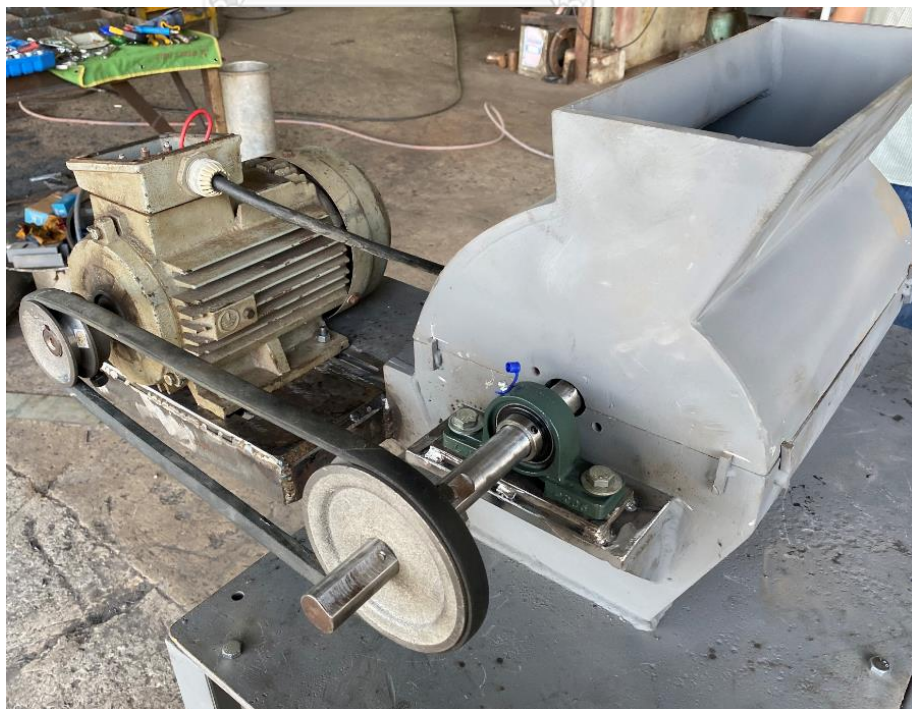
Figure 48: Chopping machine with belt (2)
