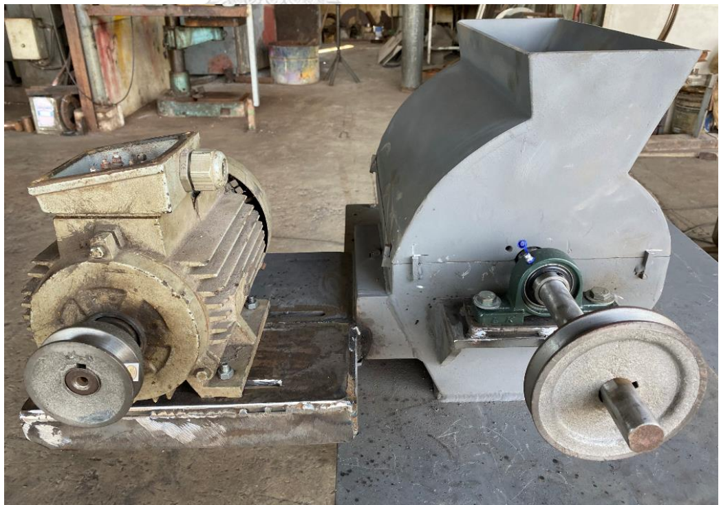
Figure 46: Chopping machine and electric motor
