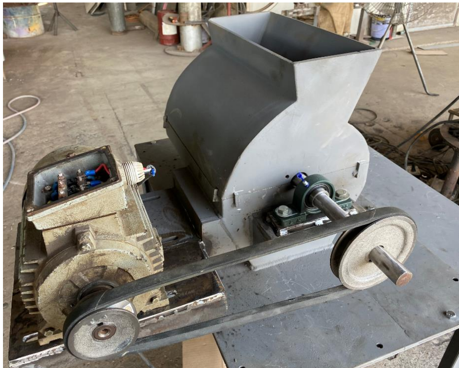
Figure 47: Chopping machine with belt
