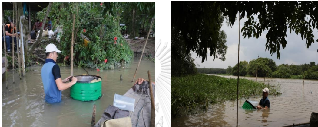
Figure B. 3: Field measure seepage of riverbed along Saigon river
