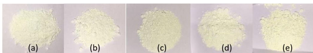
Figure 24 The appearance of fresh catalysts with different phase of \text{TiO}_2 (a) \text{WO}_3/\text{TiO}_2\text{-R0} (b) \text{WO}_3/\text{TiO}_2\text{-R25} (c) \text{WO}_3/\text{TiO}_2\text{-R50} (d) \text{WO}_3/\text{TiO}_2\text{-R75} (e) \text{WO}_3/\text{TiO}_2\text{-R100}
