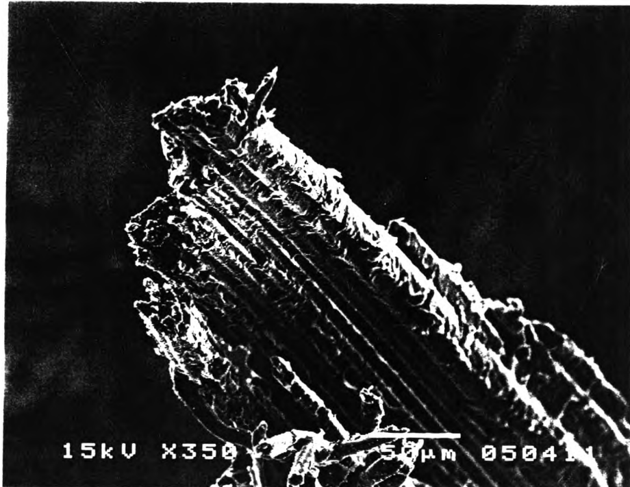
Figure 5.24 SEM micrograph of the fiber-bundle surface after using silane coupling agent ( X 350 )
