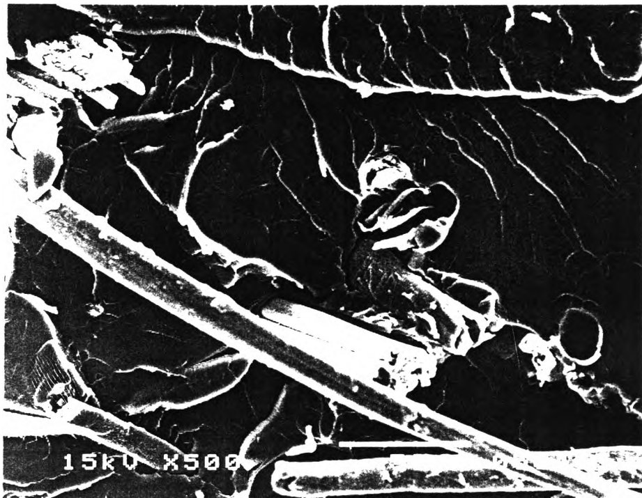
Figure 5.34 SEM micrograph of the cracking surface after 24-hour NaOH treatment. ( X 500 )
