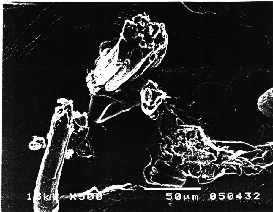
Figure 5.33 SEM micrograph of the cracking surface after 18-hour NaOH treatment. ( X 500 )
