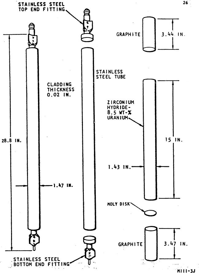
TRIGA stainless-steel-clad fuel element with triflute Fig. 3.3 end fittings. Graphite top and bottom reflector heights of 3.45 in. were used in the calculations. (Figure was reproduced from Ref. 10).
