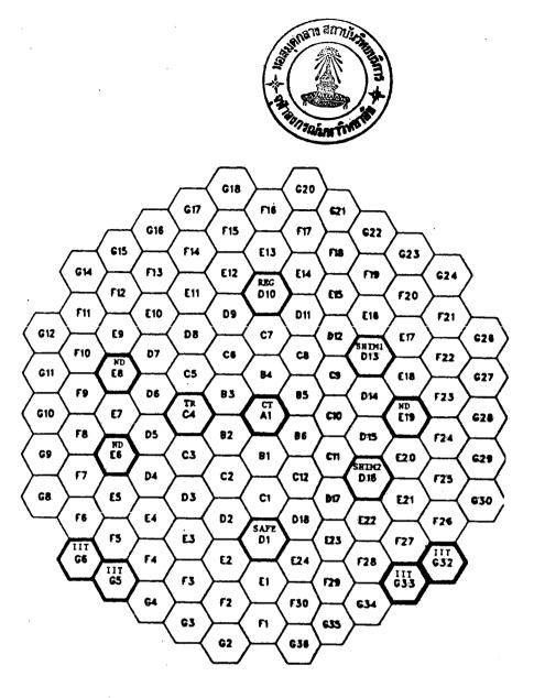
Fig. 3.1 Horizontal Cross Sections of TRR-1/M1 Reactor Core Computer Model
