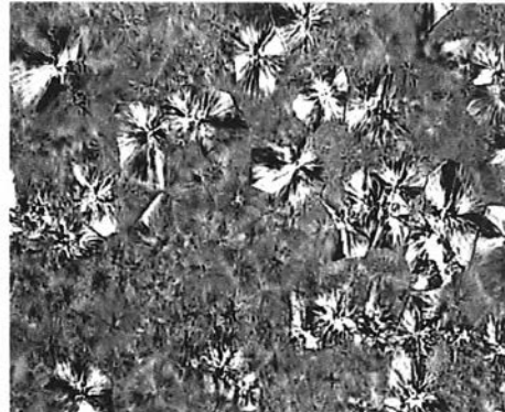
(A) Spherulite of PP
