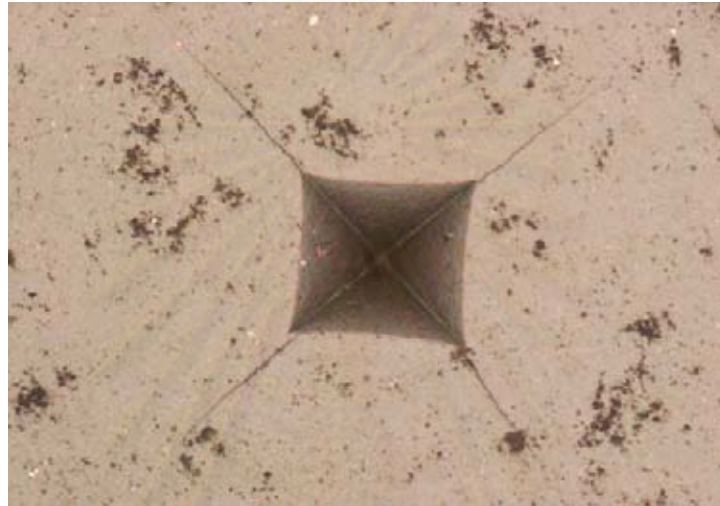
Fig 4.19 Top view of indent of E8H specimen sintered in air furnace at 1700 °C for 2 h
