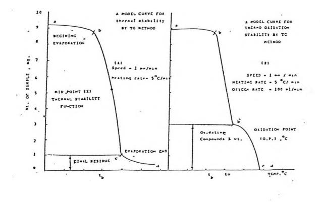
Figure 2.2 Comparison between typical model curves for both TG thermal and thermooxidation stabilities.
