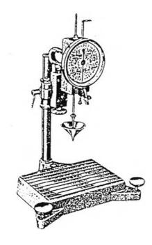
Figure 2.1 The penetrometer
