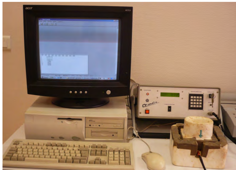
Figure 5.1 Computer connected CT meter (SA TELEPH, Meylan, France) for measurement of thermal conductivity and specific heat of ground malt.
