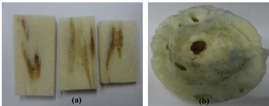
Figure 4.16 The defects of RPUR foam resulted from using \text{Cu}(\text{OAc})_2(\text{en})_2 15%wt in ethylene glycol as a catalyst (a) burning area in the foam and (b) large holes in the foam at the bottom of the mold
